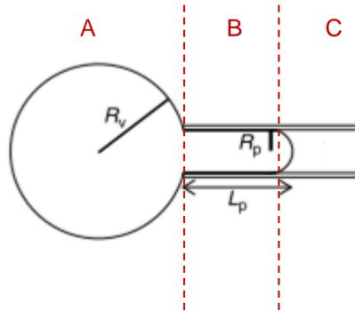
**Figure 39 – Geometry of a micropipette-aspirated vesicle**
