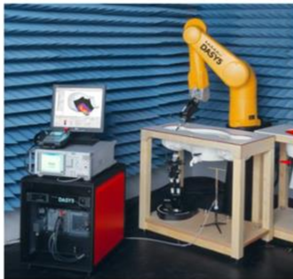
Figure 17 SAR measurement system for mobile phone that involves an E-field probe positioned by a robot in a head phantom exposed to a mobile phone at the right ear.
