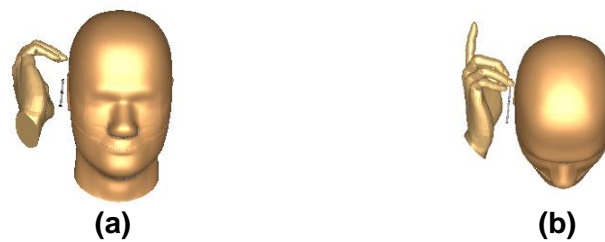
Figure 23 Half-wave dipole antenna in the vicinity of human head and hand: Perspective view (a), Top view (b).
