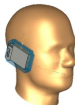
Figure 102 Perspective view of the geometrical structure of the proposed dual band PIFA antenna in the vicinity of human head.
