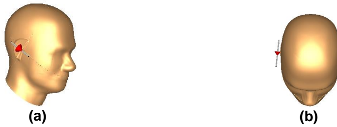
Figure 19 Half-wave dipole antenna in the vicinity of human head: Perspective view (a), Top view (b).
