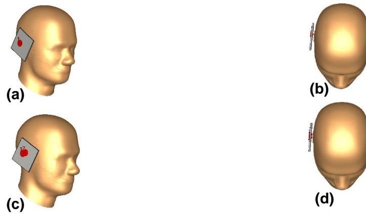
Figure 32 Patch antenna and circular polarized patch antenna in the vicinity of human head: Perspective view (a) and (c), Top view (b) and (d).
