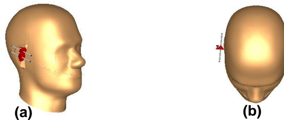
Figure 27 Array of two half-wave dipole antenna in the vicinity of human head: Perspective view (a), Top view (b).
