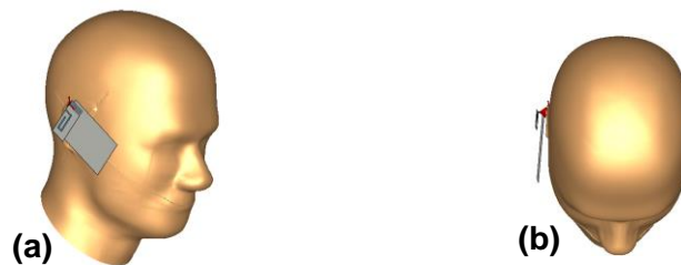
Figure 66 Geometrical structure of the dual band PIFA antenna in the vicinity of human head: Perspective view (a), and Top view (b).
