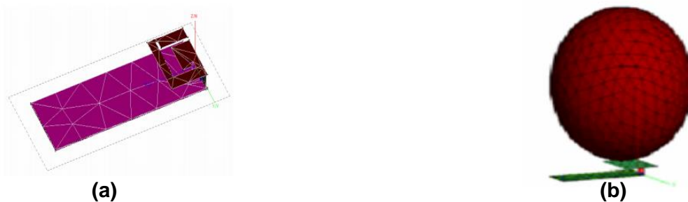
Figure 6 Slotted PIF antenna: without RF shield (a), and with RF shield in the presence of human head (b).
