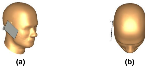
Figure 45 PIFA antenna in the vicinity of human head: (a) Perspective view, (b) Top view.
