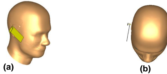
Figure 82 Geometrical structure of Tri band PIFA antenna in the vicinity of human head with U-edges: Perspective view (a), and Bottom view (b).
