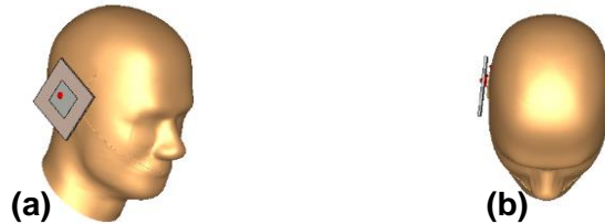
Figure 36 Patch antenna in the vicinity of human head: (a) Perspective view, (b) Top view.
