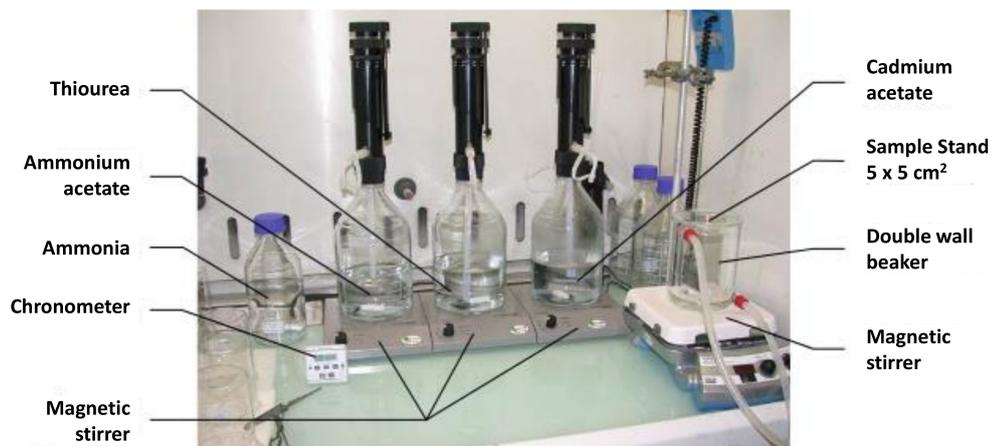
Figure 3.5: Equipment used for chemical bath deposition of CdS buffer layer.
