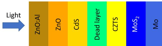
**Figure 5.21:** Schematic of thin film layers used for the EQE calculation with a dead layer to consider as front interface recombination.
