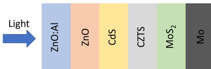
**Figure 3.18:** Schematic of the thin film layers used for the EQE construction modeling.
