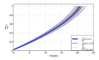
Figure IV.8 – Predicted deterioration  $\hat{D}$  for prognostic of RUL. The figure shows 300 possible trajectories of  $\overline{\hat{D}}$  within the intervals given by the observer at the time  $t_c$ .
