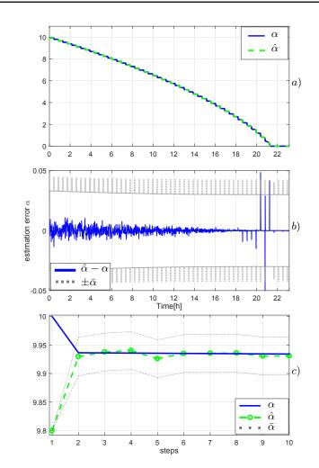
Figure IV.5 – Estimation of  $\hat{\alpha}$ . a)  $\hat{\alpha}$  is a proper estimate of the real  $\alpha$  during the lifetime. The failure time is around the 21*h*, *b*) the estimation error of  $\alpha$  is zero-mean and Gaussian, *c*) enlargement of the 10 first steps of observation.
