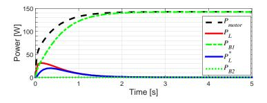
Figure III.4 – Behavior of power in roller-on-tire system
