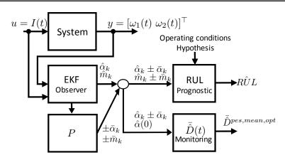
Figure IV.1 – Condition monitoring and RUL prognosis architecture.
