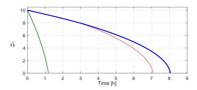
Figure V.9 – Estimated contact quality coefficient  $\hat{\alpha}$  in presence of operating conditions changes and for three different cases: 1) without RUL control (thin line), 2) with a RUL control without updating the RUL prediction (dotted line), and 3) with a RUL control which adapts the control actions according to the current RUL prediction (bold line).
