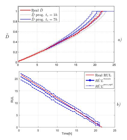
Figure IV.11 – Prognosis of RUL with an exogenous change in the system. a) Real deterioration trajectory  $\overline{D}$  with change in input (an augmentation of 20% over the nominal  $\sigma_{th}$  and  $\sigma_{tl}$  from  $t_c = 7h$ ), first prognostic at t = 0.5h (shaded lines) and updated prognostic just after the change at  $t_c = 7h$  (continuous lines); the updated prognostic is within the uncertainty interval. b) Prognostic of RUL per 0.5h with the exogenous change in the system.
