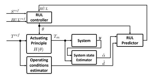
Figure V.2 – Architecture for an optimal control of the RUL.
