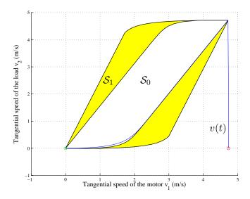
Figure III.16 – Robustly positive invariant sets for bounded electrical current  $(0 \le I(t) \le 20A)$ and admissible values of  $\alpha$  such that  $(\underline{\alpha} \le \alpha(t) \le \overline{\alpha})$ . A tangential speed v(t) out of these sets means that the actuator deterioration is not more admissible.
