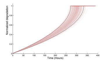
Figure IV.12 – Estimated deterioration for random input I(t), with mean 20A and a standard deviation of 0.5A. Here, 5% of the population age in more or less time than predicted (deterministic) bounded current case (i.e.  $19A \leq I(t) \leq 21A$ ).
