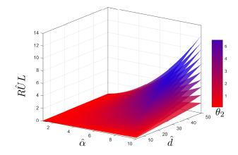
Figure V.5 – Predicted RUL as function of the parameter  $\theta_2$ , the estimated contact quality coefficient  $\hat{\alpha}$ , and the operating conditions  $\hat{d}$ .
