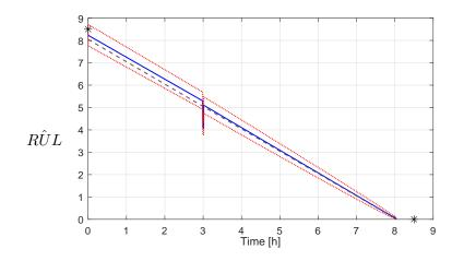
Figure V.6 – Predicted RUL along the useful lifetime: 1) by using the mean value of the estimated  $\alpha$  (solid line), 2) by using extreme values of the estimated  $\alpha$  (dotted line). Both compared to the obtained RUL (dashed line). The symbol \* represents the desired RUL.
