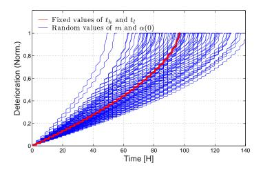
Figure III.14 – Internal mode of randomness. Deterioration D, for 100 random performances. m and  $\alpha(0)$  are used randomly using a normal distribution. Bold line: simulation of performance for the fixed central values  $m_m = 0.01$  and  $\alpha(0)_m = 10$ .
