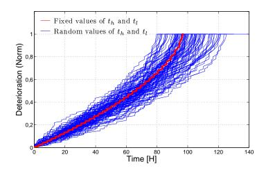
Figure III.15 – External mode of randomness. D, for 100 random trials.  $t_h$  and  $t_l$  are chosen randomly using an exponential distribution with mean values of  $\mu_{th} = 10000s$  and  $\mu_{tl} = 10s$  respectively. Bold line: simulation of performance for fixed values of  $t_h = 10000s$  and  $t_l = 10s$ .
