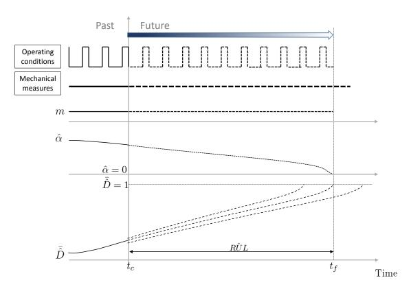
Figure IV.3 – Time diagram of a prognostic of the RUL at time  $t_c$ . At a given time  $t_c$ , a prognosis is performed, assuming future operation conditions. This prognostic can be updated as time goes on.
