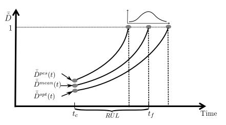
Figure IV.2 – Prognostic of the RUL at time  $t_c$ , by considering the current estimation uncertainties of  $\hat{\alpha}$  and  $\hat{m}$ , which result in an uncertainty in the calculation of the initial condition for prognostic of  $\overline{\hat{D}}$ . The resultant prognostic consist of three trajectories of deterioration: a mean trajectory and two bounds.
