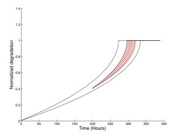
Figure IV.13 – Predicted deterioration trajectory at the very beginning and in future time (At t = 200 hours an initial condition  $\overline{D} = 0.4$ ), for random inputs I, with mean 20A and a standard deviation of 0.5A. Knowledge of the deterioration at this time allows a more accurate estimation of the remaining lifetime before outage of the actuator.
