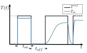
Figure V.3 – Examples of applied motor torque  $T_m$  compared to the desired one  $T^{ref}$ .
