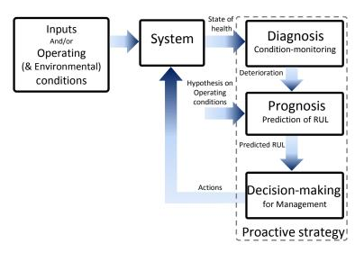
Figure II.5 – A post-prognosis set of actions for the system. The proactive actions include reaction to the failures, model of the deterioration, environmental conditions and response to a external inputs.
