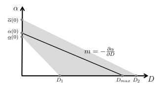
Figure III.3 – Contact quality coefficient  $\alpha$  as a function of D for m within a given interval  $\underline{m} \leq m \leq \overline{m}$ .
