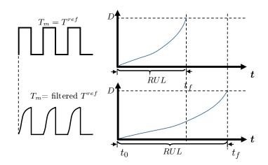
Figure V.1 – Illustration of the obtained RUL for two different sequences of the motor torque. The obtained RUL increases in cases where the motor torque is a filtered (or smoothed) signal of  $T^{ref}$ .
