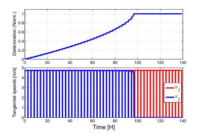
Figure III.12 – Normalized deterioration  $\overline{D}$ , tangential speed of motor  $v_1$  and tangential speed of wheel  $v_2$  for a rectangular waveform input with  $t_h = 10000s$  and  $t_l = 10s$ . It shows the failure of system at 96.7*h*.
