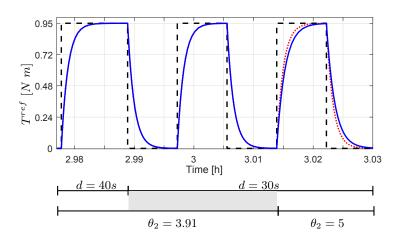
Figure V.8 – The desired torque  $T^{ref}$  (dashed line) and the applied motor torque  $T_m$  (solid line) - magnified view. For comparison, the dotted line corresponds to the applied torque without updating the value of the parameter  $\theta_2$ .
