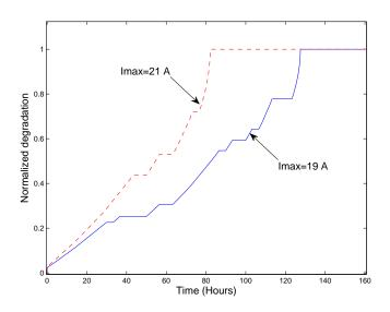
Figure IV.14 – Deterioration obtained with different maximal electrical currents for a predefined sequence of u(t).
