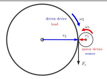
Figure III.2 – Basic roller-on-tire motor system
