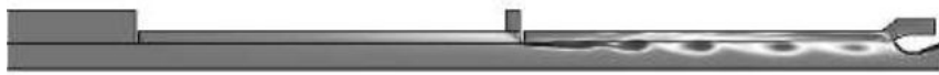
Figure 1.12: Figure taken from Vuillot et al. (Vuillot and Casalis 2004). Simulation of obstacle vortex shedding (OVS) in a LP3 motor, leading to five vortices traveling downstream from the inhibitor to the nozzle. This situation corresponds to m_h \simeq 5 .
