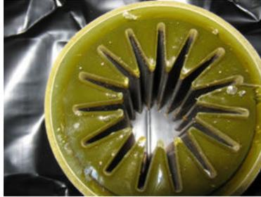
**Figure 1.3:** Star-shaped S1 propellant segment of a P230 1/35 scale motor. Picture taken from (Doisneau 2013)
