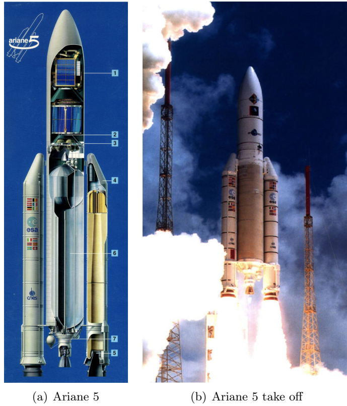
Figure 1.1: Subfigure (a) 1: Fairing, 2: L9/EPS storable propellant stage, 3: Vehicle equipment bay, 4: P230 SRM booster, 5: Booster nozzle, 6: H155/EPC main cryogenic stage, 7: Vulcain engine. Subfigure (b) ignited after the Vulcain engine, the two P230 boosters deliver more than 90% of total thrust at take off. Pictures taken from (Anthoine 2000).
