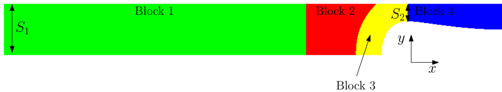
Figure J.1: Example of mesh for entropy spot-nozzle interaction. For a nozzle without a nozzle cavity.
