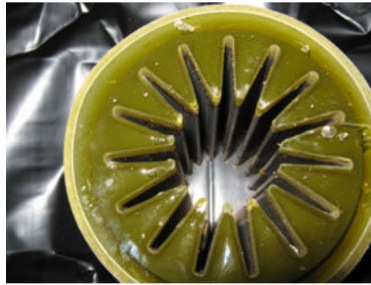
Figure 1.3: Star-shaped S1 propellant segment of a P230 1/35 scale motor. Picture taken from (Doisneau 2013)
