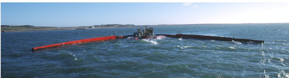
FIGURE 1.6 – Illustration du wave dragon, KOFOED et al. [61] et SORENSEN et al. [112]
