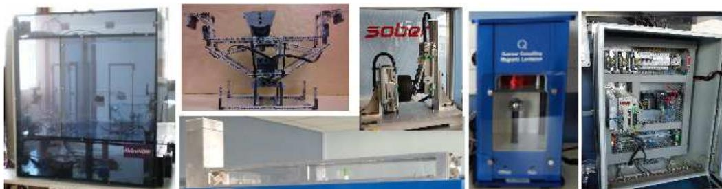
Figure 2.1: Pedagogical platform PhyAuto (from left to right): climate control over wireless networks in intelligent buildings, LEGO Mindstorm experiment (stabilizing an inverted half cube), quarter-scale vehicle for disturbance rejection with semi-active dampers, flow tube with heat and humidity regulation, magnetic suspension of a ball, and Programmable Logic Controllers for the quarter-scale vehicle and the flow tube.
