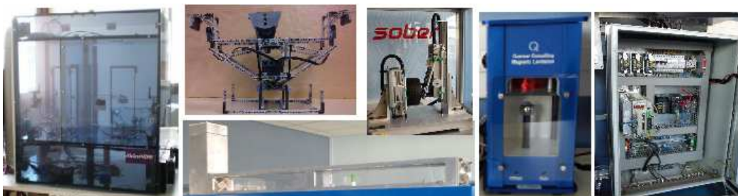
Figure 2.1: Pedagogical platform PhyAuto (from left to right): climate control over wireless networks in intelligent buildings, LEGO Mindstorm experiment (stabilizing an inverted half cube), quarter-scale vehicle for disturbance rejection with semi-active dampers, flow tube with heat and humidity regulation, magnetic suspension of a ball, and Programmable Logic Controllers for the quarter-scale vehicle and the flow tube.
