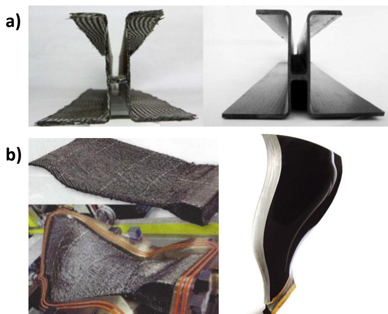
Figure 1.3- a) complex 3D woven preform geometry and composite stiffener [59] and, b) 3D woven preform applied to manufacture LEAP fan blade (Safran Aircraft Engines - Safran Group) [60].
