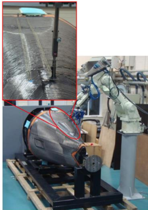
Figure 1.20 - Tail cone made of carbon composite reinforced by tufting technique [116].
