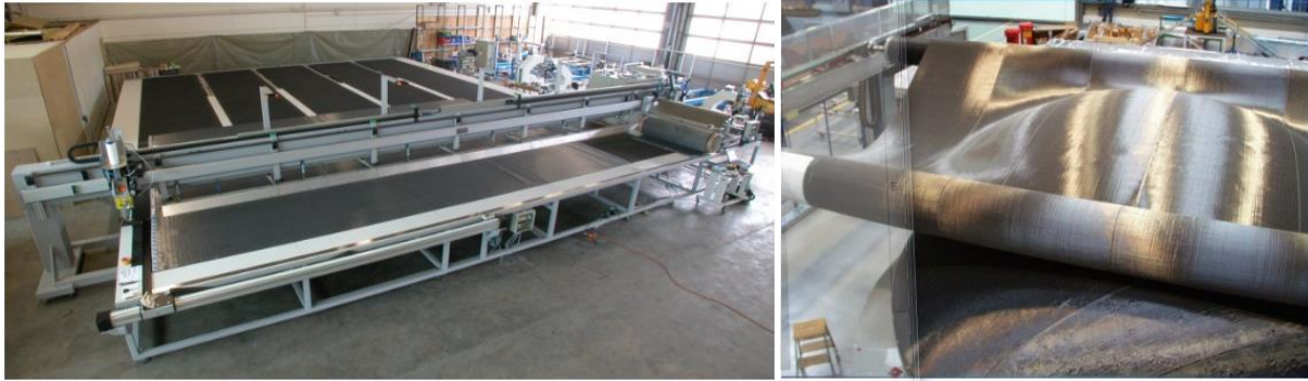
Figure 1.18- Dry-preforms joined together by blind stitching technique and laid on mold [159].
