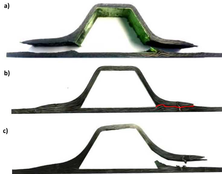
Figure 4.39 - Post-mortem images of a) REF, b) TUF1 and c) TUF2 specimens submitted to pull-off tests.
