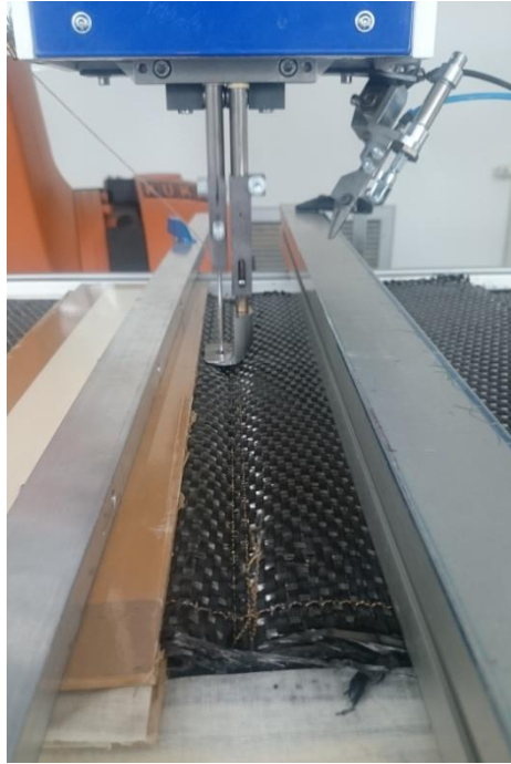
Figure 2.17 - The reinforcement between the stiffener and skin preforms for the manufacturing of the omega stringer.
