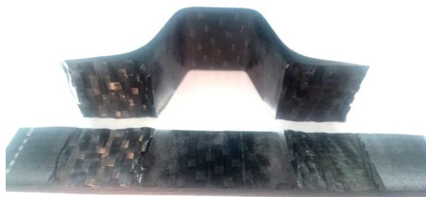
Figure 4.5 - Post-mortem image of the non-tufted omega stringer.
