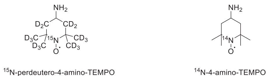
Figure 21: 15 N-perdeutero-4-amino-TEMPO and 14 N-4-amino-TEMPO used to functionalize an agarose-based matrix.
