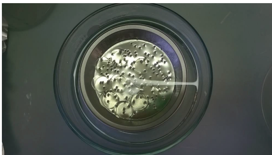
Figure 4: Aerogels immersed in acetone to remove water before being dried by supercritical CO 2 .
