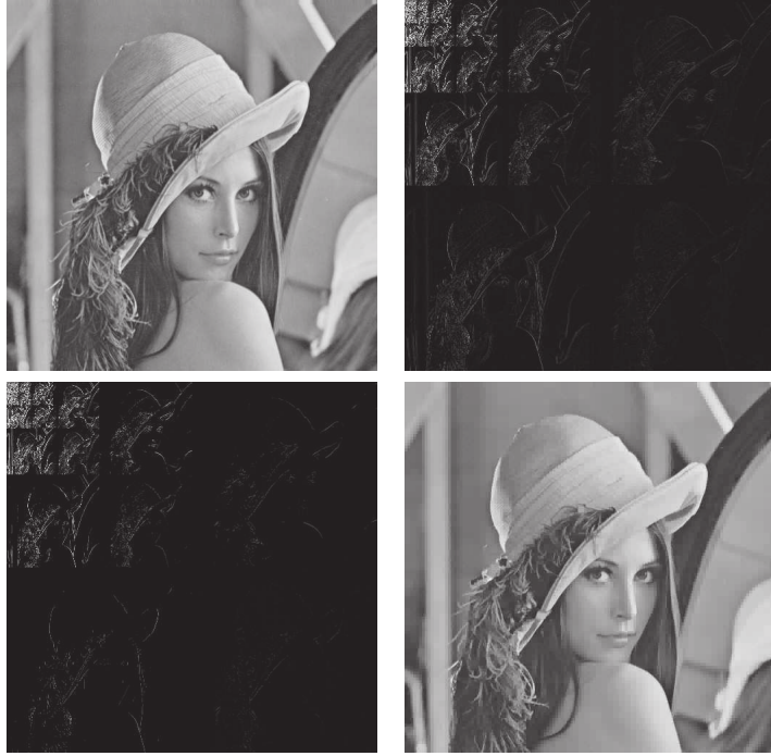
Figure 4.4: Top line: the original picture X and a representation of its wavelet transform WX . Bottom line: the matrix \bar{X} obtained after putting to zero 90% of the coefficients of WX , and the corresponding picture W^{-1}\bar{X} .
