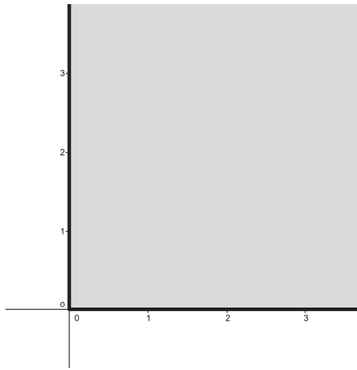
Figure 6.7: Pareto front in the value space Y = \mathbb{R}^2 . F(X) is in grey, the Pareto front is the thick black curve.
