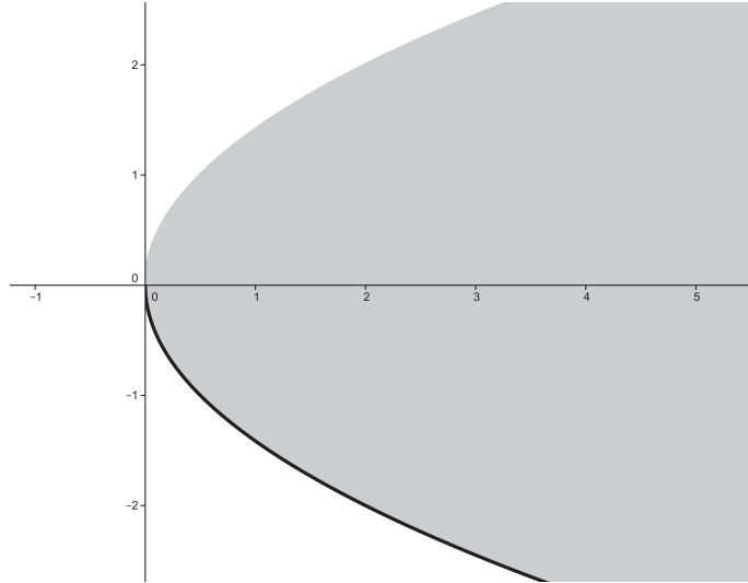
Figure 6.4: Pareto front in the value space Y = \mathbb{R}^2 . F(X) is in grey, the Pareto front is the thick black curve.
