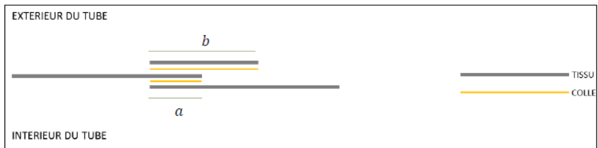
Fig. 50. How the glued parts are assembled
