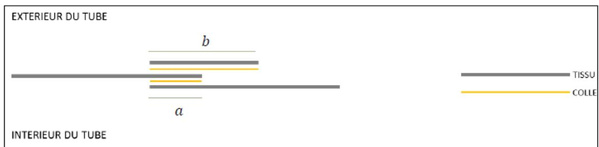
Fig. 50. How the glued parts are assembled
