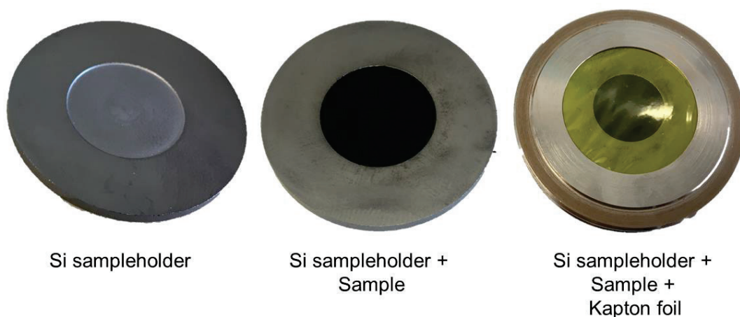
Figure 5-17: Samples preparation for XRD analysis.
