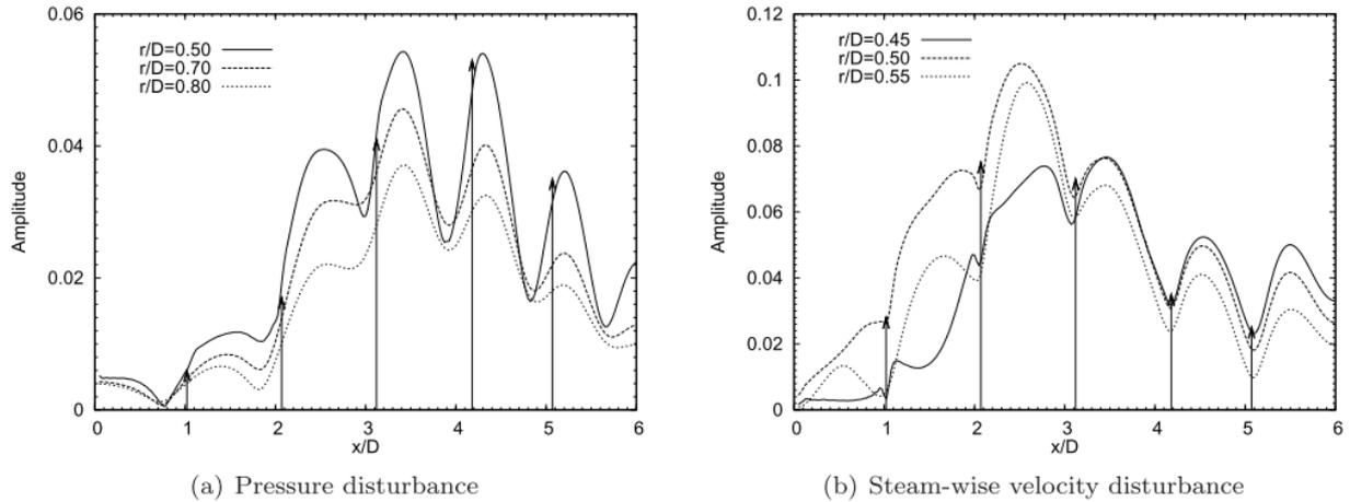
Figure 1. 25: a) amplitudes of the pressure fluctuations in the near field and b) steamwise velocity of screeching jets at  $M_j = 1.30$ . The vertical arrows in the figures represent shock locations. Gao & Li (2009).
