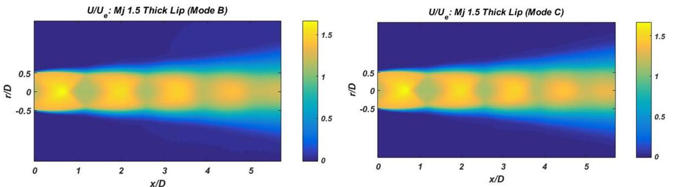
Figure 4. 3: longitudinal mean velocity ( $U$ ) normalized by  $U_e$ . Flapping (left) and helical (right) Screech modes.
