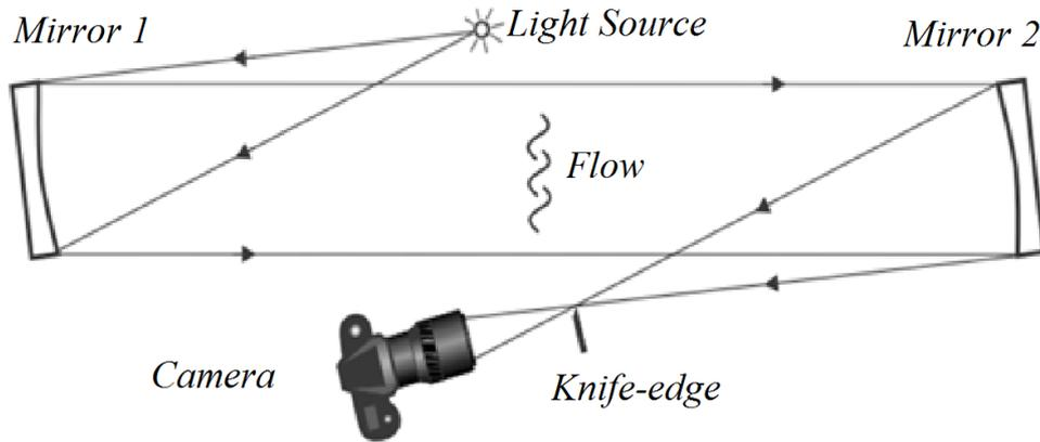
Figure 2. 4: Toepler Z-type Schlieren layout. Settles & Hargather (2017), modified.
