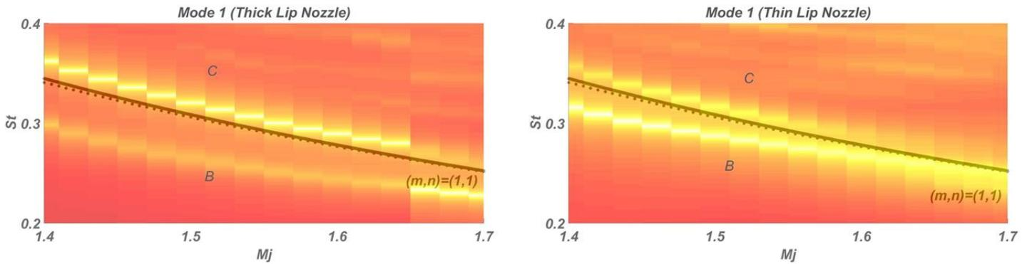
Figure 5. 6: allowable frequency ranges for helical ( $m=1, n=1$ ) upstream-travelling jet neutral waves overlapped on the PSD of the acoustic pressure cartography of the azimuthal Fourier mode 1. Thick (left) and thin (right) lip nozzle. Solid and dashed lines represent saddle and branch points, respectively.
