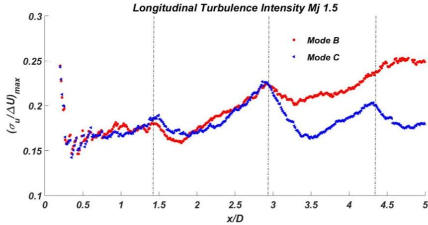
Figure 4. 10: maximum longitudinal turbulence intensity. Flapping (red) and helical Screech mode (blue). The shock positions are represented by dashed lines from Prandt-Pack's theory.
