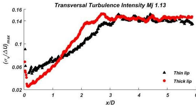
Figure 3. 25: maximum transversal turbulence intensity for  $M_j = 1.13$
