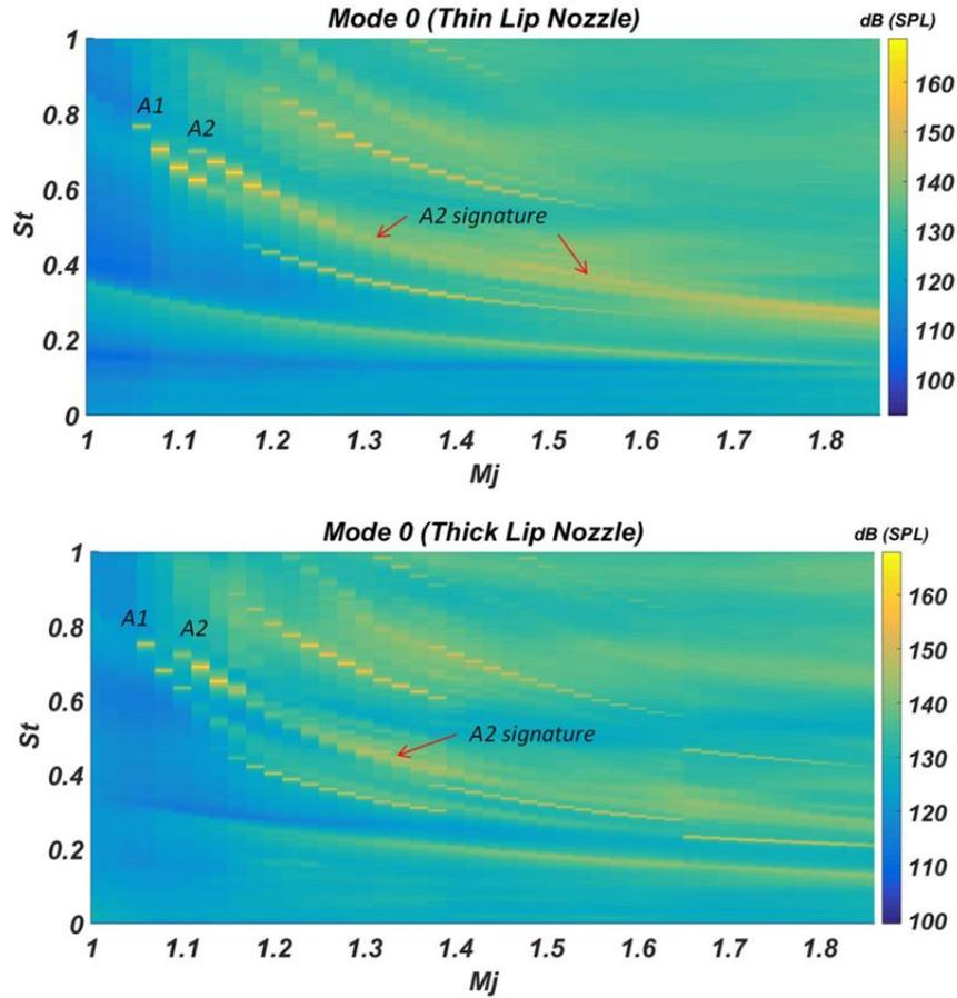
Figure 3. 3: cartography of the PSD of the first azimuthal mode ( $m=0$ ) of the near-field pressure as a function of  $St$  number and  $M_j$ . Effect of the nozzle lip on  $A1/A2$  Screech modes: thin (top) and thick lip (bottom).
