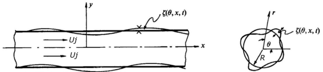
Figure 5. 2: sketch of cylindrical vortex-sheet. Tam & Hu (1989) modified.
