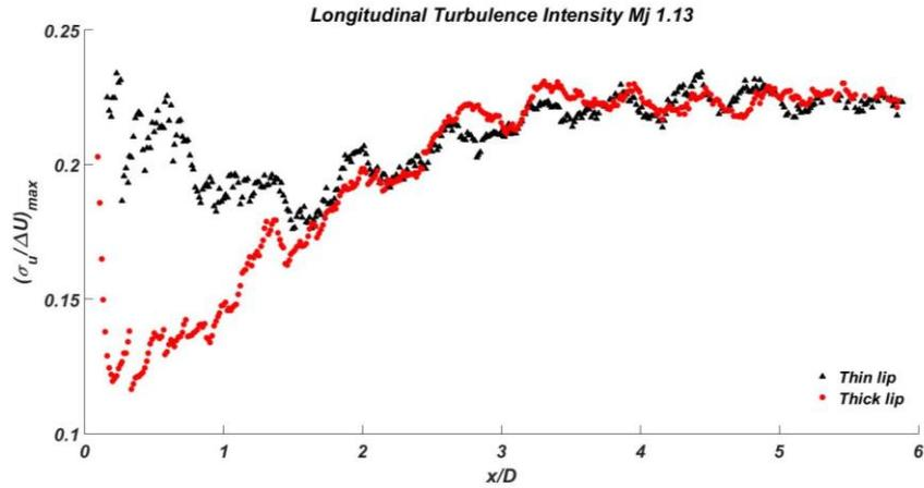
Figure 3. 22: maximum longitudinal turbulence intensity for  $M_j=1.13$ .
