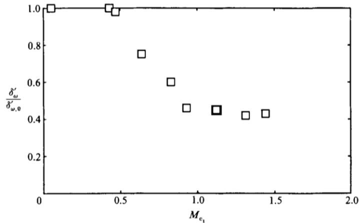
Figure 1. 4: experimental data of compressible mixing layer growth rate, normalized by incompressible value. Papamoschou & Roshko (1988).
