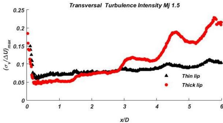
Figure 3. 27: maximum transversal turbulence intensity for  $Mj=1.5$ .
