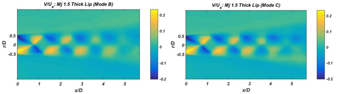
Figure 4. 4: transversal mean velocity ( $V$ ) normalized by  $Ue$ . Flapping (left) and helical (right) Screech modes.
