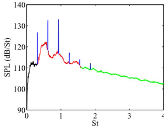
Figure 1. 13: typical jet noise spectrum of underexpanded nozzle in far field at  $M_j=1.35$ . The black line represents mixing noise, red line the broadband noise, blue line the screech noise and green line is the combination between mixing and broadband noise. André (2012).
