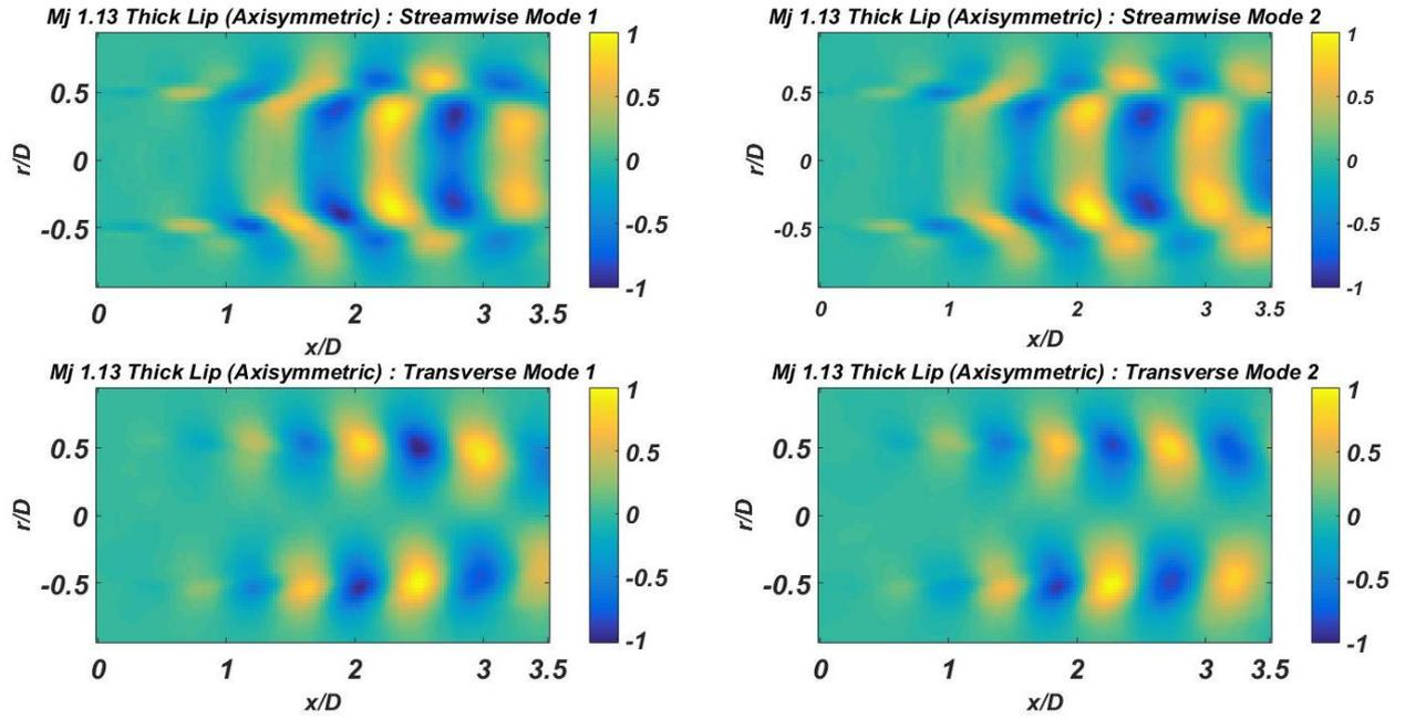
Figure 5. 7: spatial POD functions ( $\Phi$ ) of the modes 1 and 2, for the streamwise (top) and transverse (bottom) velocity components. Each mode is individually normalized by its respective maximum value of  $\Phi$ .
