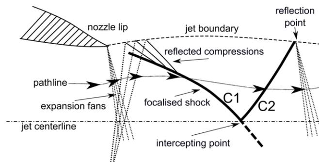
Figure 1. 6: shock-cell structure scheme. Savarese (2014).
