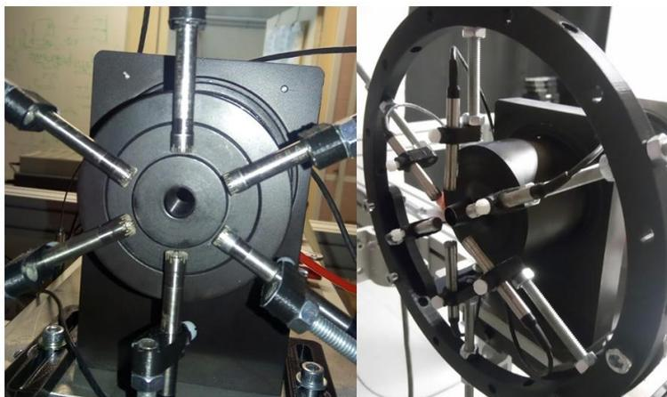
Figure 2. 3: microphone array employed for azimuthal Fourier decomposition.
