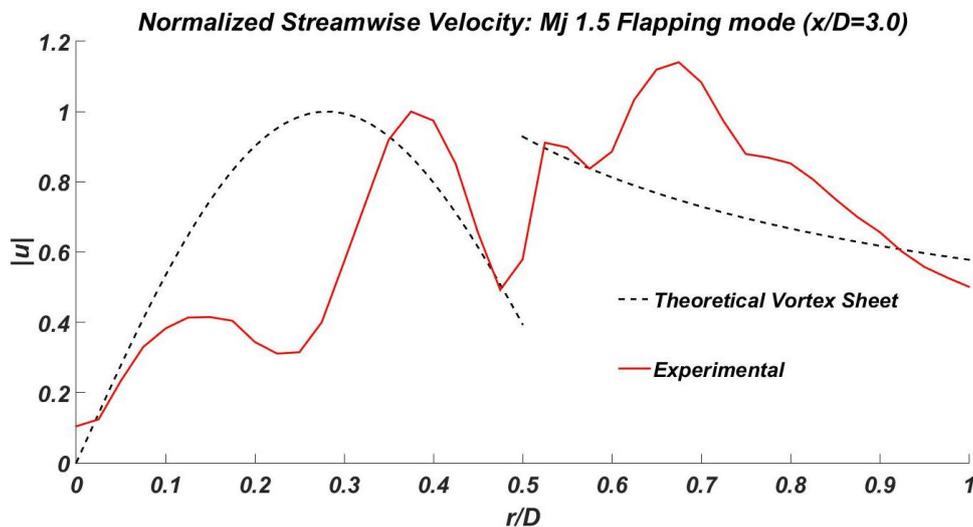
Figure 5. 28: Comparison between the amplitude of the velocity at the axial position  $x/D=3.0$  of the experimental upstream-travelling waves and theoretical vortex-sheet eigenfunction for  $k(m=1, n=1)$ .  $Mj=1.5$ , flapping mode ( $B$ ), the velocities are normalized by the maximum value inside of the jet.
