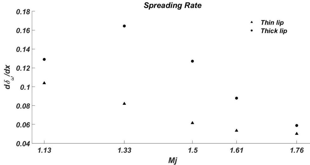
Figure 3. 15: spreading rate for all  $Mj$  conditions considered.
