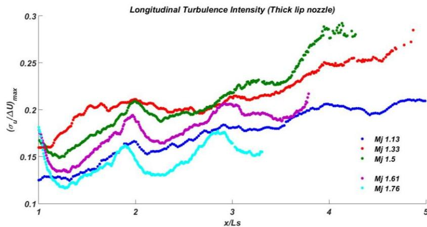
Figure 3. 31: maximum longitudinal turbulence vs shock-cell length for all  $M_j$  analysed conditions. Thick lip nozzle.
