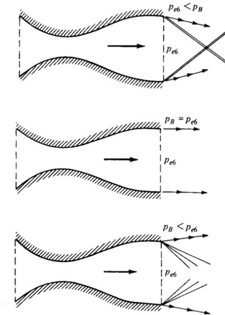
Figure 1. 1: three kinds of jet topology as a function of exit conditions. Overexpanded on the top, perfectly expanded in the middle and underexpanded at the bottom. Anderson Jr (1991).
