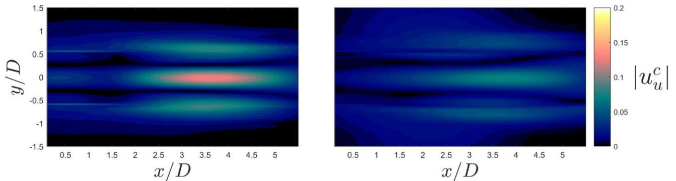
Figure 5. 12: amplitude of the upstream-travelling waves component associated to the negative wavenumbers ( $k^-$ ), normalized by the maximum value of  $u_u^c$ .  $M_j = 1.09$  left and  $1.14$  right. Edgington-Mitchell *et al.* (2018).
