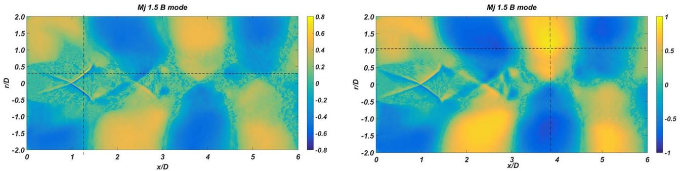
Figure 3. 37: correlation coefficient ( $R$ ) for the jet at  $Mj=1.5$  generated by thick lip nozzle. The reference points are represented by intersecting dashed lines: shock line (left) and standing wave (right).
