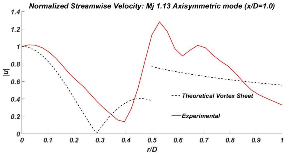
Figure 5. 14: Comparison between the amplitude of the velocity at the axial position  $x/D=1.0$  of the experimental upstream-travelling waves and the theoretical vortex-sheet eigenfunction for ( $m=0, n=2$ ).  $Mj=1.13$ , the velocities are normalized by their value at the jet axis ( $r/D=0$ ).
