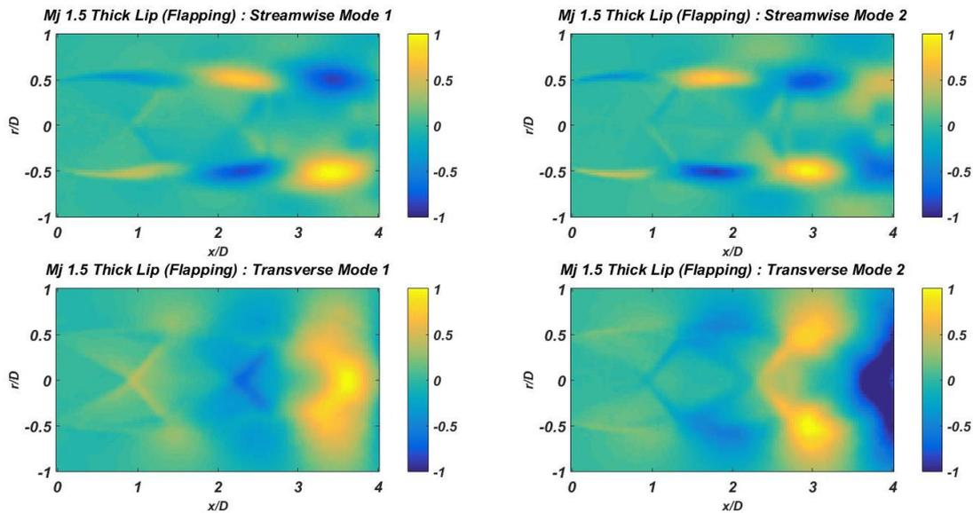
Figure 5. 22: spatial POD functions ( $\Phi$ ) of the modes 1 and 2, for the streamwise (top) and transverse (bottom) velocity components. Each mode is individually normalized by the respective maximum value of  $\Phi$ .
