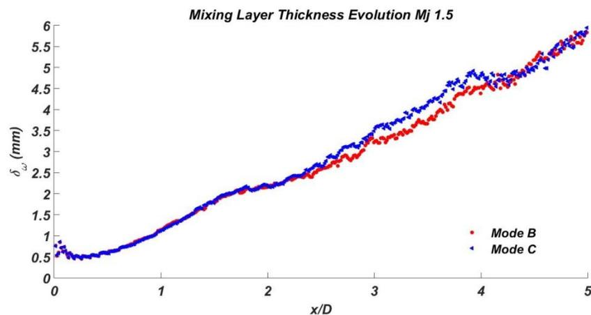
Figure 4. 7: mixing layer thickness evolution. Flapping (red) and helical Screech mode (blue).
