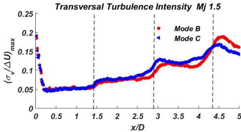
Figure 4. 11: maximum transversal turbulence intensity. Flapping (red) and helical Screech mode (blue). The shock positions are represented by dashed lines from Prandt-Pack's theory.
