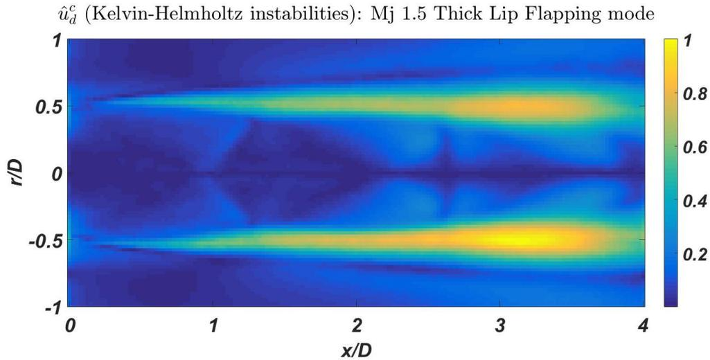
Figure 5. 25: amplitude of the downstream travelling waves normalized by the maximum value.
