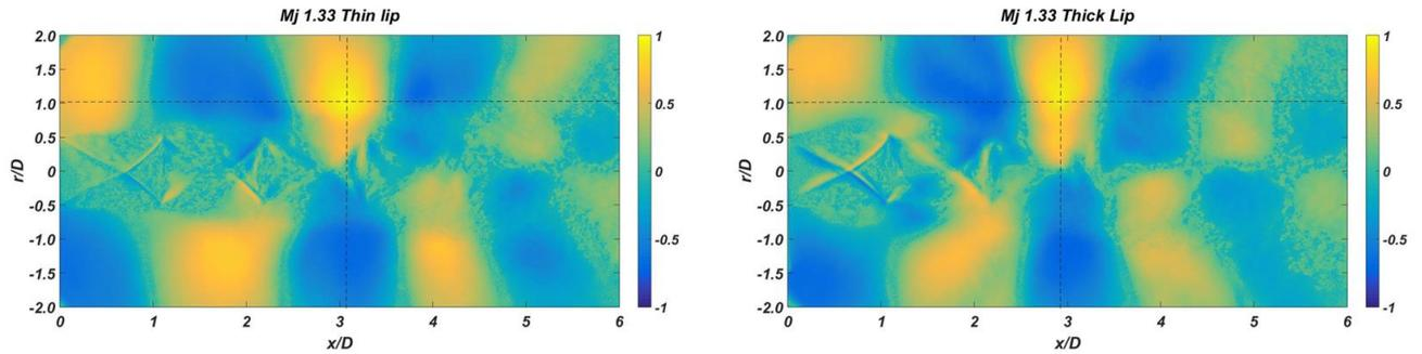
Figure 3. 38: correlation coefficient ( $R$ ) for the jet at  $Mj=1.33$ . The reference point is located inside the standing waves and is represented by the intersecting dashed lines. Thin (left) and thick (right) lip nozzle.
