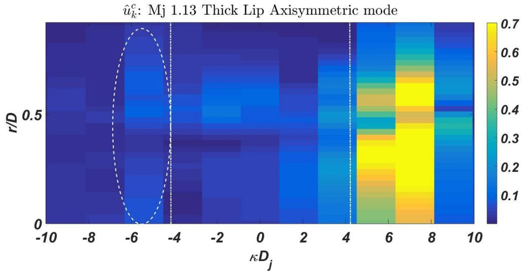
Figure 5. 9: wavenumber spectrum of the coherent streamwise velocity ( $\hat{u}_k^c$ ). Vertical dashed lines represent the wavenumbers associated to the speed of sound at the Screech frequency in the upstream (negative values) and downstream (positive values) directions.
