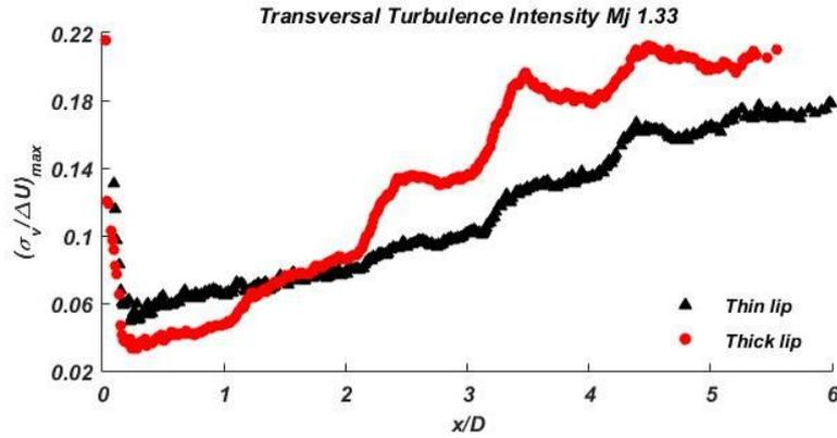
Figure 3. 26: maximum transversal turbulence intensity for  $Mj=1.33$ .
