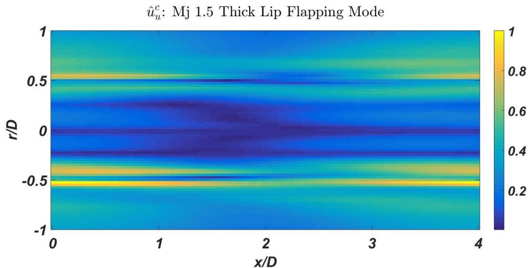
Figure 5. 26: amplitude of the upstream-travelling waves component associated to the negative wavenumbers ( $kD_j = -3.4$  and  $-5.1$ ), normalized by the maximum value.
