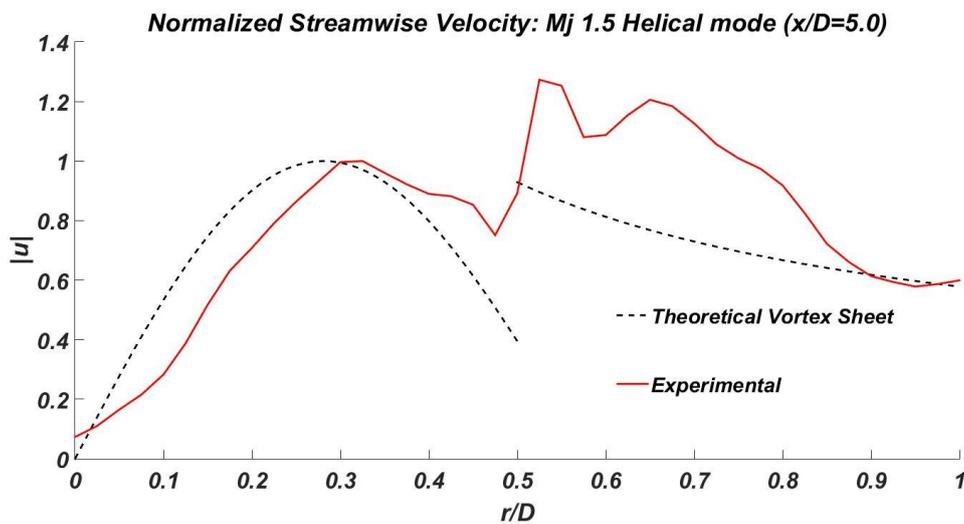
Figure 5. 21: Comparison between the amplitude of the velocity at the axial position  $x/D=5.0$  of the experimental upstream-travelling waves and the theoretical vortex-sheet eigenfunction for  $k(m=1, n=1)$ ,  $M_j=1.5$ . The velocities are normalized by the maximum value inside of the jet.
