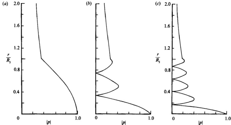
Figure 5. 1: pressure eigenfunction of upstream subsonic waves. Cold jets, Mach number 1.5. a) (0,1) mode,  $\kappa R_j=0.7$ , b) (0,3) mode,  $\kappa R_j=3.0$ , and c) (0,5) mode,  $\kappa R_j=5.5$ . Tam & Hu (1989).
