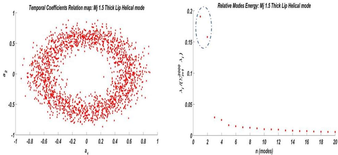
Figure 4. 18: phase portrait of the temporal coefficients  $a_1$  and  $a_2$  (left). Relative POD modes energy (right) for the helical  $C$  Screech mode.
