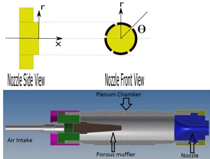
Figure 2. 2: coordinates system centered at the nozzle exit (top) and layout of supersonic flow facility (bottom).
