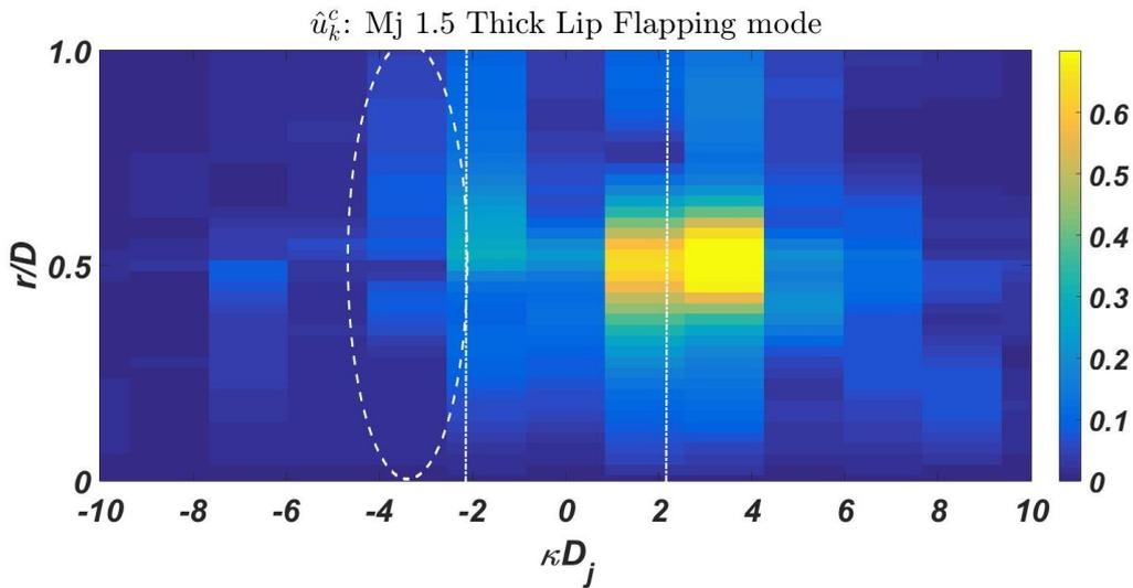
Figure 5. 24: wavenumber spectrum of the coherent streamwise velocity ( $\hat{u}_k^c$ ). Vertical dashed lines represent the wavenumbers associated to the speed of sound at the Screech frequency in the upstream (negative values) and downstream (positive values) directions.
