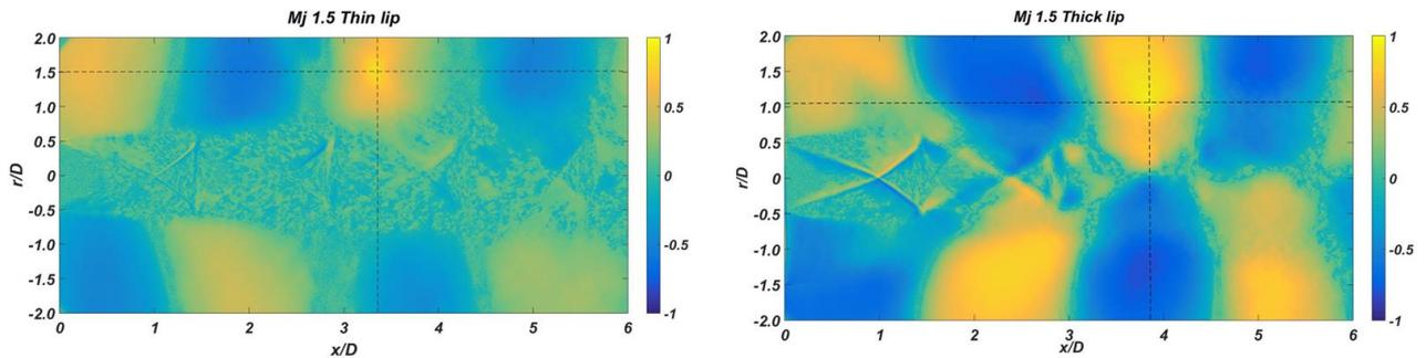
Figure 3. 39: correlation coefficient ( $R$ ) for the jet at  $Mj=1.5$ . The reference point is located inside the standing waves and is represented by the intersecting dashed lines. Thin (left) and thick (right) lip nozzle.
