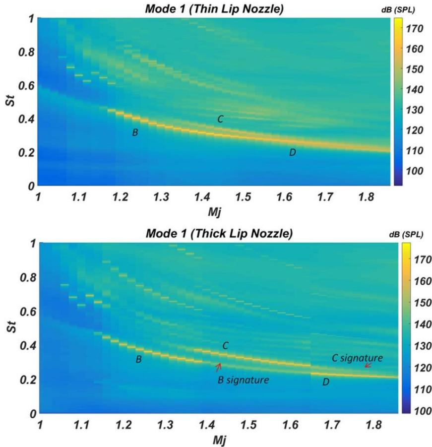
Figure 3. 4: cartography of the PSD of the first azimuthal mode ( $m=1$ ) of the near-field pressure as a function of  $St$  number and  $M_j$ . Effect of the nozzle lip on  $B/C/D$  Screech modes: thin (top) and thick lip (bottom).
