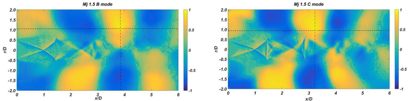
Figure 4. 14: correlation coefficient ( $R$ ). The reference point is placed in the standing waves and represented by intersecting dashed lines. Jet under dominant flapping  $B$  (left) and helical  $C$  (right) Screech mode.
