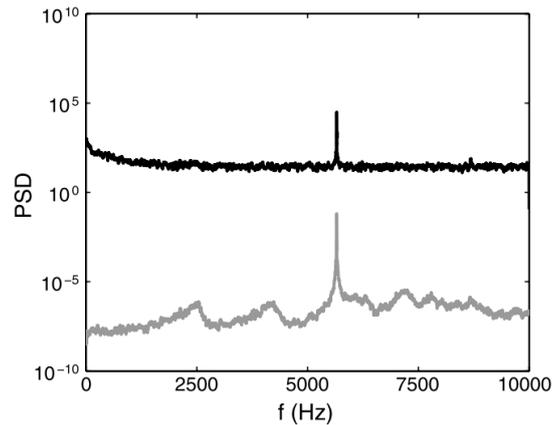
Figure 1. 11: PSD (Power Spectral Density) of near-field microphone signal (gray) and  $\text{PSD} \times 10^5$  of the signal of containing the axial location at the first shock tip at NPR 2.27 (black). André et al. (2011).
