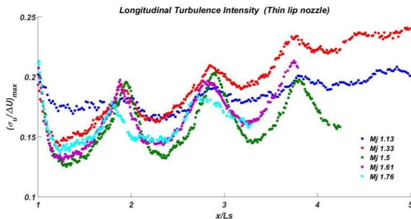
Figure 3. 32: maximum longitudinal turbulence vs shock cell length for all  $M_j$  analysed conditions. Thin lip nozzle.
