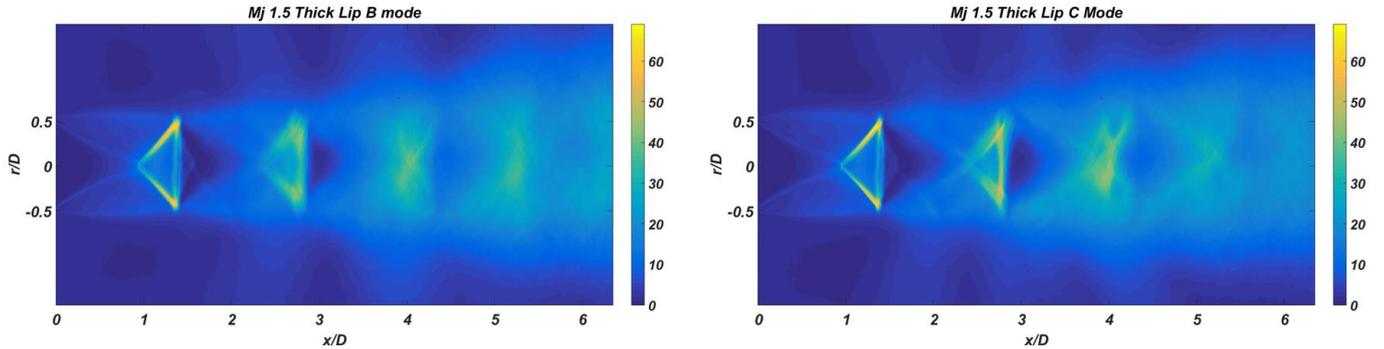
Figure 4. 2: *rms* intensity of grey level fluctuations. *B* flapping (left) and *C* helical modes (right).
