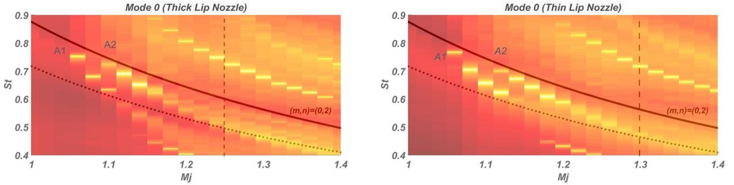
Figure 5. 5: allowable frequency ranges for axisymmetric ( $m=0, n=2$ ) upstream-travelling jet neutral waves overlapped on the PSD of the acoustic pressure cartography of the axisymmetric azimuthal Fourier mode. Thick (left) and thin (right) lip nozzle. Solid and dashed lines represent saddle and branch points, respectively.
