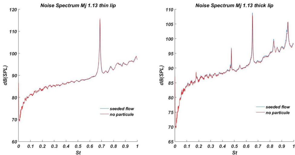
Figure 2. 9: particle effect in the noise spectrum for  $M_j=1.13$ , thin (left) and thick (right) lip nozzle.
