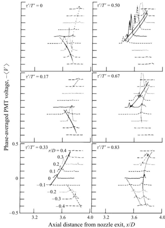
Figure 1. 10: phase-average PMT data obtained at nine radial positions, on third shock in  $M_j=1.42$  and at the different phases of Screech cycle ( $\tau/T_s$ ). Panda (1998).
