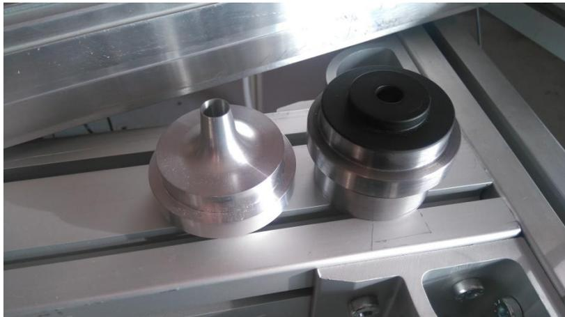
Figure 2. 1: evaluated nozzles. Thin lip (left) and thick lip (right).
