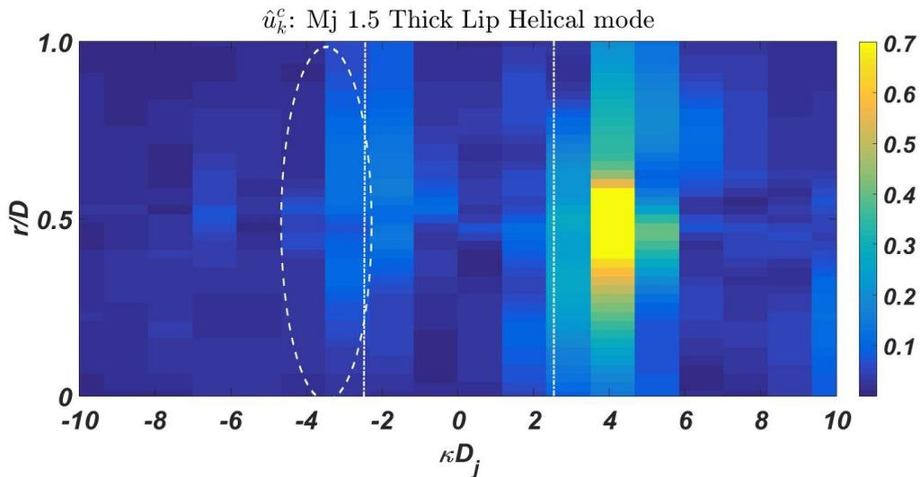
Figure 5. 17: wavenumber spectrum of the coherent streamwise velocity ( $\hat{u}_k^c$ ). Vertical dashed lines represent the wavenumbers associated to the speed of sound at the Screech frequency in the upstream (negative values) and downstream (positive values) directions.
