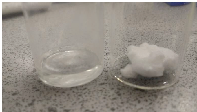
Figure 104: Picture of autoclave contents upon depressurisation for the dispersion polymerisation of PMMA in scCO_2 at 35°C and 276 bar using 5 wt.% of P(VAc-stat-VPI)-block-PNVP-X2 ( Table 20, entry 1 ).
