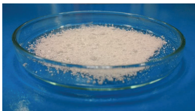
Figure 97: PNVP polymer powder made by dispersion polymerisation in scCO_2 using 5 wt% of P(VAc-stat-VPi)-X2 (Table 188, entry 2).
