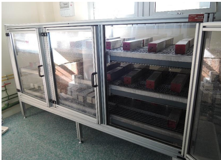
Figure 2-23: Real atomized device for humidification/drying cycles
