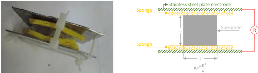
Figure 2-2: Uniaxial measurement of the specimen resistance
