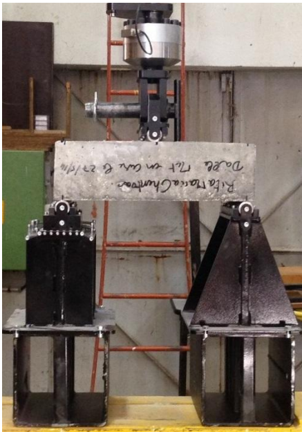
Figure 2-30: Cracking protocol of the concrete slabs
