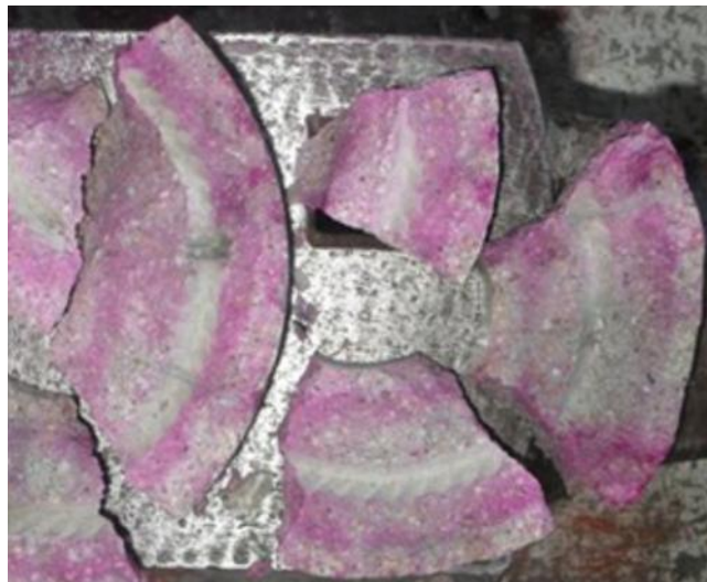
Figure 3-15: Phenolphthalein pH test on a ring shape mortar specimen carbonated at 50% CO 2 for 7 days [173]
