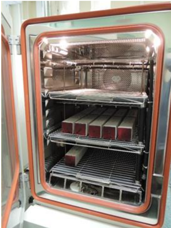
Figure 2-25 : Plans and real view of the adapted climatic raining chamber
