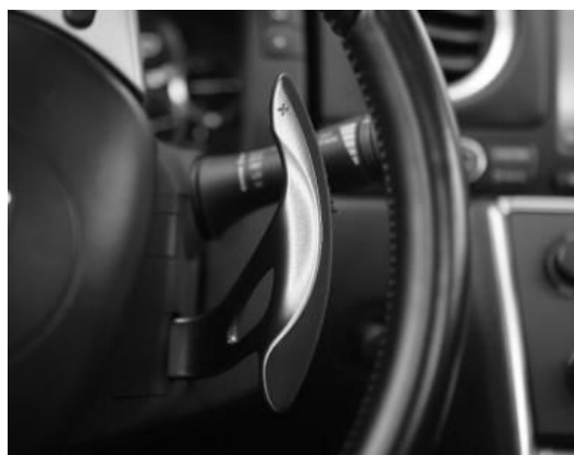
Figure 22. Semi-automatic gear shifter (TRCG, 2015)
