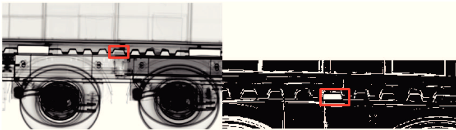
Figure 5.53 – Chassis inspection using registration
