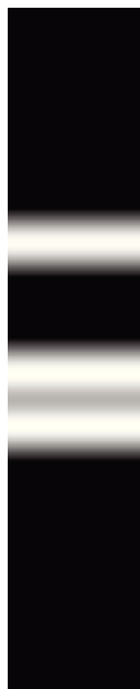
Figure 3.14 – Mask composed of Gaussians as described in equation 3.59. It is used to confine the diffusion process to sub-images boundaries.
