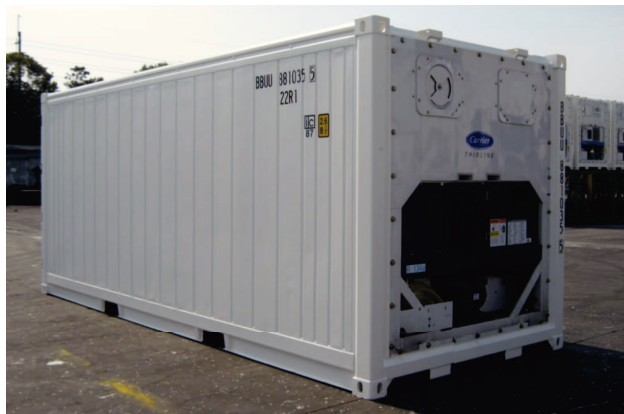
Figure 5.4 – Refrigerated ISO container.
