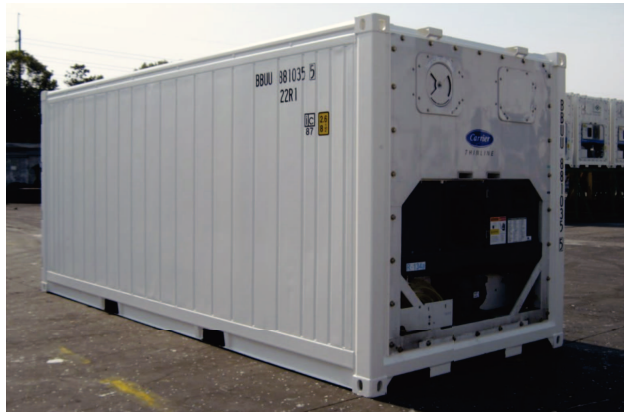
Figure 5.4 – Refrigerated ISO container.
