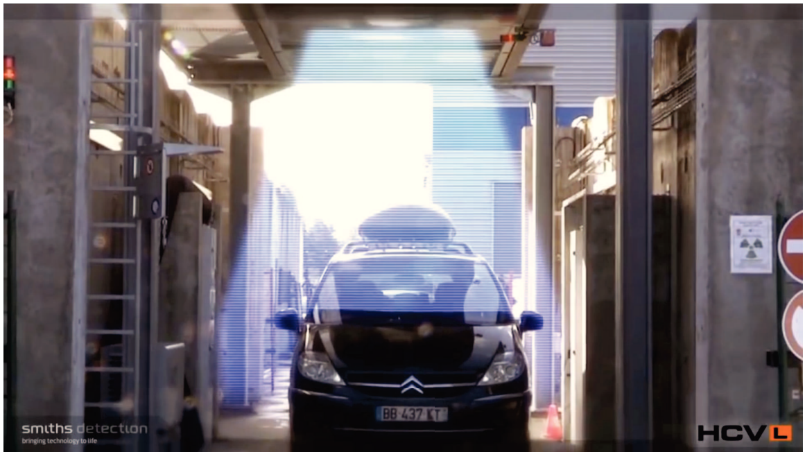
Figure 6.37 – Illustration of X-ray beam during scanning.
