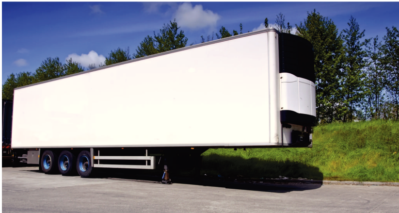
Figure 5.5 – Refrigerated trailer example. The air-cooler module is placed outside of the trailer.
