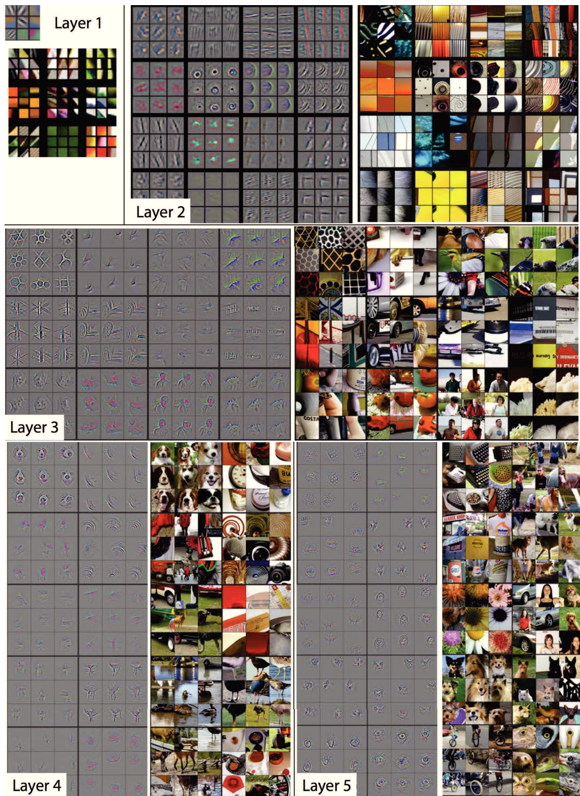
Figure 2.10 – Visualization of bottom to top levels activations. As described, responses become more and more abstract as layers get deeper (from [133]).
