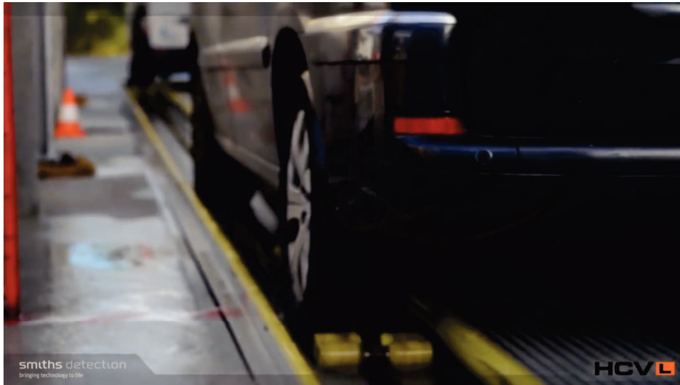
Figure 6.8 – The conveyor rollers (in yellow) applying a pushing force on the rear wheels before scanning.
