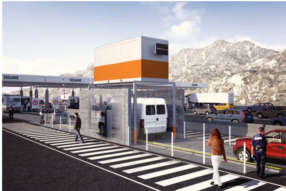
Figure 6.1 – HCVL system representation. Each vehicle is trailed slowly to be imaged.
