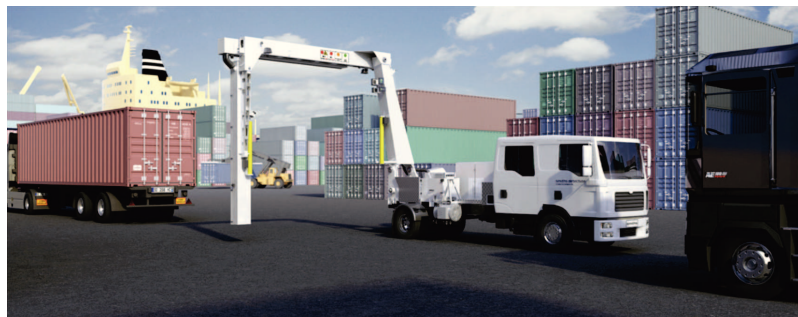
Figure 21 – HCVMe X-ray machine
