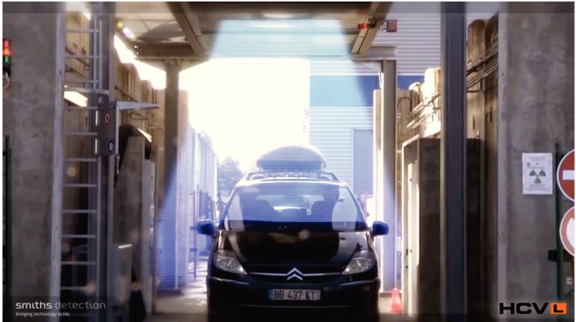
Figure 6.37 – Illustration of X-ray beam during scanning.
