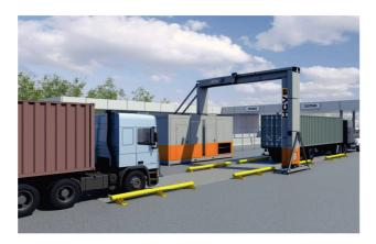
Figure 18 - HCVP scanning machine
