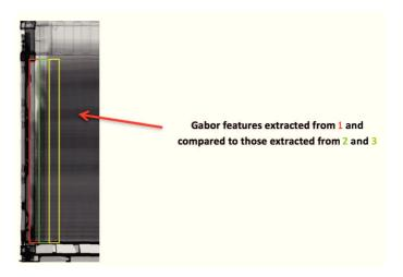
Figure 5.60 – Possible irregularity checking technique in case of cluttered region.
