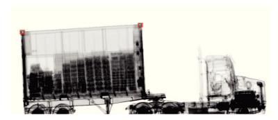
Figure 5.9 – ISO container scanned by the HCVM system. Illustration of corner patches extracted for SVM classification.
