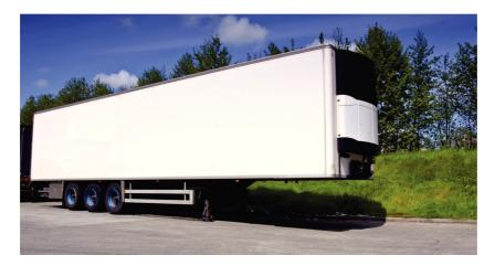
Figure 5.5 – Refrigerated trailer example. The air-cooler module is placed outside of the trailer.
