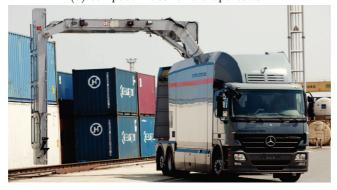
(b) scanning arm deployed
