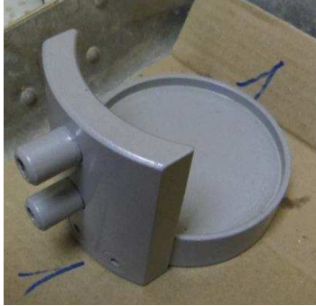
Figure 59 – Support with guides to make holes in the sample to insert the tensiometers.
