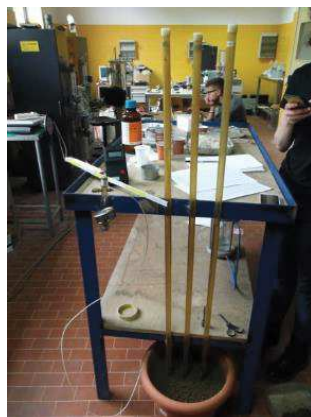
Figure 107 – SDEC France tensiometers with different initial air columns.
