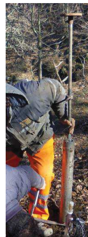
Figure 99 – Tube and extension used to open a borehole for the installation of TDR probes.
