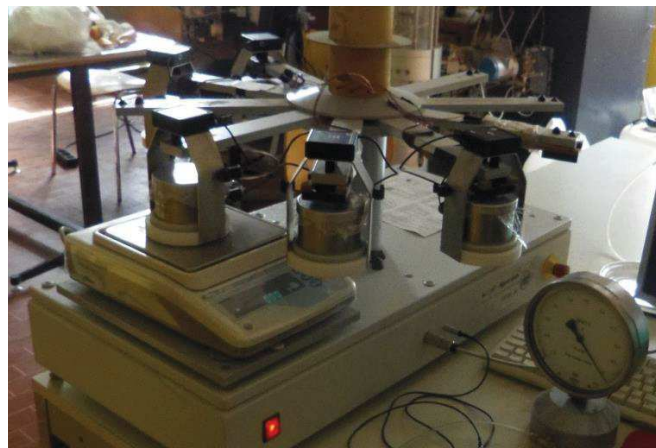
Figure 52 – ku-pf apparatus used in the experimentation.
