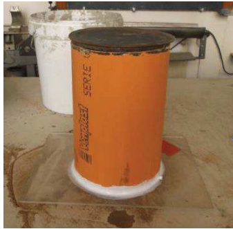
Figure 102 – Plexiglas base glued to the mould.
