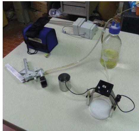
Figure 56 – Setup of the saturation of tensiometers.
