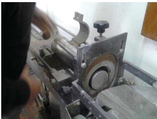
Figure 47 – Soil sample extrusion from the borehole.
