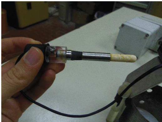
Figure 55 – Tensiometer (do not hold the tensiometer in this manner during the saturation).
