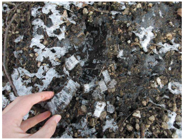
Figure 42 – Formation of a frozen soil layer.
