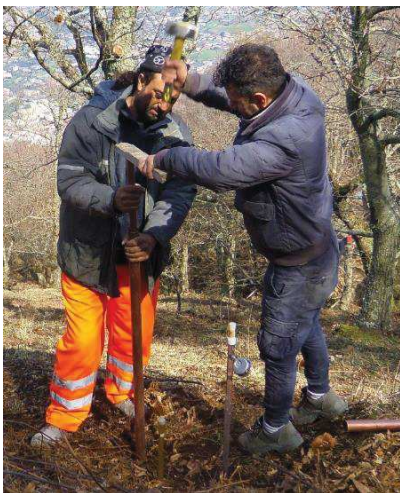
Figure 98 – Interior and exterior cooper tubes to install tensiometers.
