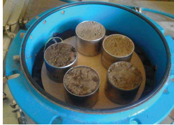
Figure 62 – Position of the samples inside the pressure plate chamber.
