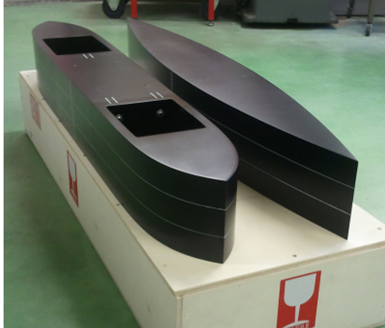
Figure 3.3.: Picture of CWn8 (left) and CWn2 (right) model ship hulls Source: Caplier et al. (2015)
