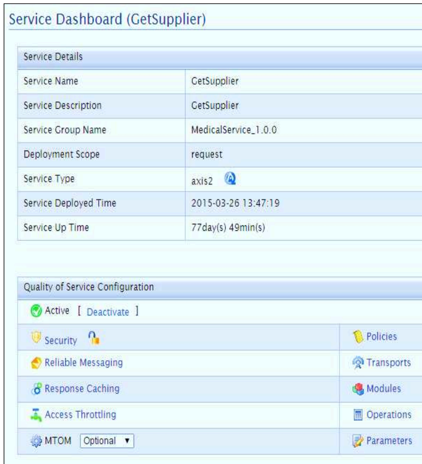
Figure 17: GetSupplier Service Information in WSO2 server (Upper part: Service Statistics. Lower part: QoS Configuration)
