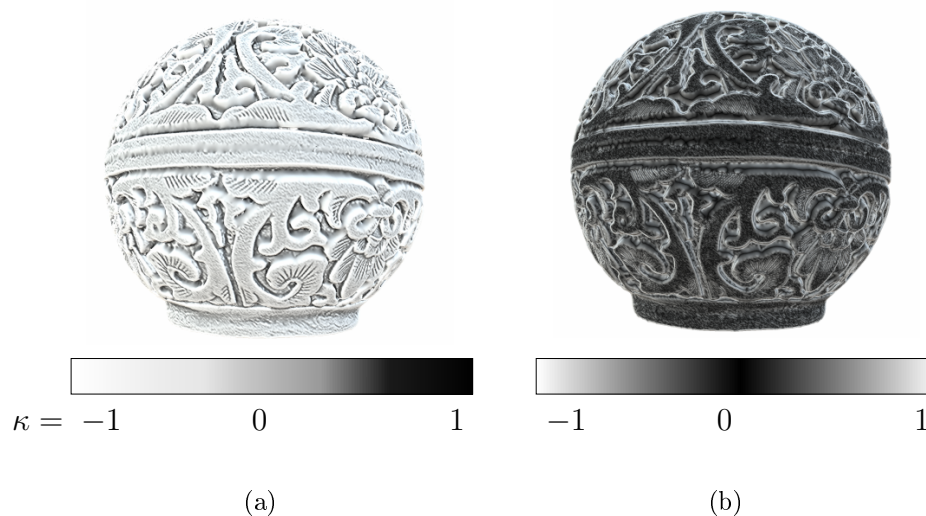
Figure 2.8 – (a) The transfer function we use to modulate shading brightens convexities and darkens concavities. (b) Another example: bright curved surfaces, dark flat ones.
