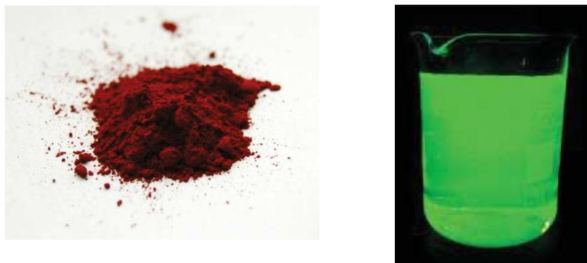
**Figure 3.5** Fluorescein in various forms, on the right is disodium salt which is also known as “uranin” and on the left is dissolution in the water with typical bright green color.
