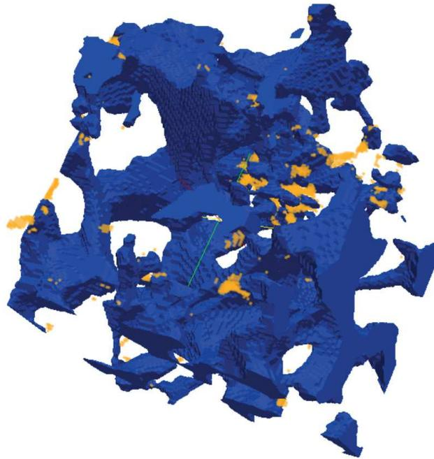
Figure 4.4 3-dimensional visualization of pore-space network (blue) and connected microporosity (yellow)
