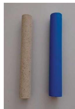
Figure 3.3 Cross section through experimental cell for laboratory tracer experiment (a) and different stages of preparing core samples; b) Berea sandstone block from which core is extracted; c) coring machine at Geosciences Montpellier laboratory and d) on the left Berea sandstone core and on the right same core coated with thermo-plastic coating
