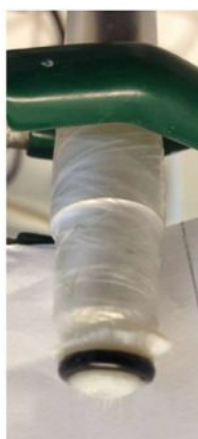
Fig 96 Legend and figure from the paper of Nocchi et al. [157]. Photo of oxygen electrode covered with skin membrane.
