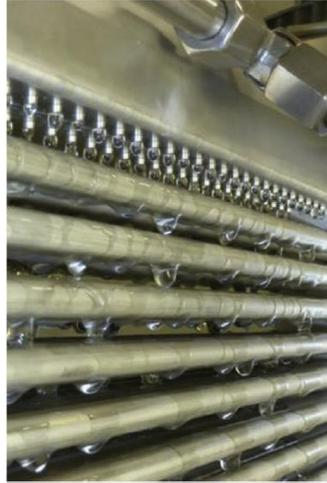
Figure 1.13. Falling film bundle heat and mass exchanger considered in the sorption reaction zone (Daguenet-Frick et al, 2016)
