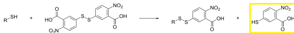
Figure 6.8: DTNB reaction with thiol. The reaction releases TNB 2- that can be quantified by spectrophotometry.
