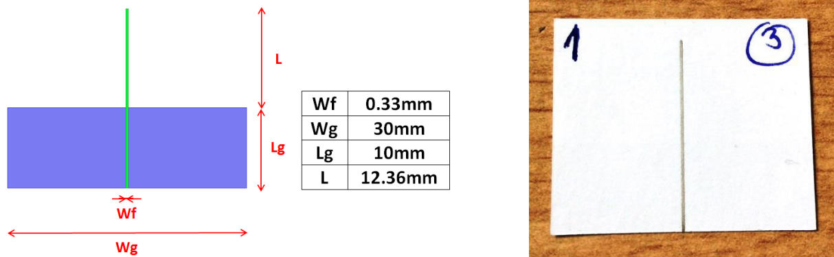
Figure 3-7: Layout and prototype of the 5GHz monopole antenna, screen-printed on E4D-100 \mu m paper
