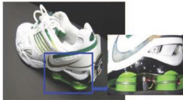
Figure 1-58: Self-powered RFID shoe with mounted electronics
