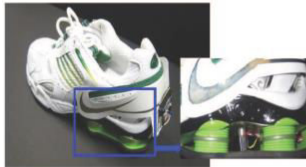
Figure 1-58: Self-powered RFID shoe with mounted electronics
