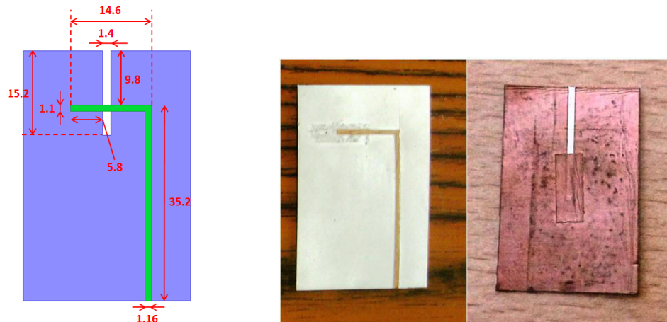
Figure 3-19: Layout and prototype of the ultra-wideband dipole antenna, fabricated with adhesive copper tape on Teslin-250 \mu m paper
