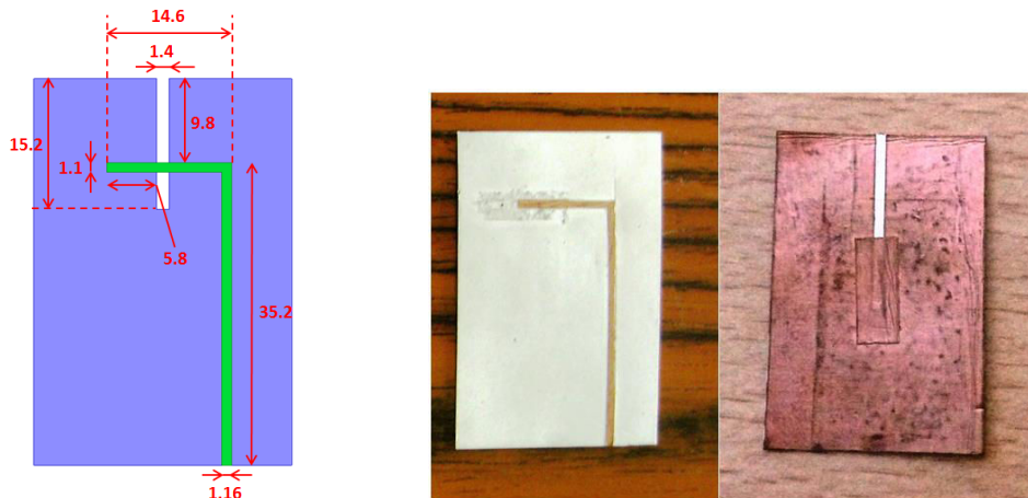
Figure 3-19: Layout and prototype of the ultra-wideband dipole antenna, fabricated with adhesive copper tape on Teslin-250 \mu m paper
