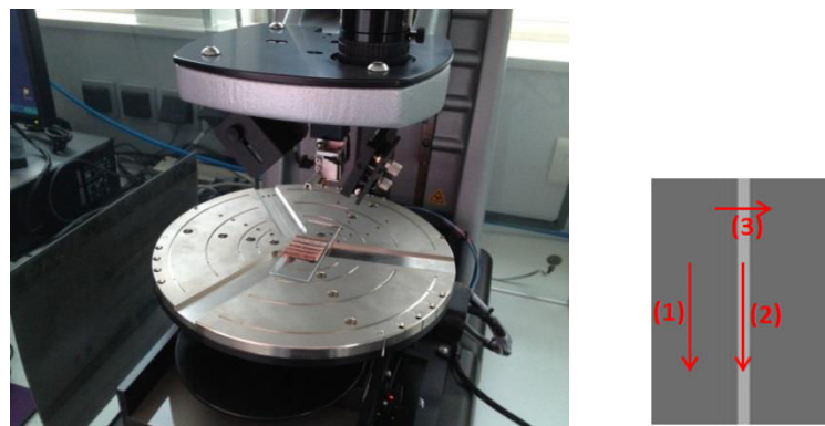
Figure 2-43: Measurement of the deposit thickness with a Veeco mechanical profilometer at UBO
