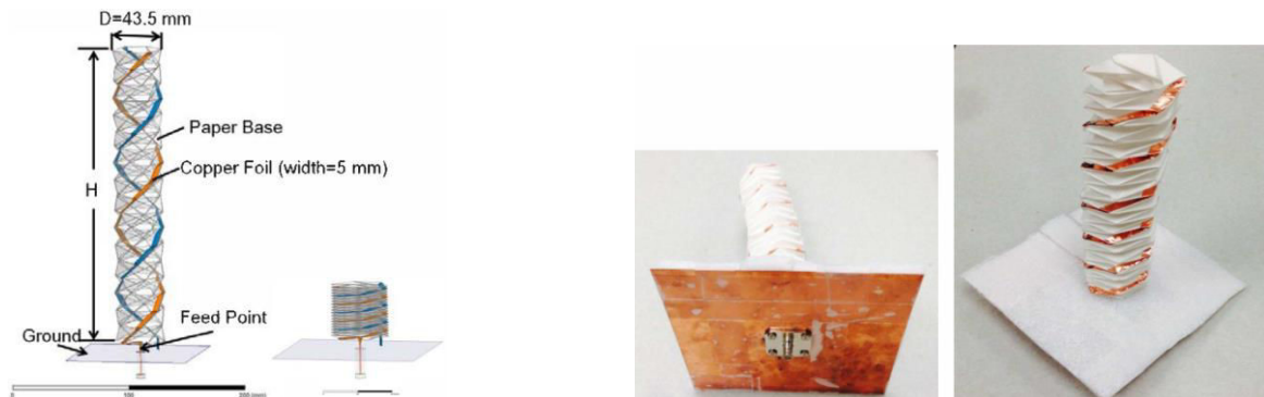
Figure 1-49: Simulated model [L] and manufactured prototype [R] of the 18-steps origami helical antenna
