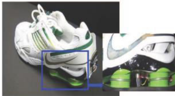
Figure 1-58: Self-powered RFID shoe with mounted electronics
