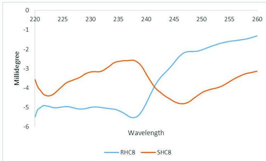
Figure 73: CD spectra of RHC8 and SHC8 in pure methanol (high concentration, 50mM). Step size 0.5nm.
