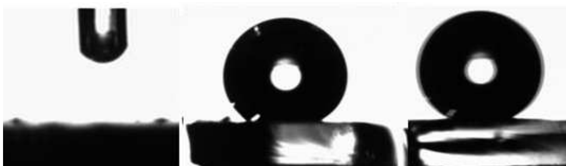
Figure 92: Contact angle measurements. Left: silica electrode, complete dispersion, angle =0°, middle C6 modified electrode, hydrophobic surface, angle=145.5°, right doped electrode, hydrophobic surface angle=149.3°.
