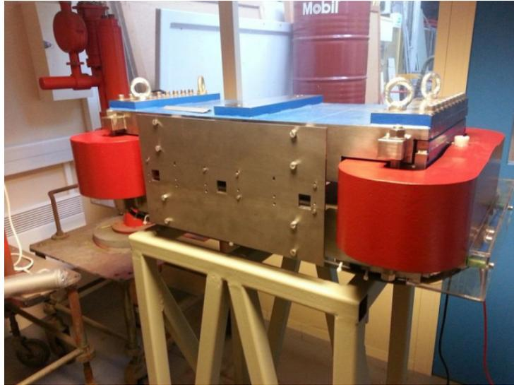
Figure 4.9: The dipole magnet with the protection screen against stray field.
