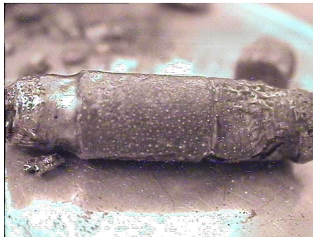
Figure II-49: VERDON-4 fuel elements recovered after the VERDON-4 test
