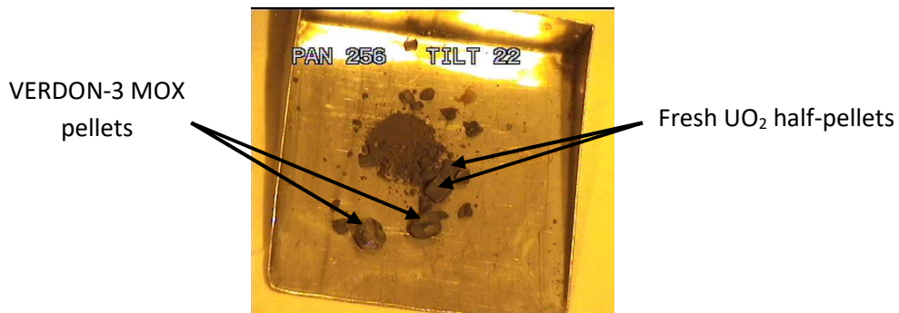
Figure II-17: VERDON-3 pellets and debris recovered from the case
