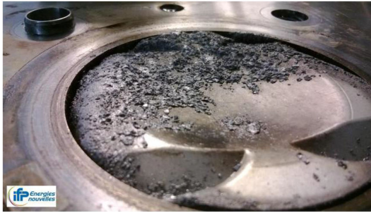
Figure 1.8: Erosion of the piston due to knocking combustion
