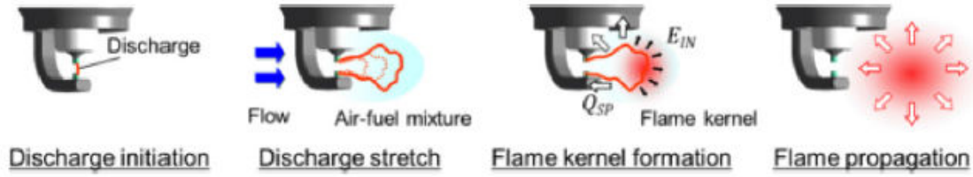
Figure 3.8: Ignition process from spark-discharge to turbulent premixed flame propagation. Reprinted from [55].
