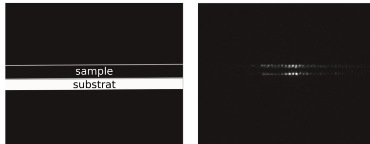
Figure III.15 – Mode observed after reflection on air prism with input power of 5 mW and camera integration time of 300 \mu s (input edge) (magnification \times 5 ).
