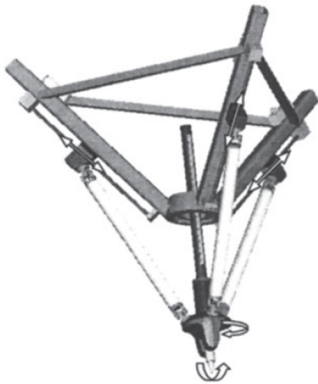
Figure 1.15 – A 5- dof industrial hybrid manipulator [TGK99].
