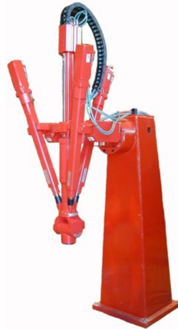
Figure 1.16 – Tricept modular hybrid robot [SL04b].
