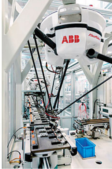
Figure 1.6 – ABB FlexPicker DELTA robot [Cla88; Cla90].
