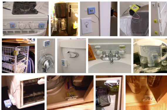
Figure 2.8 – Examples of state-change sensors in one of the 2 homes instrumented for the activity recognition in the home dataset.
