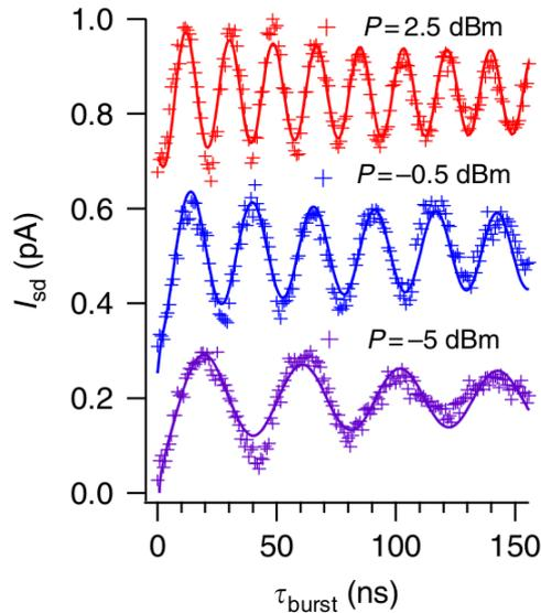
Figure 2.9: Rabi oscillations for different microwave powers. From Ref. [93].
