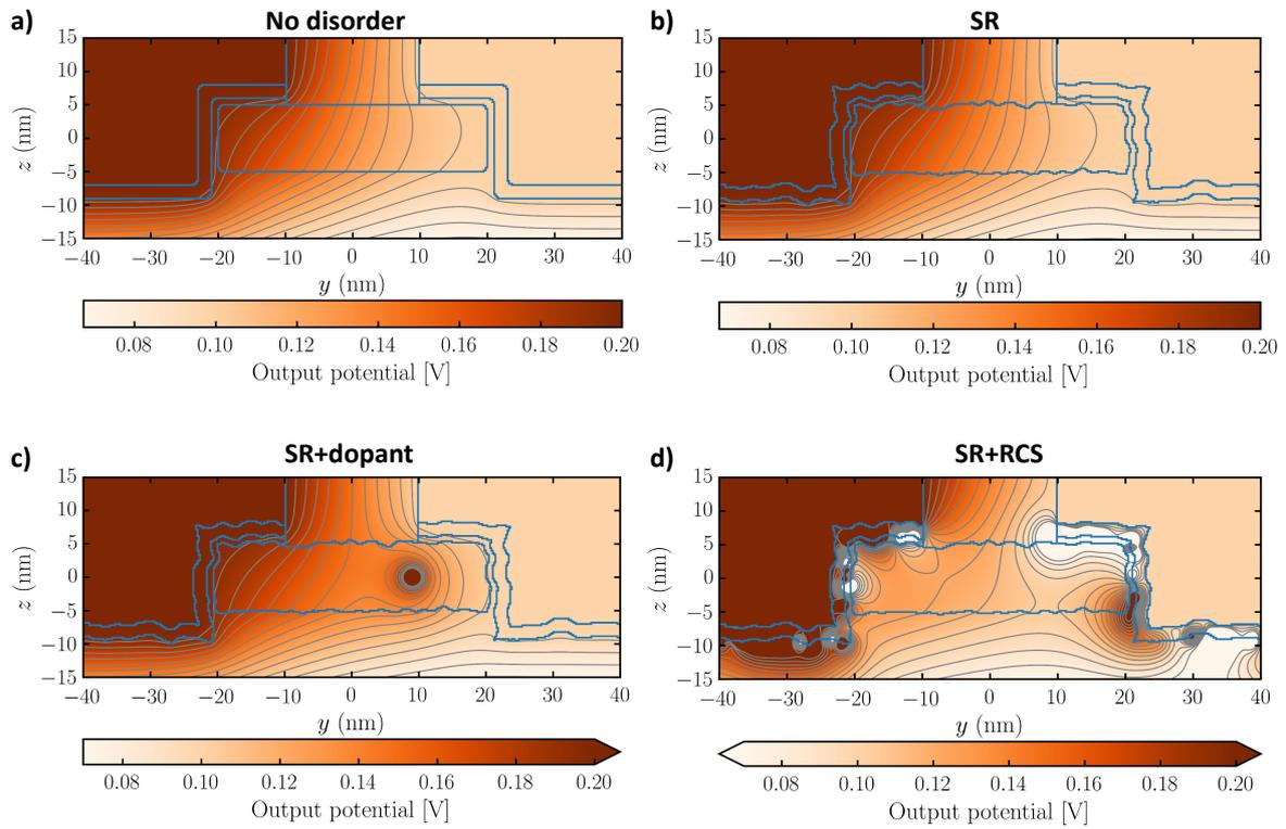
Figure 3.3: Cross-section of the calculated potential in the  $yz$ -plane at  $x = 0$ , for different cases. (a) Perfect device without disorder. (b) Including surface roughness (SR). (c) Including SR and one dopant with charge +1 at  $(x, y, z) = (0, 9, 0)$  nm. The color scale is the same than (a), with open scale. (d) Including SR and positive RCS charges with surface density  $n_{\text{RCS}} = 10^{13} \text{ cm}^{-2}$ . The color scale is the same than (a), with open scale.
