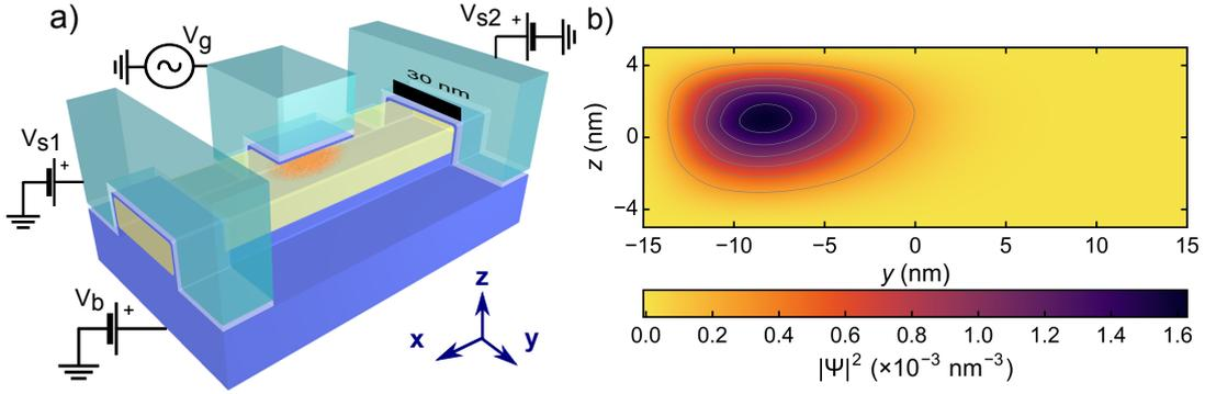
Figure 4.7: (a) Schematics of the device. The silicon nanowire is in yellow, SiO<sub>2</sub> in blue, HfO<sub>2</sub> in light gray and the gate are in dark green. The squared wavefunction is schematized in orange. (b) Cross-section of the squared wavefunction in the (yz) plane, computed with tight-binding.
