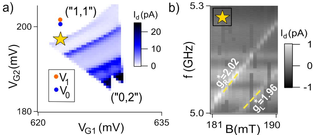
Figure 6.2: (a) Bias triangles of the double dot under study at  $V_d = 5$  mV. Quoted numbers denote the equivalent excess charges deducible from Pauli spin blockade; points  $V_0$ ,  $V_1$  mark where spins are manipulated during pulse sequences. (b) Spectroscopy of the hole qubit under Pauli spin blockade (yellow star in (a)) via  $I_d$  as a function of a continuous microwave frequency  $f$  and  $|\mathbf{B} = (B, 0, 0)|$ . From Ref. [100].
