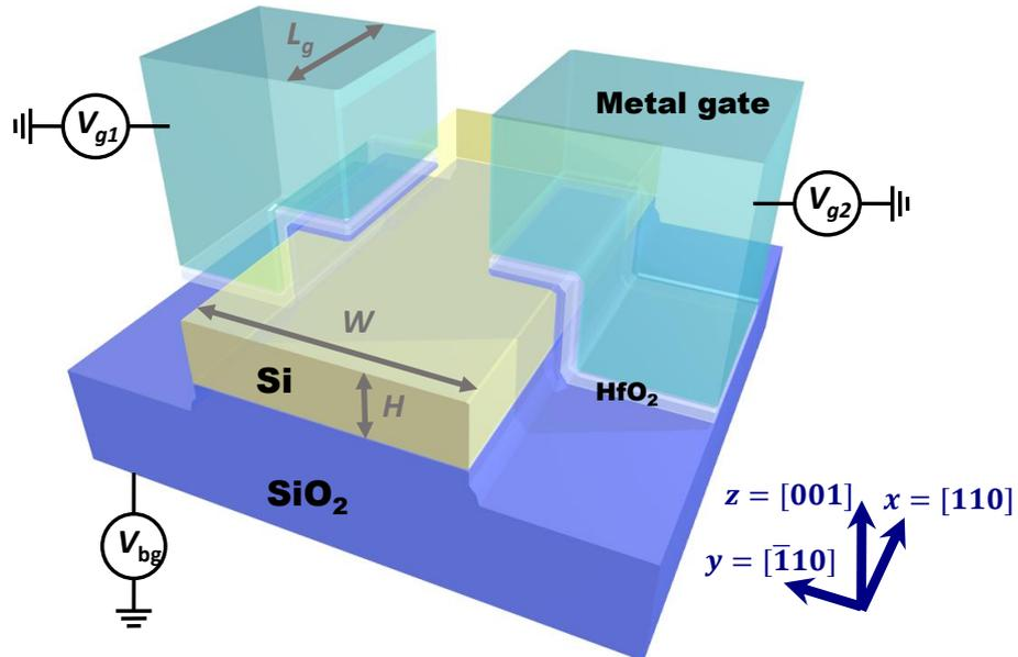
Figure 3.2: Geometry of the "face-to-face" device. The silicon nanowire is in yellow,  $\text{HfO}_2$  is in light gray,  $\text{SiO}_2$  is in dark blue and the metal gates are in light blue. The buried  $\text{SiO}_2$  lies on top of a Si substrate, not shown.
