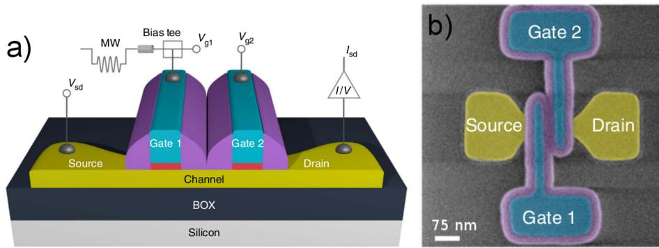
Figure 2.8: (a) 3D schematic of a double quantum dot sample. (b) Top view of the device. From Ref. [93].
