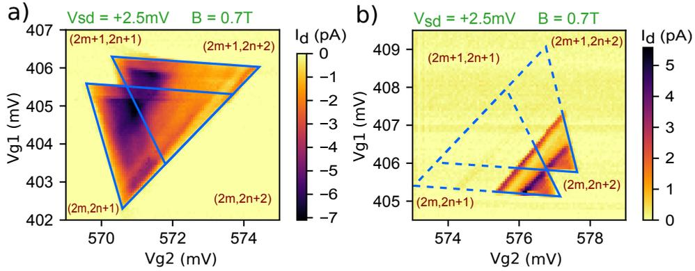
Figure 4.3: Bias triangles. (a) Map of the current  $I_{ds}$  as a function of  $V_{g1}$  and  $V_{g2}$  at finite  $V_{ds} = -2.5 \text{ mV}$  around a pair of triangles showing current rectification. The magnetic field  $B = 0.7 \text{ T}$  is parallel to  $\mathbf{x} - \mathbf{y}$  (see axes on Fig. 4.2). The number of electrons in each dot is given between parentheses. (b) Same as (a) at opposite  $V_{ds} = +2.5 \text{ mV}$ . Adapted from Ref. [53]
