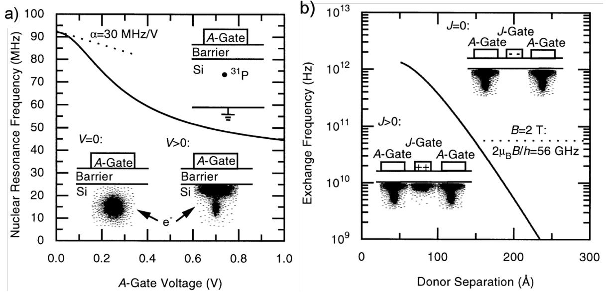
Figure 2.4: Kane quantum computer proposal (a) A-gate, which controls the hyperfine interaction. (b) J-gate, which controls the exchange interaction between two neighboring dots. Both figures are from Ref. [36].
