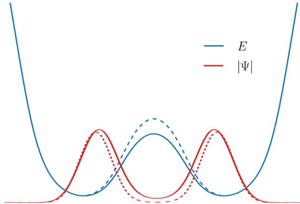
Figure 1.5: Sketch of two qubits coupled by exchange interaction. The height of the barrier between dots tunes  $t$  and thus  $J$ . Dotted lines correspond to the high-barrier regime ( $t \simeq 0$ ) and full lines to the the low-barrier regime (finite  $t$ ).
