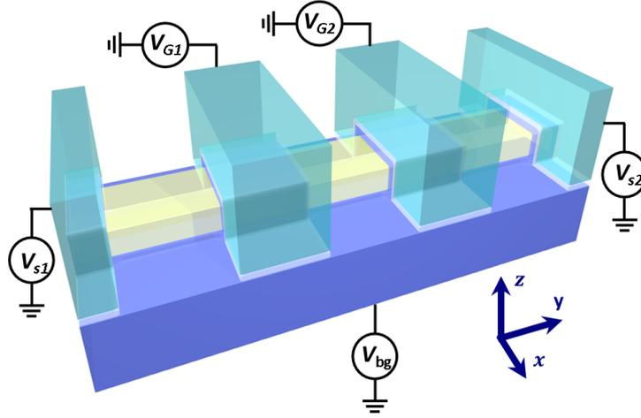
Figure 6.15: Schematic of the device. The silicon nanowire is in yellow,  $\text{SiO}_2$  is in blue,  $\text{HfO}_2$  in light gray and the gates are in dark green.
