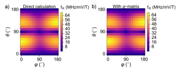
Figure 6.13: (a) Direct calculation of  $f_R$  using Eq. 6.25 (b) Calculation of  $f_R$  using the g-matrix formalism and Eq. 6.13.
