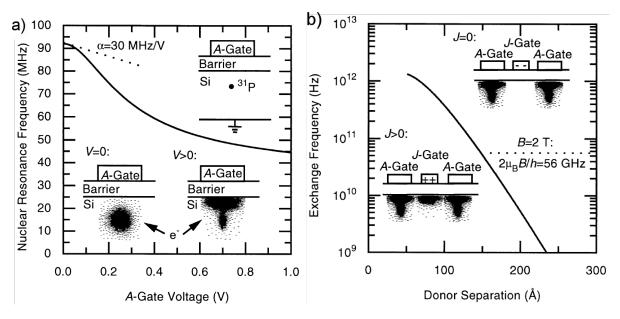
Figure 2.4: Kane quantum computer proposal (a) A-gate, which controls the hyperfine interaction. (b) J-gate, which controls the exchange interaction between two neighboring dots. Both figures are from Ref. [36].
