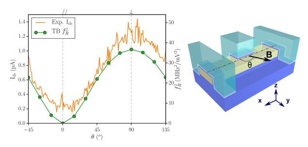
Figure 4.16: Comparison of the dependence with in-plane magnetic orientation of the measured current and of the squared Rabi frequency computed in tight-binding. The directions parallel and perpendicular to the nanowire are highlited with dashed lines. The definition of the angle  $\theta$  is given in the right panel, on the schematic of the device.
