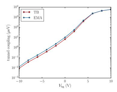
Figure 3.7: Tunnel coupling between the two dots of the face-to-face device as a function of  $V_{\text{bg}}$ , calculated using TB and EMA.
