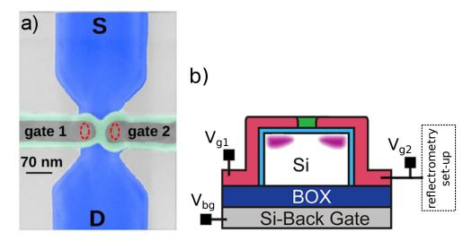
Figure 2.10: (a) Top view of a face-to-face device. The quantum dots approximate locations are shown by red lines. From Ref. [97]. (b) Schematic of the cross-section of the device and set-up. The position of the wavefunctions into the corner states is outlined in pink. Adapted from Ref. [94].
