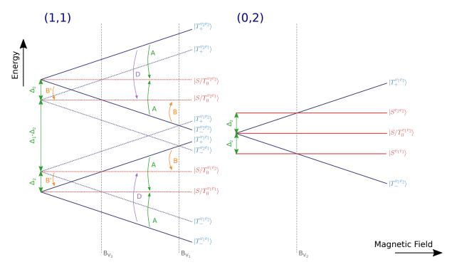
Figure B.1: Scheme of the energy levels for a system with two dots, filled with two electrons in the (1,1) and (0,2) charge configurations, as a function of magnetic field. We assume different valley splittings in the two dots (respectively  $\Delta_1 > \Delta_2$ ). Triplets in the (0,2) configurations with two electrons in the same valley are not represented, since they are energetically far away.
