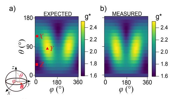
Figure 6.8: (a)  $g^*$  as a function of the field angles  $\theta$  and  $\varphi$ , reconstructed from the six values of  $g^*$  defining the Zeeman tensor. (b) Experimental cartography of  $g^*$ , same as Fig. 6.5b), for comparison. From Ref. [100].
