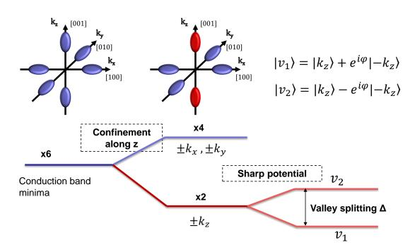
Figure 2.3: Schematic of the effect of the confinement and potential on the valley states and their degeneracy.
