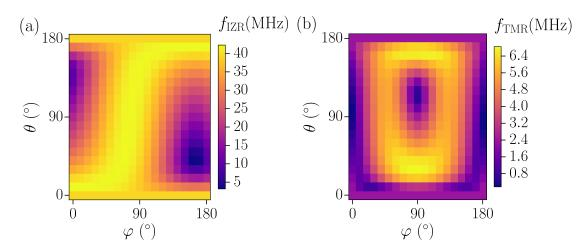
Figure 6.19: Rabi frequency cartography for a state located under between the two gates, at constant Zeeman energy (9 GHz), with tensile in-plane strain, with surface roughness and RCS charges with density  $n_{\rm RCS} = 2 \times 10^{12}$  cm<sup>-2</sup>. (a) IZ-EDSR contribution (b) g-TMR contribution.
