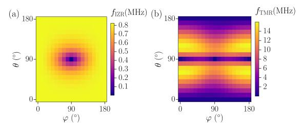
Figure 6.16: Rabi frequency cartography for a state located under the main gate, at constant Zeeman energy (9 GHz) (a) IZ-EDSR contribution (b) g-TMR contribution.
