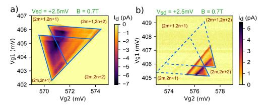
Figure 4.3: Bias triangles. (a) Map of the current  $I_{ds}$  as a function of  $V_{g1}$  and  $V_{g2}$  at finite  $V_{ds} = -2.5$  mV around a pair of triangles showing current rectification. The magnetic field B = 0.7 T is parallel to  $\mathbf{x} - \mathbf{y}$  (see axes on Fig. 4.2). The number of electrons in each dot is given between parentheses. (b) Same as (a) at opposite  $V_{ds} = +2.5$  mV. Adapted from Ref. [53]
