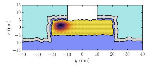
Figure 3.5: Cross-section of the squared TB wavefunction of an electron in the yz-plane at x=0, calculated with the potential of Fig. 3.3b. The iso-probability surfaces are in gray. The Si atoms are the black dots, and the same colors have been used for the other materials as in Fig. 3.2.
