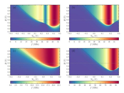
Figure 5.11: Map of the Rabi frequency as a function of the magnetic field and  $V_{\text{bg}}$ , for different realizations of the disorder. The dotted black line is the anti-crossing condition  $E_Z = g\mu_B B = \Delta(V_{\text{bg}})$ . The horizontal dashed line is a target magnetic field B = 0.5 T for qubit operation.  $V_g = 0.1$  V and  $\mathbf{B} \parallel y$  in all plots.
