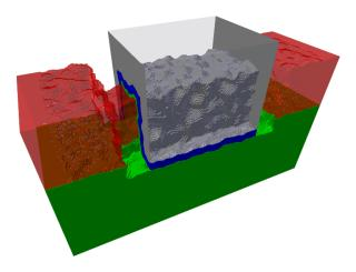
Figure 2.6: 3D schematic of a typical trigate silicon MOSFET from Leti. Silicon is in red,  $SiO_2$  in green,  $HfO_2$  in blue, and the metallic gate is in gray.
