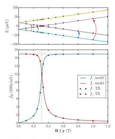
Figure 4.11: Energy levels and  $f_-$  and  $f_+$  Rabi frequencies, corresponding to transitions between the ground state and respectively  $|\Psi'_-\rangle$  and  $|\Psi'_+\rangle$ , as highlighted by the blue  $(f_-)$  and red  $(f_+)$  arrows. Dots are for direct tight-binding calculations, the solid lines are for the analytical model with  $C_{v_1v_2}=1.8$ ,  $D_{v_1v_2}=70~\mu\text{eV/V}$  and  $\Delta=36~\mu\text{eV}$ , extracted from the TB calculations.
