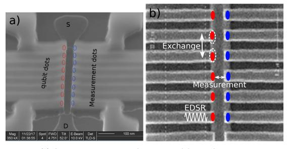
Figure 2.11: (a) SEM tilted top view of an array of face-to-face devices on a single nanowire. Schematics of the dots approximate position are given in red for the qubit dots and in blue for the measurement dots. (b) SEM top view with same color code. The possible operations (spin measurement, single spin control via EDSR, and exchange interaction) are outlined in white.
