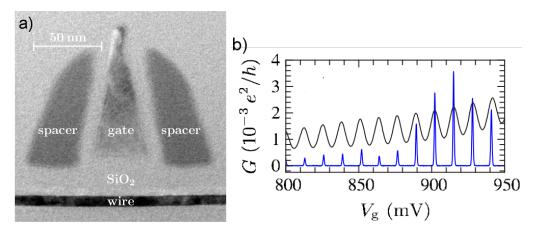
Figure 2.7: (a) MOSFET transistor with long spacers, isolating a quantum dot under the gate, capacitively coupled to the source and drain contacts. (b) Measured Coulomb oscillations at 4.2 K (black curve), and at 400 mK (blue curve). Adapted from Ref. [90].
