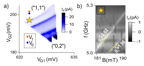
Figure 6.2: (a) Bias triangles of the double dot under study at  $V_d = 5$  mV. Quoted numbers denote the equivalent excess charges deducible from Pauli spin blockade; points  $V_0$ ,  $V_1$  mark where spins are manipulated during pulse sequences. (b) Spectroscopy of the hole qubit under Pauli spin blockade (yellow star in (a)) via  $I_d$  as a function of a continuous microwave frequency f and  $|\mathbf{B} = (B, 0, 0)|$ . From Ref. [100].
