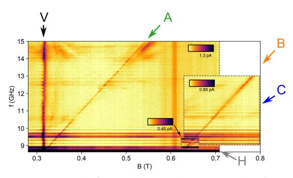
Figure 4.4: Experimental EDSR map. The measured current is plotted as a function of the frequency of the microwave signal and of the magnetic field amplitude. The relevant lines are labelled A, B, C, V, H. Adapted from Ref. [53].
