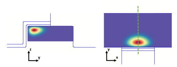
Figure 4.14: Symmetry plane in half-gated device. The mirror planes of the wavefunction are given by the dotted green lines.
