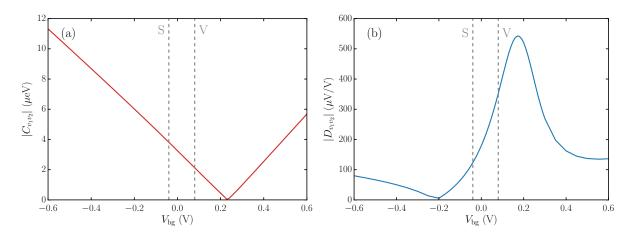
Figure 5.5: (a) Spin-orbit and (b) dipolar inter-valley matrix elements as a function of  $V_{\text{bg}}$ . The gray dashed lines highlight the spin and valley mode arbitrarily chosen for the qubit operation.
