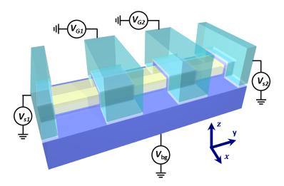
Figure 6.15: Schematic of the device. The silicon nanowire is in yellow,  $SiO_2$  is in blue,  $HfO_2$  in light gray and the gates are in dark green.
