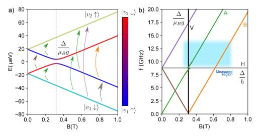
Figure 4.6: (a) Energy diagram of the first four states as a function of the magnetic field amplitude. An avoided crossing is supposed at  $B = \Delta/(g\mu_B)$ . The energy of  $|v_1\downarrow\rangle$  is in light blue, and the energy of  $|v_2\uparrow\rangle$  is in green. The spin and valley composition of the hybridized states is quantified by a colour scale. (b) Sketch of the possible transitions noted by the arrows in (a). The experimentally measured region is in light blue.
