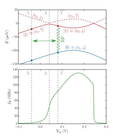
Figure 5.4: (Top panel) Energy levels as a function of  $V_{\rm bg}$ . The gray dashed lines highlight the spin (S) and valley (V) mode chosen for the qubit operation and the avoided crossing (A) separating the two regimes. (Bottom panel) Rabi frequency corresponding to the transition  $|0\rangle \leftrightarrow |1\rangle$  as a function of  $V_{\rm bg}$ .
