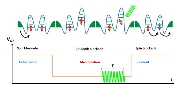
Figure 6.3: Protocol for manipulation and detection of the spin. Adapted from Ref. [93].
