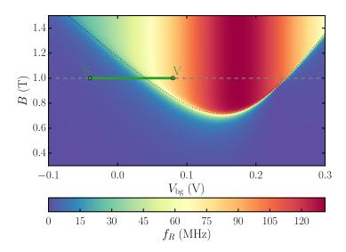
Figure 5.3: Map of Rabi frequency as a function of the magnetic field amplitude and  $V_{\text{bg}}$ . The dotted black line is the anticrossing condition  $E_z = g\mu_B B = \Delta(V_{\text{bg}})$ . The RF amplitude is  $V_{ac} = 1$  mV. The green line is the path chosen for qubit operation at B = 1 T.
