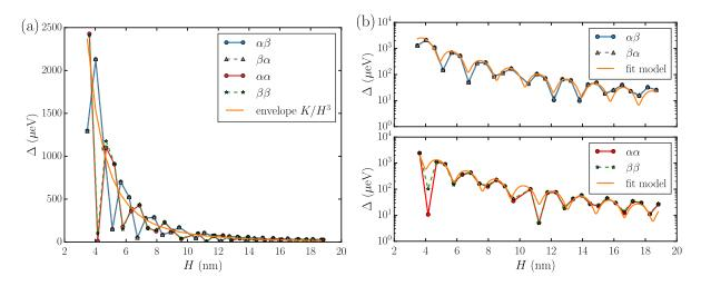
Figure 5.13: Valley splitting as function of the wire thickness H, for four sets of surface termination. The hydrogen bondings of top and bottom surfaces are either parallel (AA or BB) or orthogonal (AB or BA). (a) Linear scale, we fit the envelope from the model of Eq. 5.31. (b) Semilog scale, we fit the full model from Eq. 5.32 for orthogonal surface bondings (top panel) and parallel surface bondings (bottom panel).
