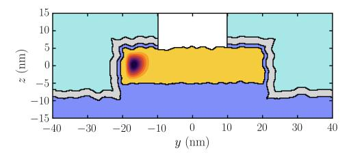
Figure 3.6: Iso-surfaces of the squared wavefunction of a hole obtained from 6-bands  $\mathbf{k}.\mathbf{p}$  in the yz-plane at x=0. The same colors have been used for the materials as in Fig. 3.2.
