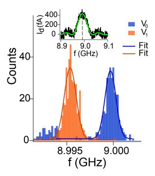
Figure 6.6: Inset: current trace as a function of microwave frequency f for burst duration  $\tau = 20 \,\text{ns}$  at  $\mathbf{B} = (0, 216, 216) \,\text{mT}$ . Blue and orange histograms display the dispersion of the resonance frequency when  $V_{G2}$  is pulsed to point  $V_0$  and  $V_1$ , respectively. The Gaussian fits yield  $g^*(V_0) = 2.013 \pm 0.001$  and  $g^*(V_1) = 2.010 \pm 0.001$ , taking into account the field uncertainty. From Ref. [100].
