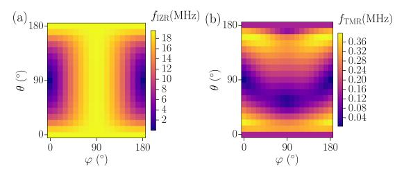
Figure 6.18: Rabi frequency cartography for a state located under between the two gates, at constant Zeeman energy (9 GHz), with tensile in-plane strain, without disorder. (a) IZ-EDSR contribution (b) g-TMR contribution.
