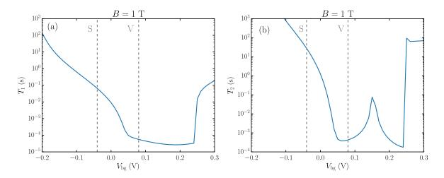
Figure 5.9: (a) Relaxation time including phonons and Johnson-Nyquist noises as a function of  $V_{\rm bg}$  (b) Dephasing time for Johnson-Nyquist noise  $T_{2,\rm jn}^*$  as a function of  $V_{\rm bg}$ . For both panels B=1 T, and the vertical gray dotted lines mark the spin and valley operation points of part 5.2.
