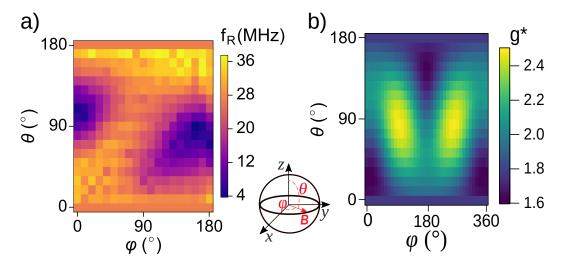
Figure 6.5: (a) Cartography the angular dependence of the Rabi frequency. The measurement is performed at constant Zeeman splitting (9 GHz). (b) Measured  $g^*$  carthography.  $\theta, \varphi$  are stepped by 10° between 0° and 180°. The whole plot can be obtained by symmetry  $(\mathbf{B} \to -\mathbf{B})$ .
