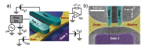
Figure 4.2: (a) Sketch of the sample and measurement setup. The silicon nanowire is coloured in yellow, the two top gates in green and the side gate in violet. The gate oxides are colored in orange and the buried oxide (BOX) is in blue. (b) Colourized device top view obtained by scanning electron microscopy before the deposition of the spacers of a device similar to the one used in the experiment, with same colour code. Adapted from Ref. [53]
