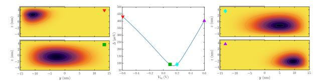
Figure 5.2: (Central panel) valley splitting as a function of backgate potential ( $V_g = 0.1$  V). The valley splitting shows a minimum  $\Delta^{\min} = 83 \ \mu\text{eV}$  at  $V_{\text{bg}}^{\min} = 0.15$  V. (Lateral panels) The squared wavefunction of the ground state  $|0\rangle$  is plotted in the (yz) cross section, at the four bias points labelled by the symbols. The thick gray lines outline the position of the front gate.
