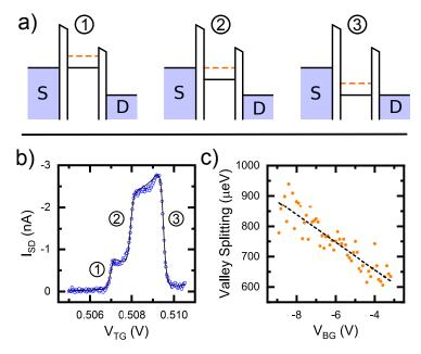
Figure 5.16: (a) Diagrams illustrating the respective alignment of the quantum dot and source and drain electrochemical levels at the three features observed in b). (b) Measured source-drain current (blue dots) in the first Coulomb oscillations at  $V_{BG}=-7.8~V$ . The black line is a fit considering that the system is in the sequential multi-level transport regime [43]. (c) Plot of valley splitting against  $V_{BG}$  with a best-fit line gradient of  $-45\pm3~\mu eV/V$ . From Ref. [57] .
