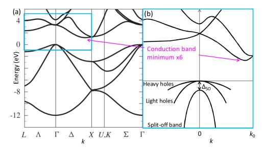
Figure 2.1: (a) Band structure of bulk silicon. (b) Zoom on the conduction band minimum and valence band maximum. From Ref. [43].
