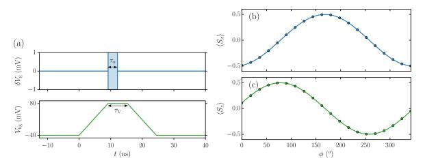
Figure 5.8: (a) Time series for a  $\pi/2$  rotation from the  $|v_1\downarrow\rangle$  state (b,c) Expectation value of  $S_x$  and  $S_z$  in the rotating Bloch sphere after that  $\pi/2$  rotation as a function of the phase  $\phi$  of the driving RF signal.
