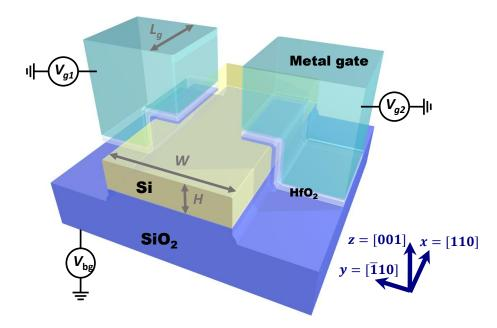
Figure 3.2: Geometry of the "face-to-face" device. The silicon nanowire is in yellow,  $HfO_2$  is in light gray,  $SiO_2$  is in dark blue and the metal gates are in light blue. The buried  $SiO_2$  lies on top of a Si substrate, not shown.
