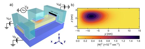
Figure 4.7: (a) Schematics of the device. The silicon nanowire is in yellow,  $SiO_2$  in blue,  $HfO_2$  in light gray and the gate are in dark green. The squared wavefunction is schematized in orange. (b) Cross-section of the squared wavefunction in the (yz) plane, computed with tight-binding.
