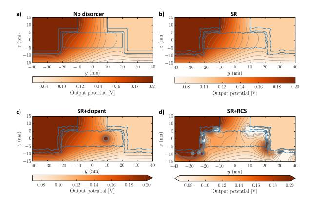
Figure 3.3: Cross-section of the calculated potential in the yz-plane at x=0, for different cases. (a) Perfect device without disorder. (b) Including surface roughness (SR). (c) Including SR and one dopant with charge +1 at (x,y,z)=(0,9,0) nm. The color scale is the same than (a), with open scale. (d) Including SR and positive RCS charges with surface density  $n_{\rm RCS}=10^{13}~{\rm cm}^{-2}$ . The color scale is the same than (a), with open scale.
