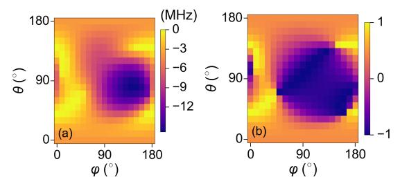
Figure 6.12: (a) Map of  $|\mathbf{f}_R| - |\mathbf{f}_{IZR}| - |\mathbf{f}_{TMR}|$  as a function of the orientation of the magnetic field. (b) Map of  $\cos(\theta_Z)$  as a function of the orientation of the magnetic field, where  $\theta_Z$  is the angle between  $\mathbf{f}_{IZR}$  and  $\mathbf{f}_{TMR}$ .
