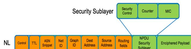
Figure 3.5: WirelessHART NPDU structure
