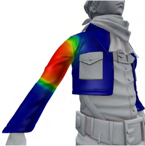
Figure 1.9: Weight painting in Blender, showing the influence of the arm bone over the jacket vertices from w_{ij} = 1 in red (maximal influence) to w_{ij} = 0 in blue (no influence).
