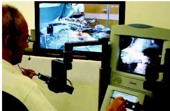
Figure 4.1 - Teleoperated surgery using Zeus system, demonstrated by Dr. Jacques Marescaux in New York on the patient in Strasbourg, France. Source: (Marescaux et al., 2001).
