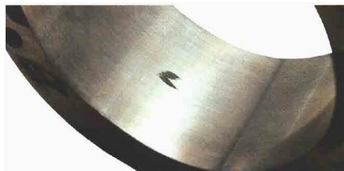
Figure 4.8 Aeration damage: black mark on cam ring due to air bubble implosion, from [2]
