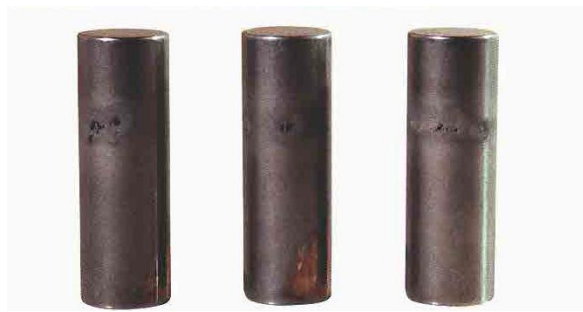
Figure 4.5 Cavitation erosion: craters on pins, from [2]
