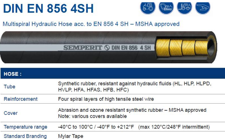
Figure B.3 Flexible Hoses: Semperit DIN 31 EN 856 4SH, from [17]
