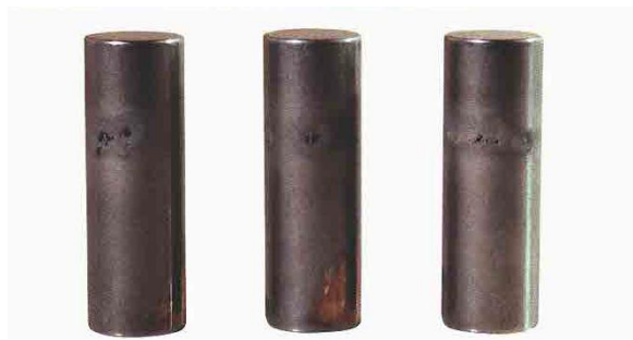
Figure 4.5 Cavitation erosion: craters on pins, from [2]
