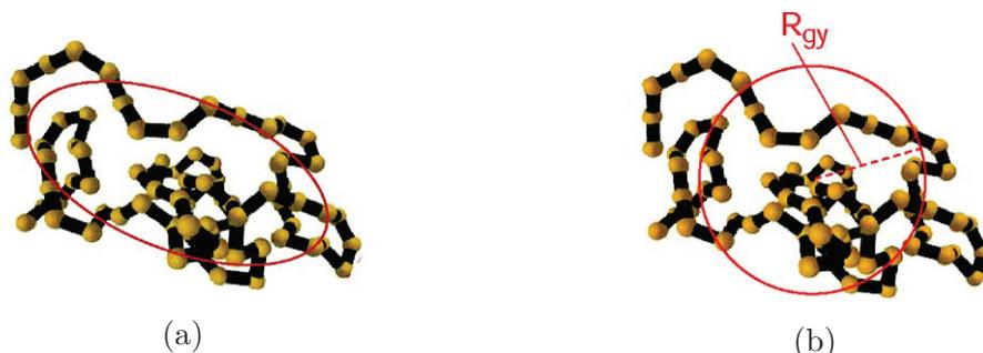
Figure 4.12: Schematic of the contour of a disordered polymer chain measured by (a) gyration tensor and (b) radius of gyration [95].
