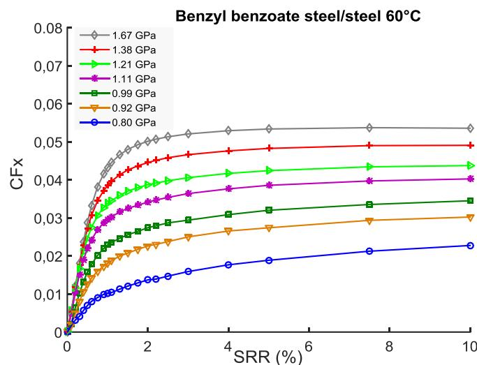
Figure II-13: Friction coefficient versus SRR,  $U_e=5\text{m/s}$ .
