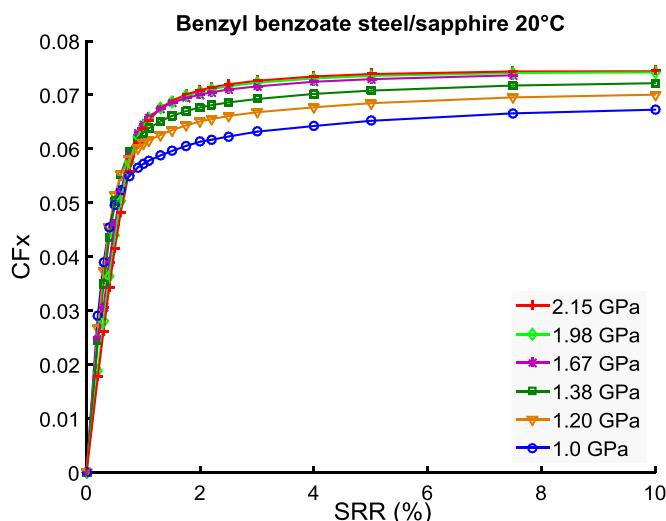
*Figure II-8: Friction coefficient versus SRR,  $U_e=1.3\text{m/s}$ .*
