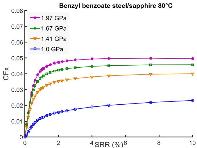
Figure II-15: Friction coefficient versus SRR,  $U_e=6.5\text{m/s}$ .
