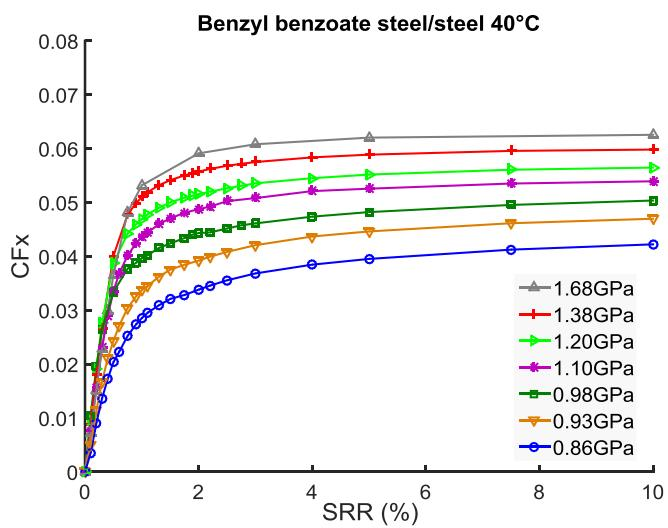
Figure II-10: Friction coefficient versus SRR,  $U_e=2.5\text{m/s}$ .
