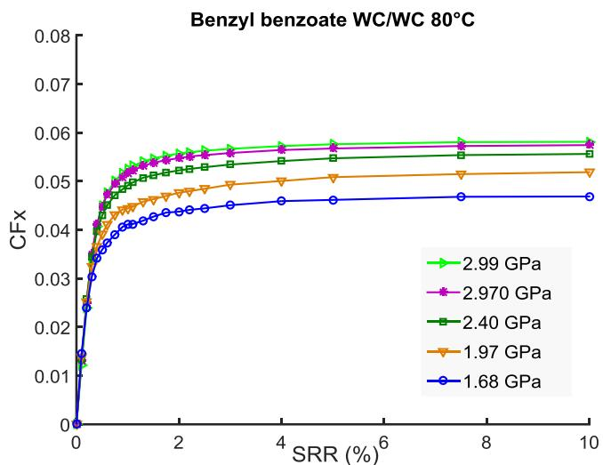
Figure II-16: Friction coefficient versus SRR,  $U_e=6.5\text{m/s}$ .
