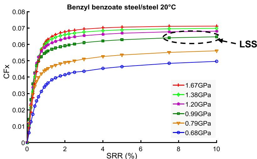
*Figure II-7: Friction coefficient versus SRR,  $U_e=1.3\text{m/s}$ .*
