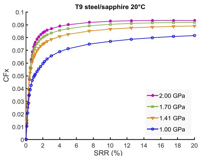
Figure II-19: Friction coefficient versus SRR,  $U_e=0.5\text{m/s}$ .
