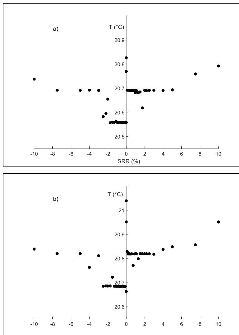
Figure II-4: Inlet temperature variations during friction measurements with benzyl benzoate at  $T=20^{\circ}\text{C}$  and  $U_e=1.3 \text{ m/s}$  in:
