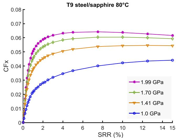
Figure II-25: Friction coefficient versus SRR,  $U_e=6.5\text{m/s}$ .
