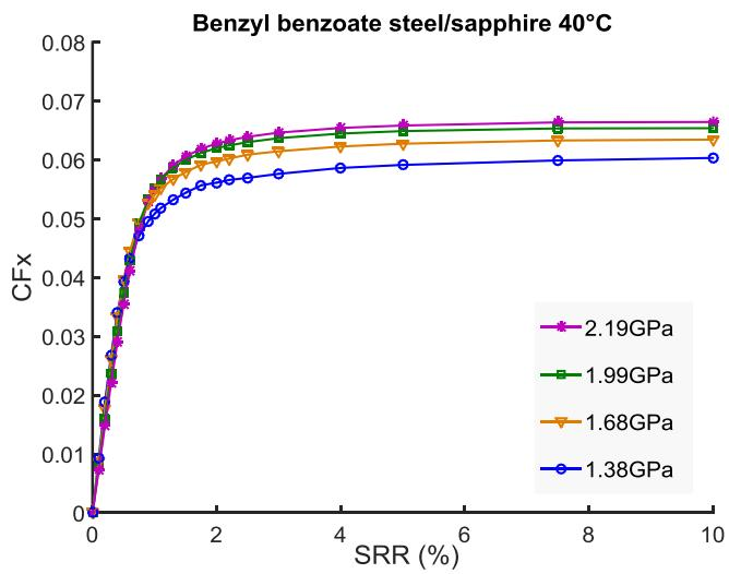
Figure II-11: Friction coefficient versus SRR,  $U_e=2.5\text{m/s}$ .
