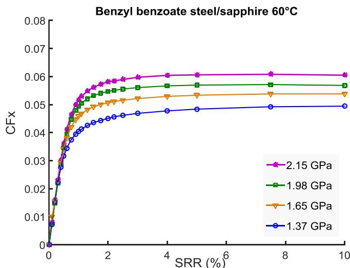
Figure II-14: Friction coefficient versus SRR,  $U_e=5\text{m/s}$ .
