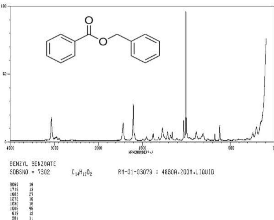
Figure III-8: Schematic structure of the benzyl benzoate molecule, of formula  $C_{14}H_{12}O_2$ , and its Raman spectrum (SDBS Web: <http://sdbbs.db.aist.go.jp> (National Institute of Advanced Industrial Science and Technology, date of access) (SDBS No.:7302).
