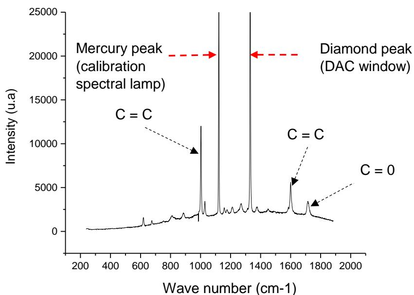
Figure III-10: Raman spectrum of benzyl benzoate at  $20^\circ\text{C}$  and  $P_{\text{atm}}$  (u.a stands for arbitrary units).
