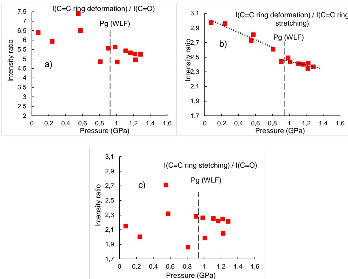
Figure III-15 : Intensity ratio variations of benzyl benzoate with pressure at 40°C.
