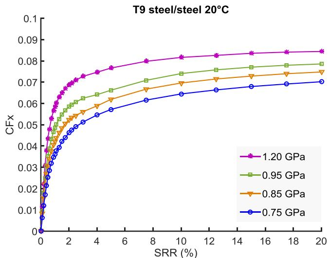
Figure II-18: Friction coefficient versus SRR,  $U_e=0.5m/s$ .
