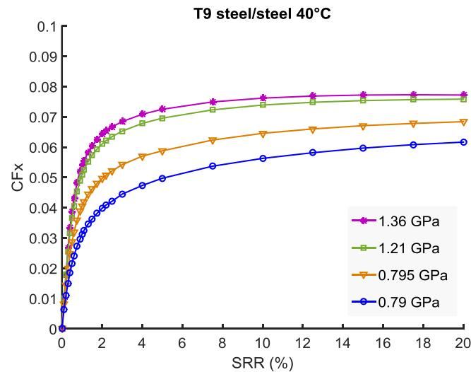
Figure II-21: Friction coefficient versus SRR,  $U_e=1.3\text{m/s}$ .
