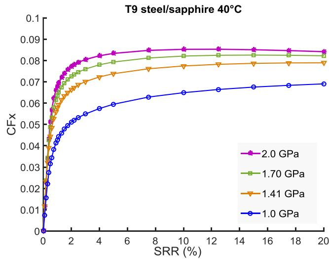
Figure II-22: Friction coefficient versus SRR,  $U_e=1.3\text{m/s}$ .
