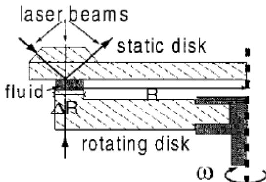
Figure I-8: Schematic of half of the flow cell used by Pit et al. [18].
