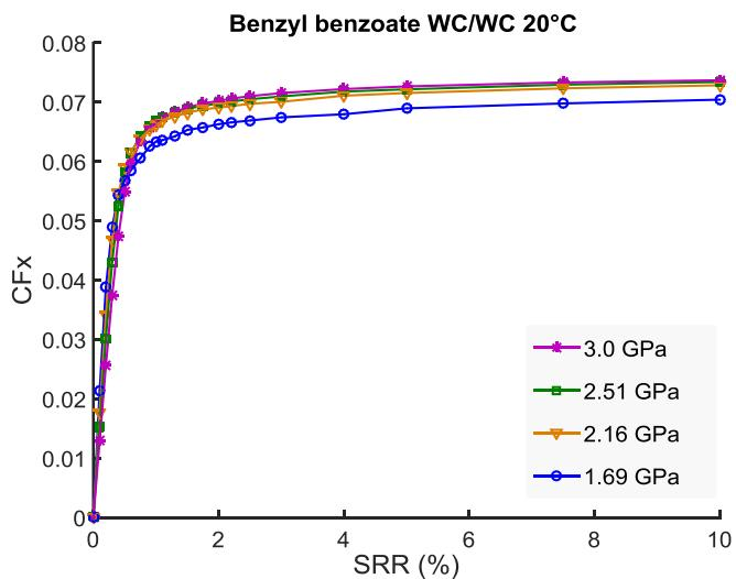
Figure II-9: Friction coefficient versus SRR,  $U_e=1.3\text{m/s}$ .
