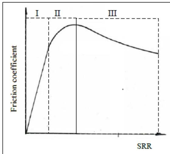
Figure I-5: Friction regimes according to Dyson [62].
