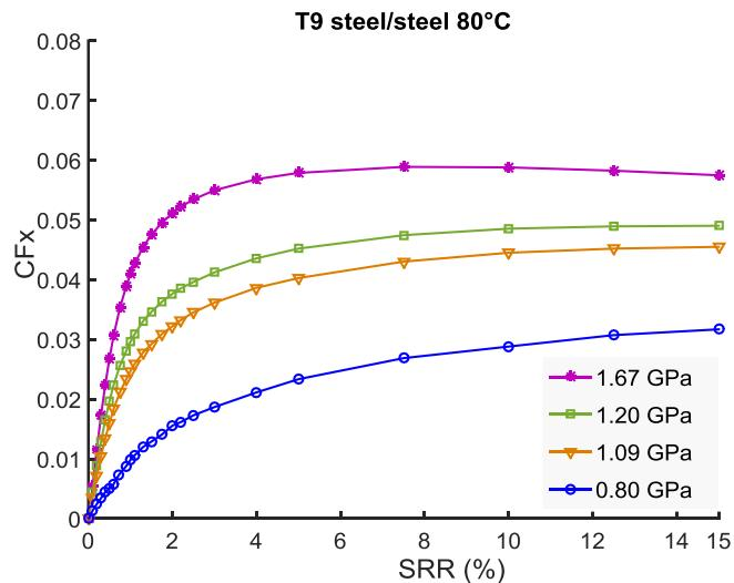
Figure II-24: Friction coefficient versus SRR,  $U_e=6.5\text{m/s}$ .
