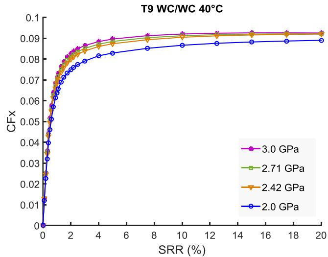
Figure II-23: Friction coefficient versus SRR,  $U_e=1.3\text{m/s}$ .
