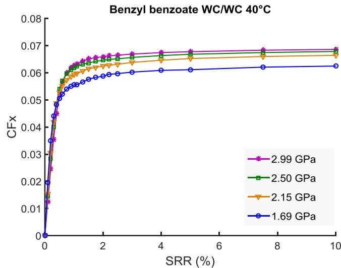
Figure II-12: Friction coefficient versus SRR,  $U_e=2.5\text{m/s}$ .
