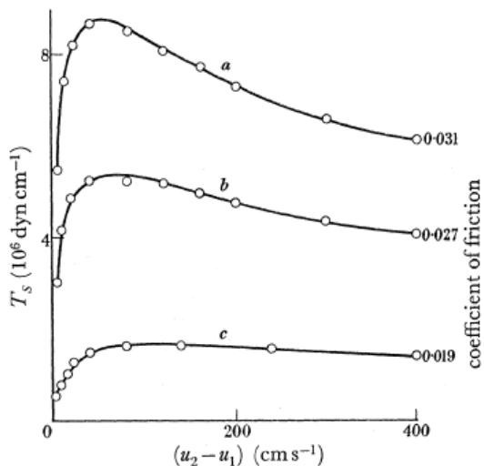
Figure I-4: Friction as function of sliding speed; (rolling speed at  $400 \text{ cm}^{-1}$ ). Load ( $10^7 \text{ dyn cm}^{-1}$ ): (a) 20, (b) 15, (c) 7.5 from [57].
