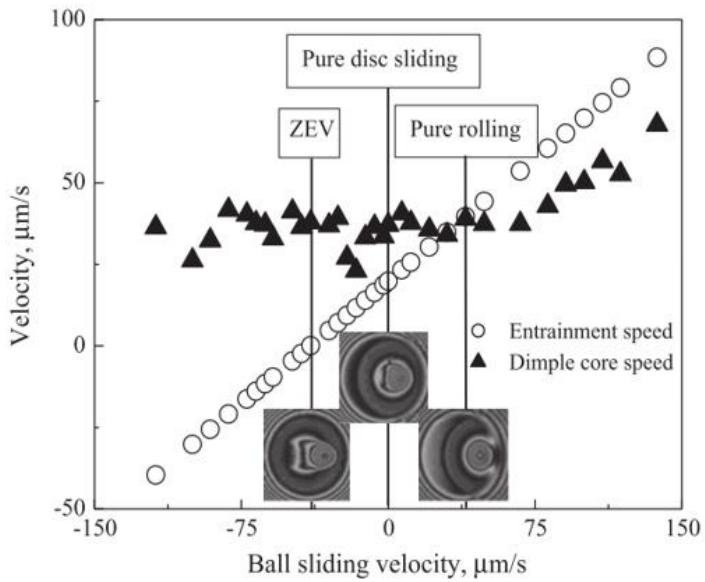
*Figure I-7: Dimple velocity under various ball velocities for a constant disc velocity (PB1300 steel/SiO<sub>2</sub>,  $ud=+39.6\mu\text{m/s}$ , 20N) from Wong et al.[71].*
