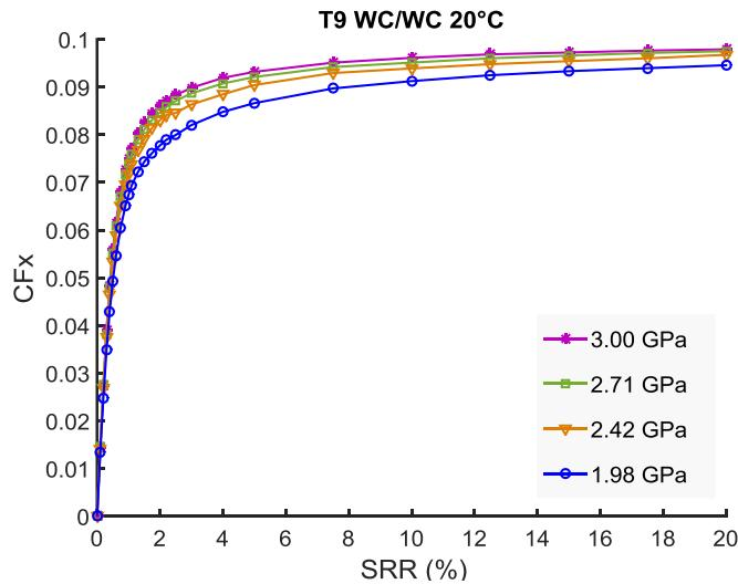
Figure II-20: Friction coefficient versus SRR,  $U_e=0.5\text{m/s}$ .
