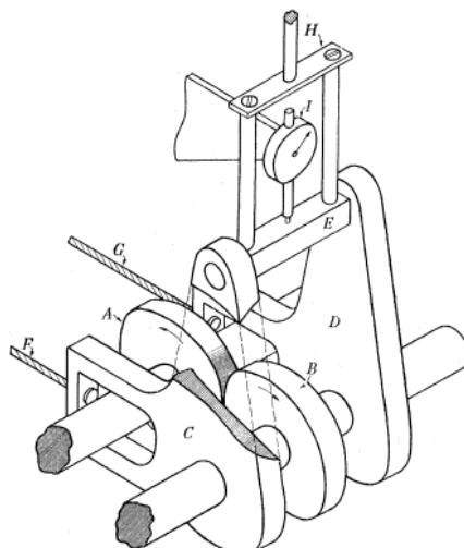
*Figure I-2: The two disc machine arranged for the measurement of friction from Crook [57]. A and B discs; C and D swinging arms; E axle; F and G loading cables. H spring beam; I dial gauge.*
