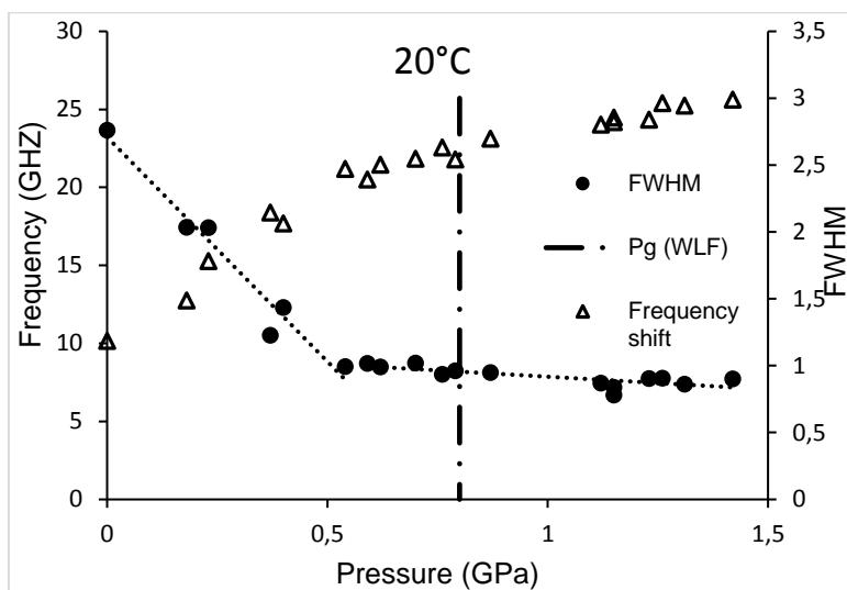
Figure III-18: Brillouin spectroscopy results obtained at 20°C.
