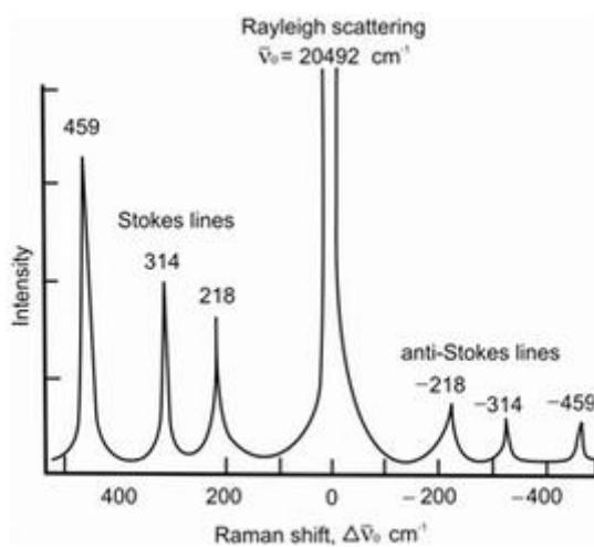
Figure III-7: Example of a Raman spectrum (CCl<sub>4</sub>, 488 nm excitation)
