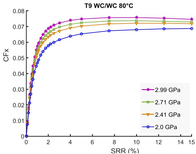
Figure II-26: Friction coefficient versus SRR,  $U_e=6.5\text{m/s}$ .
