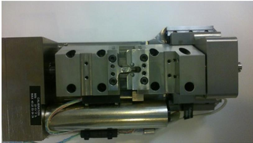
Figure 2.13: A set up allowing to perform 3PB in SEM
