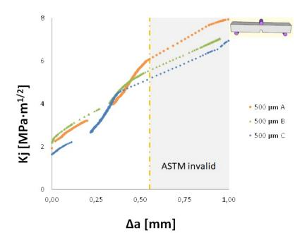
Figure 5.55: R-curves of the material with  $500\mu$ m foil
