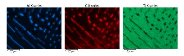
Figure 5.19: Chemical analysis of intermetallics
