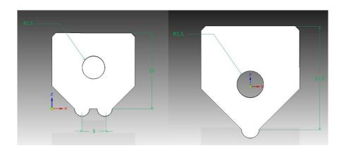
Figure 2.11: Upper parts of three and four point bending set up
