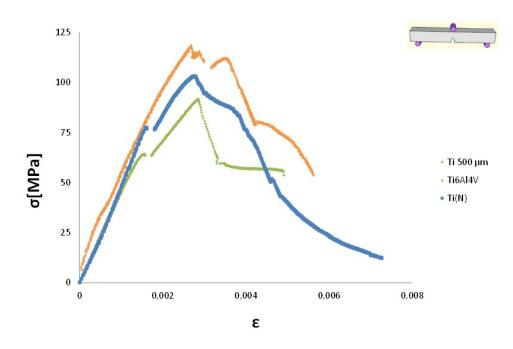
Figure 5.63: Comparison of Stress-Strain curves of materials with different foil chemistry (500  $\mu$ m thick metal layers)
