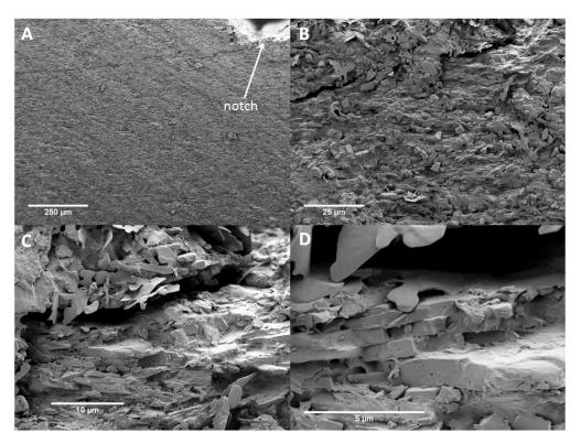
Figure 4.22: SEM images of crack in the sample with graphene in the interphase. A) A white arrow indicates the tip of the notch and beginning of crack which propagates visibly on one side; B) Same zone of the sample with higher magnification; C) A zone where crack has changed its path (from horizontal in the middle of the image to vertical on the left); D) Zone where some flaky structures are visible on the surface of some alumina platelets
