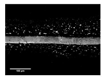
Figure 5.13: A sample sintered at 1500 °C with 30 minutes holding time at 1500 °C; significant diffusion of titanium (BSE detector)
