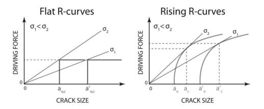
Figure 1.3: Schematic illustrations of crack-resistance curves (R-curves) [3]
