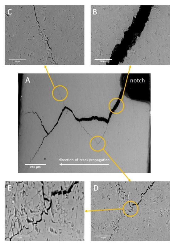
Figure 5.44: SEM pictures of the broken reference sample during three point bending in situ
