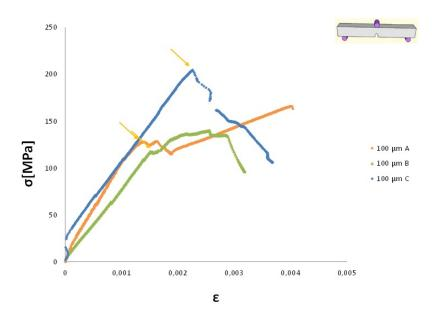
Figure 5.51: Stress-Strain curves of the material with  $100\mu$ m foil
