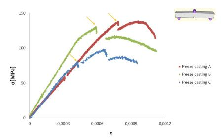
Figure 3.5: Stress-Strain curve of the material processed by freeze casting
