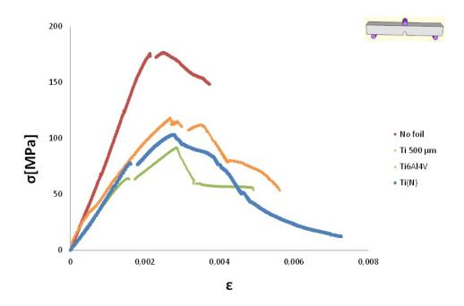
Figure 5.69: Comparison of Stress-Strain curves of materials with different foil chemistry with reference material
