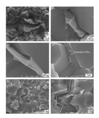
Figure 4.17: Toughening mechanisms in GPL alumina composite [22]
