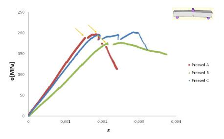
Figure 3.9: Stress-Strain curve of the material processed by uniaxial pressing
