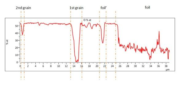
Figure 5.29: Linear analysis of oxygen along the line shown in fig. 5.25
