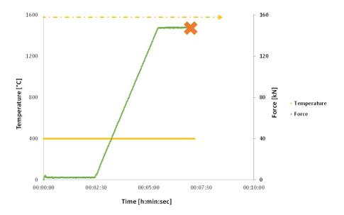
Figure 3.11: Sintering cycle for the first attempt of up-scaling material fabrication, 90 g sample
