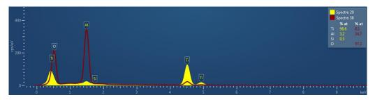
Figure 5.33: Comparison between spectres of metal and intermetallic. Y-axis: number of X-rays received and processed by the detector [cps/eV], X-axis: energy level of those counts [keV].
