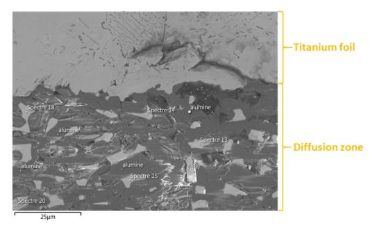
Figure 5.21: Analysis of ceramic matrix and metal grains composition (BSE detector)
