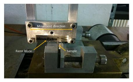
Figure 2.5: A notch sharpening set up
