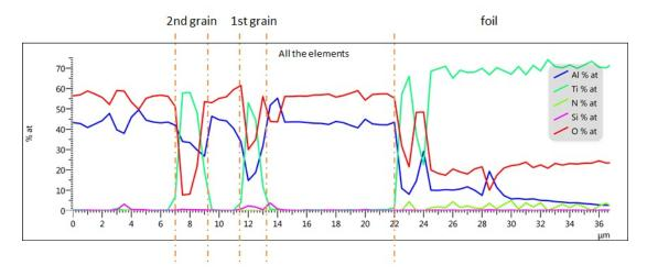
Figure 5.36: Linear analysis of all elements present in the composite along the line shown in fig. 5.35
