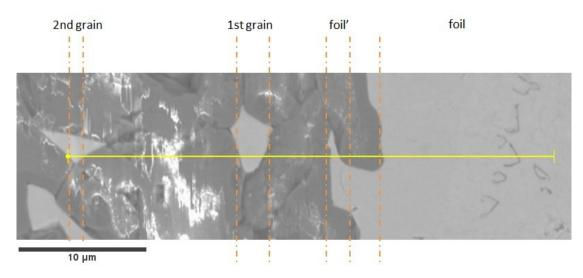
Figure 5.25: Analysis of linear composition of diffusion zone
