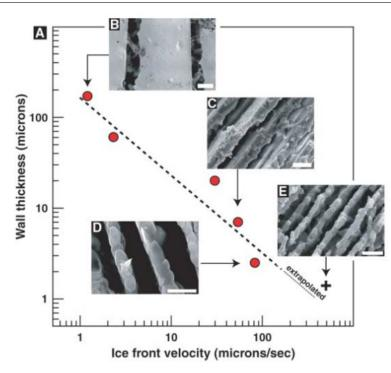
Figure 1.13: (A) Thickness of the lamellae in alumina samples as a function of the speed of the solidification front. The scanning electron micrographs shown in the graph correspond to cross sections parallel to the direction of movement of the ice front. Sample (E) was obtained with ultrafast freezing to gauge the thickness limit achievable by this technique. Scale bars indicate (B) 50 mm, (C) 10 mm, (D) 5 mm, (E) 5 mm. [26]
