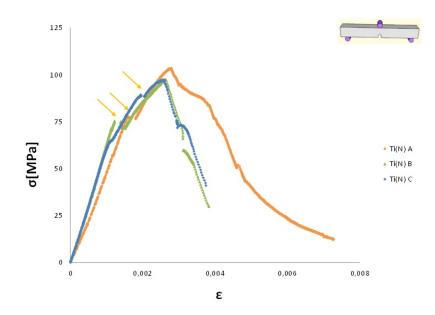
Figure 5.61: Stress-Strain curves of the material with Ti foil with TiN layer (around  $500\mu$ m thick)
