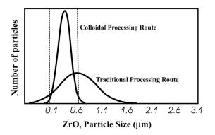
Figure 4.10: Zirconia grain size distribution depending on processing route [20]
