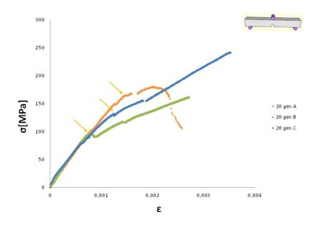
Figure 5.48: Stress-Strain curves of the material with  $20\mu$ m foil
