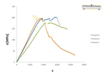
Figure 5.42: Stress-Strain curves of the reference material
