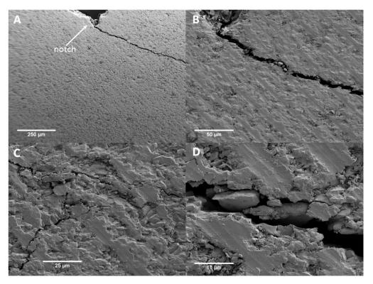
Figure 4.14: SEM images of crack in the sample with platelets processed by alkoxide reaction. A) A white arrow indicates the tip of the notch and beginning of crack which propagates visibly on one side; B) Same zone of the sample with higher magnification; C) Crack branching; D) Zone where some platelets probably have been pulled out, it looks like crack had passed from their both sides
