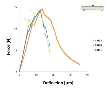
Figure 5.60: Force-Deflection curves of the material with Ti foil with TiN layer (around  $500\mu m$  thick)
