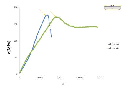
Figure 4.12: Stress-Strain curve of the material with platelets processed by alkoxide reaction
