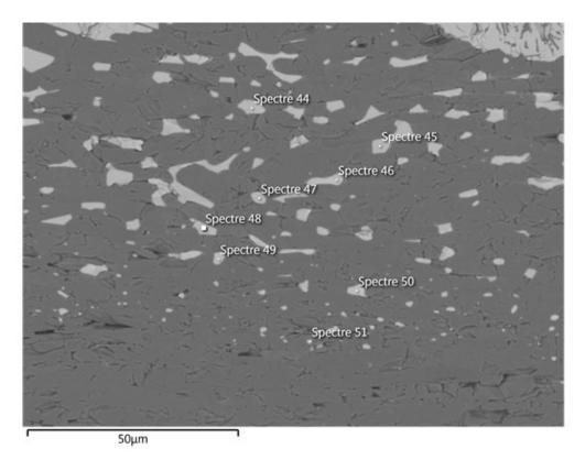
Figure 5.34: Analysis of grain composition in the diffusion zone. Sample with Ti(N) foil, sintered at 1500°C, heating rate 100°C/min, cooling rate 10°C/min.
