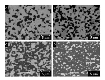
Figure 1.27: SEM pictures of alumina/titanium composites fabricated by FAST [17]. Content of titanium (light gray) in wt% is as follows: A) 80, B) 60, C) 40 and D) 20.
