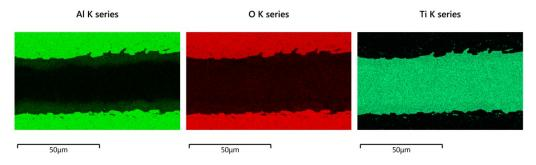
Figure 5.3: Placement of the three elements found during EDX
