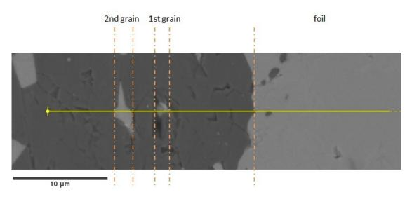
Figure 5.35: Analysis of linear composition of diffusion zone
