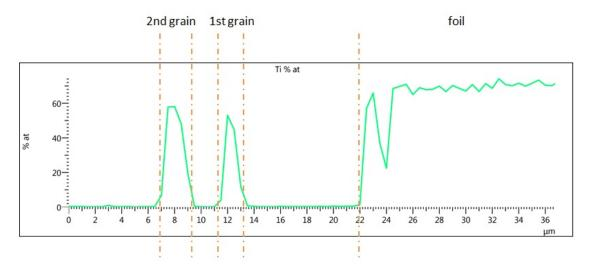
Figure 5.37: Linear analysis of titanium along the line shown in fig. 5.35
