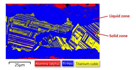
Figure 5.65: Microstructural difference between the zone which was solid and the zone that was probably liquid during sintering
