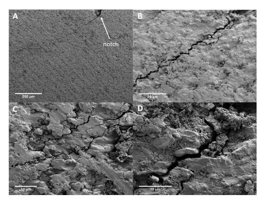
Figure 4.6: SEM images of crack in the sample with zirconia powder instead of TM-DAR. A) A white arrow indicates the tip of the notch and beginning of crack which propagates visibly on one side; B) Same zone of the sample with higher magnification; C and D) Crack branching
