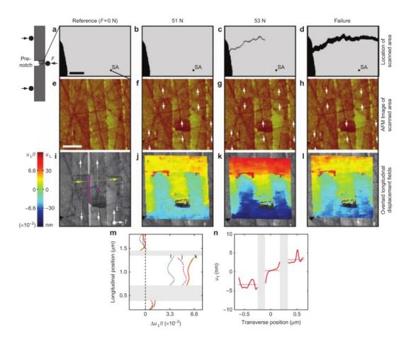
Figure 1.7: Fracture tests (3 point bending on notched samples) performed on natural nacre in AFM, combined with quantitative analysis of tablet sliding [6]
