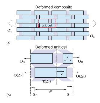
Figure 1.9: Scheme of a) the analysed composite and b) the single unit cell for the analysis [8]
