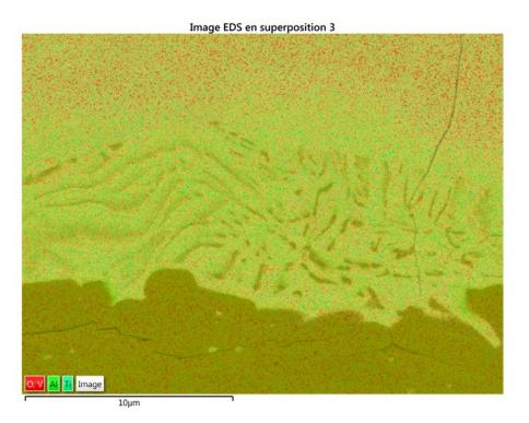
Figure 5.7: EDX image of the observed intermetallics, sample cooling speed: 100°C/min.
