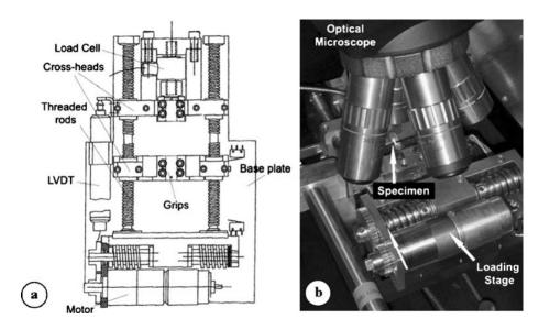
Figure 1.5: Experimental set-up for tensile test under an optical microscope [5]
