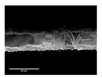
Figure 5.11: A sample sintered at 1500 °C with 30 minutes holding time at 1300 °C; minor diffusion of titanium (BSE detector)
