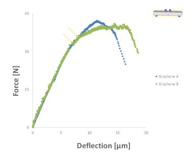
Figure 4.19: Force-Deflection curve of the material with graphene in the interphase
