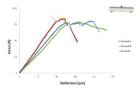
Figure 3.8: Force-Deflection curve of the material processed by uniaxial pressing
