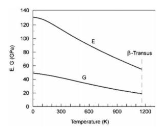
Figure 1.19: Change of value of elastic and sheer modulus in function of temperature of  $\alpha$ Ti [15]
