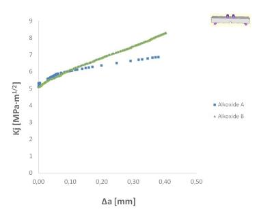
Figure 4.13: R-curves of the material with platelets processed by alkoxide reaction
