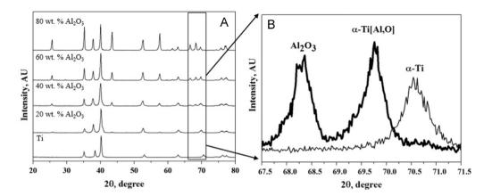
Figure 1.25: Comparison of XRD patterns for titanium and alumina/titanium composites [17]
