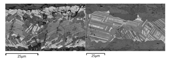
Figure 5.5: Band Contrast image of the titanium foil (camera EBSD). Both samples sintered at 1500°C. Sample on the left: cooling 100°C/min, initial foil thickness 50 $\mu$ m, sample on the right: cooling 10°C/min, initial foil thickness 100  $\mu$ m. Magnification on both images is not the same.
