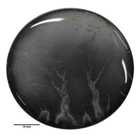
Figure 3.13: Sample obtained by uniaxial pressing and FAST with modified sintering cycle
