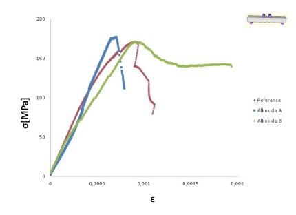
Figure 4.15: A comparison of stress-strain curves of the material with platelets processed by alkoxide reaction with standard nacre-like alumina
