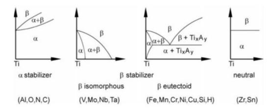
Figure 1.20: Schematic phase diagrams of titanium alloys depending on alloying elements [14]
