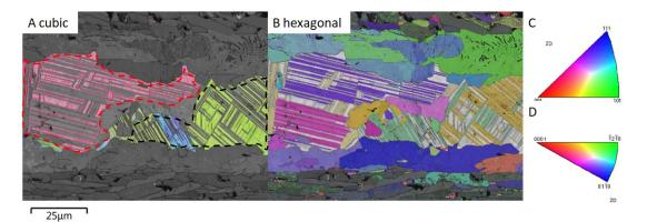
Figure 5.66: IPFZ maps for the titanium foil. A) IPFZ for cubic phase, B) IPFZ for hexagonal phase, C and D) color codes for grain orientations for cubic and hexagonal phase, respectively. Images obtained from EBSD analysis and software Channel 5.
