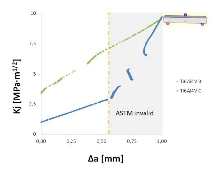
Figure 5.59: R-curves of the material with Ti6Al4V foil (around 500 $\mu$ m thick)
