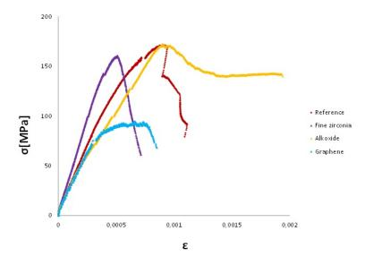
Figure 4.24: A comparison of stress-strain curves of all the material formulations tested in this study
