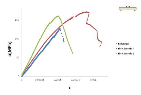
Figure 4.7: A comparison of stress-strain curves of the material with fine zirconia powder instead of TM-DAR with standard nacre-like alumina
