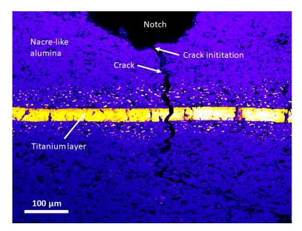
Figure 2.8: An example of crack observation by confocal microscopy
