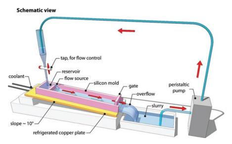
Figure 2.2: A schematic view of freezing under flow set up [19]
