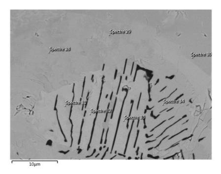
Figure 5.31: Difference between metal in inclusions zone and metal deeper in the foil
