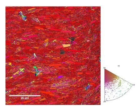
Figure 3.7: Platelets orientation and grain boundaries of sample processed by uniaxial pressing instead of freeze casting
