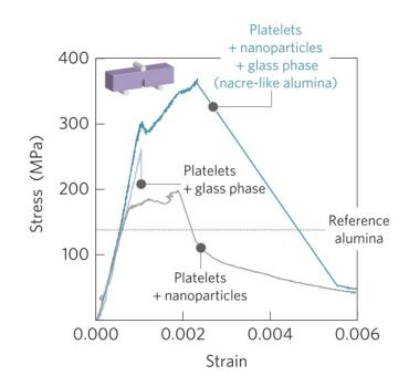
Figure 4.1: Stress-Strain curves of materials with three variants of the interphase (notched samples) [9]
