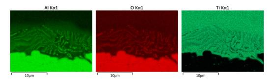
Figure 5.8: EDX images of particular elements present in the intermetallics
