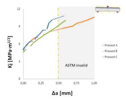
Figure 5.43: R-curves of the reference material
