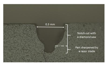
Figure 2.6: A notch prepared according to the protocol
