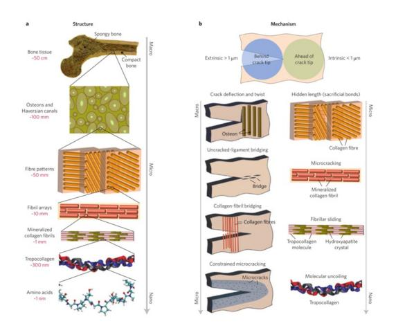
Figure 1.1: Structure and toughening mechanisms on multiple structural levels (from nanoto macro-scale) which improve mechanical properties of natural material: bone [1]
