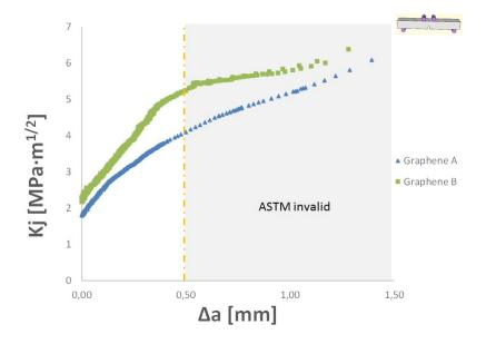
Figure 4.21: R-curves of the material with graphene in the interphase
