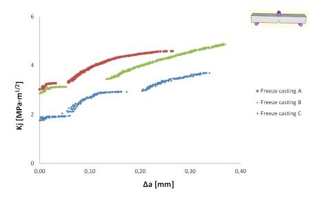
Figure 3.6: R-curves of the material processed by freeze casting
