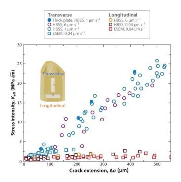
Figure 1.2: Crack-resistant curves (R-curves) of human bone tested in two directions: transverse and longitudinal [2]
