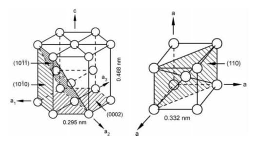
Figure 1.18: Unit cells of  $\alpha$  (hcp) and  $\beta$  (bcc) phase of titanium [14]
