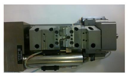
Figure 2.13: A set up allowing to perform 3PB in SEM
