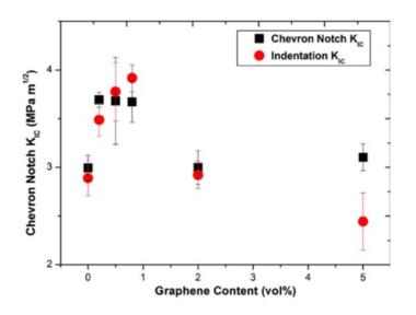
Figure 4.16: Values of fracture toughness measured by indentation and chevron notch as a function of graphene content in dense alumina composites [21]
