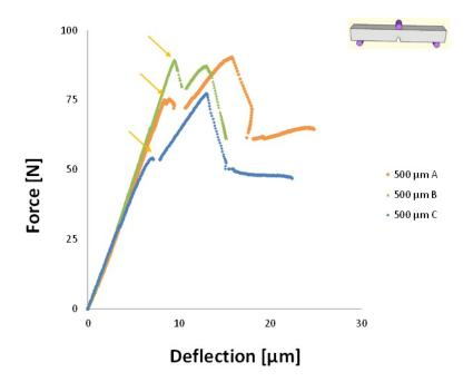
Figure 5.53: Force-Deflection curves of the material with 500 $\mu$ m foil
