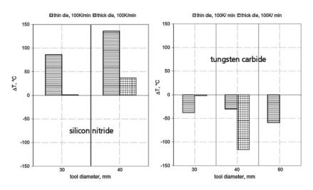
Figure 5.17: Temperature differences between internal and external zone of the material [24]. Sintering dies differed in diameter and thickness. Horizontal lines: thin die, grid: thick die.
