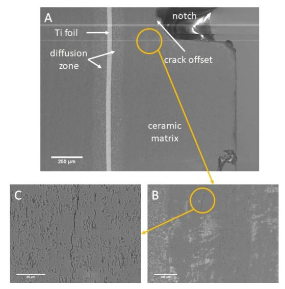
Figure 5.45: SEM pictures of the sample with a layer of titanium foil (without glassy phase) in the moment of crack offset (at 70 N) during three point bending *in situ*
