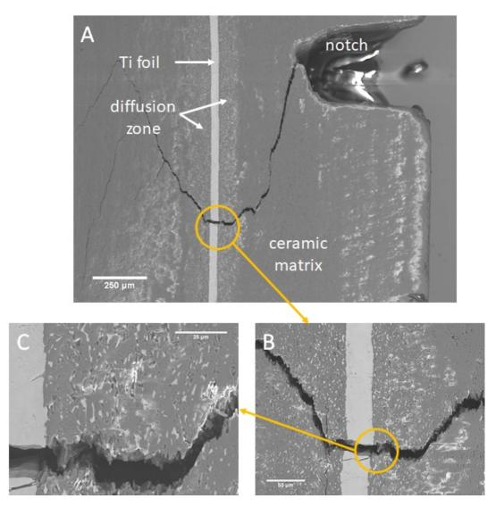
Figure 5.46: SEM pictures of the broken (at 73 N) sample with a layer of titanium foil (without glassy phase) during three point bending *in situ*
