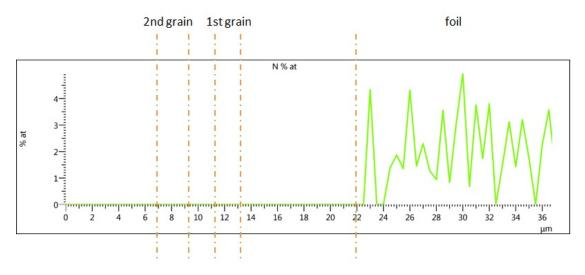
Figure 5.38: Linear analysis of nitrogen along the line shown in fig. 5.35
