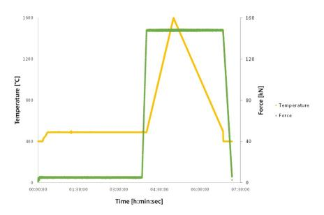
Figure 3.12: Optimized sintering cycle for up-scaling material fabrication
