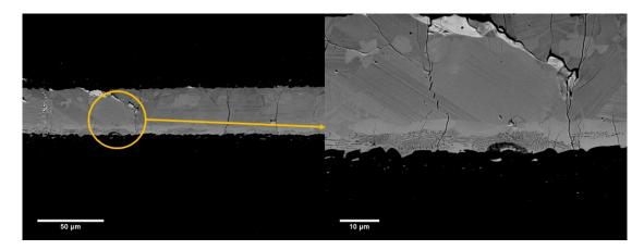
Figure 5.10: A sample sintered at 1500 °C with 30 minutes holding time at 1200 °C; minor diffusion of titanium (BSE detector)
