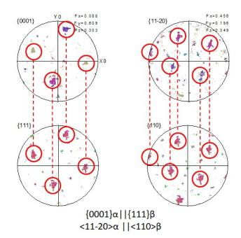
Figure 5.67: Orientation relationships between cubic and hexagonal phase found in the first domain (contoured in a red dashed line in the picture 5.66B)
