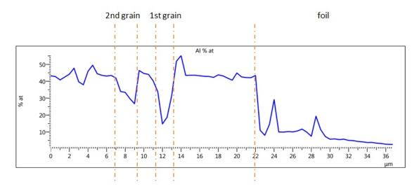
Figure 5.39: Linear analysis of aluminium along the line shown in fig. 5.35
