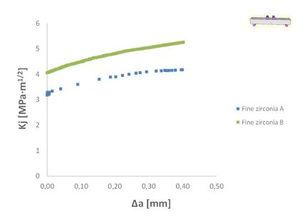
Figure 4.5: R-curves of the material with zirconia powder instead of TM-DAR
