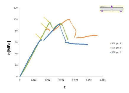
Figure 5.54: Stress-Strain curves of the material with 500 $\mu$ m foil
