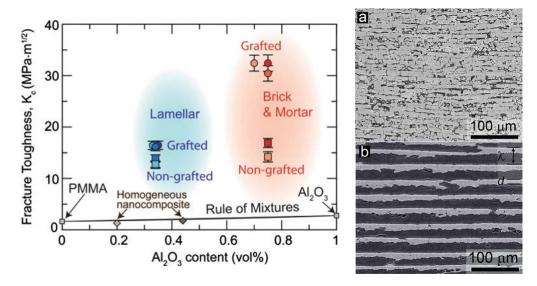
Figure 1.8: On the left: comparison of fracture toughness in alumina composites with two types of microstructure: lamellar and "brick and mortar" [7]. On the right: SEM picture of "brick and mortar" structure (a) and lamellar structure (b).
