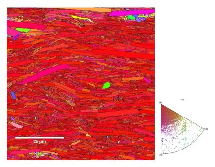
Figure 3.3: Platelets orientation and grain boundaries of sample processed by freeze casting and pressing (cross section perpendicular to sample surface)
