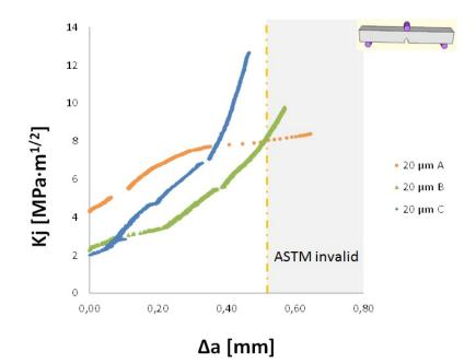
Figure 5.49: R-curves of the material with  $20\mu$ m foil. For samples B and C an ASTM invalid zone begins earlier, before 0.4 mm crack extension.
