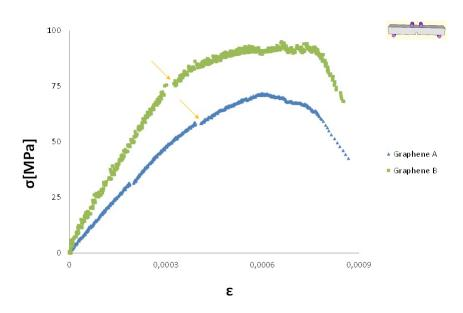
Figure 4.20: Stress-Strain curve of the material with graphene in the interphase
