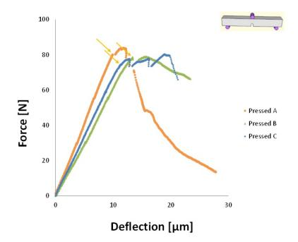
Figure 5.41: Force-Deflection curves of the reference material (no metal foil)
