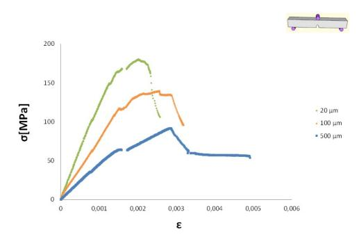
Figure 5.56: Comparison of Stress-Strain curves of materials with different foil thickness
