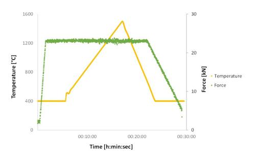
Figure 3.2: Sintering cycle for samples prepared by freeze-casting
