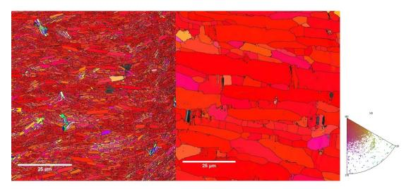
Figure 3.14: Comparison of platelets orientation and grain size of sample processed by uniaxial pressing and up-scaled one
