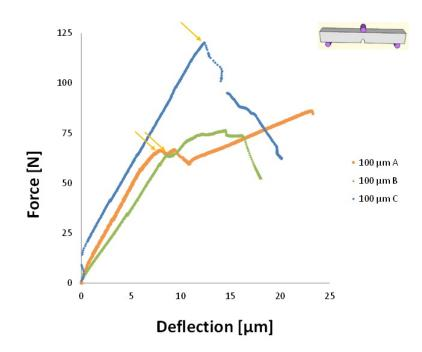
Figure 5.50: Force-Deflection curves of the material with  $100\mu$ m foil
