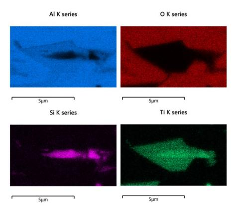
Figure 5.24: Varied chemical composition of a single grain
