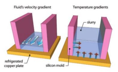
Figure 2.3: A schematic view of gradients created during freezing under flow [19]
