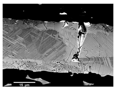
Figure 5.4: SEM image of titanium foil sintered between alumina pellets (BSE detector)
