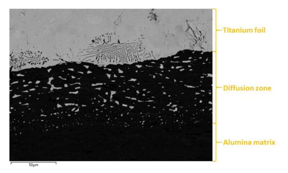
Figure 5.30: SEM picture of metal foil and diffusion zone in the composite  $Al_2O_3/TiN/Ti$ . Sintering temperature: 1500°C, heating rate: 100°C, cooling rate: 10°C.
