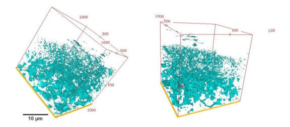
Figure 5.15: 3D volume recontruction of the sample sintered during 30 min at 1500°C. Ceramic phase was removed from the reconstruction to show titanium which infiltrated porosity.
