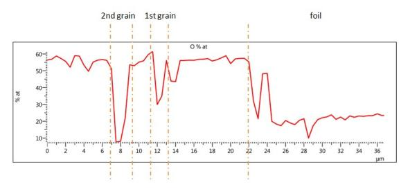
Figure 5.40: Linear analysis of oxygen along the line shown in fig. 5.35
