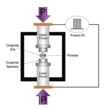
Figure 1.15: Schematic of a pulsed electric current sintering apparatus. [12]
