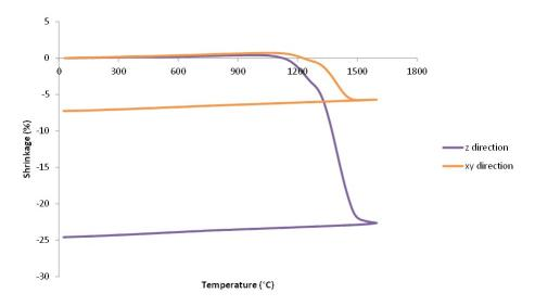
Figure 4.2: Linear thermal expansion of a composite composed of 25% alumina platelets and 75% TM-DAR (alumina nano-powder) as a function of direction: in plane (xy) or out of plane (z)
