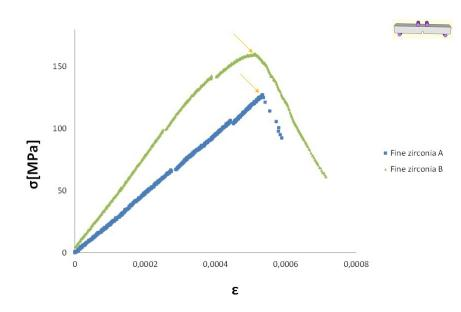
Figure 4.4: Stress-Strain curve of the material with fine zirconia powder instead of TM-DAR
