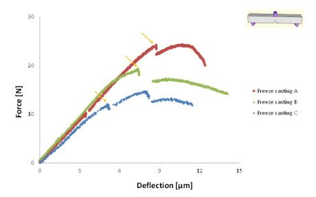
Figure 3.4: Force-Deflection curve of the material processed by freeze casting
