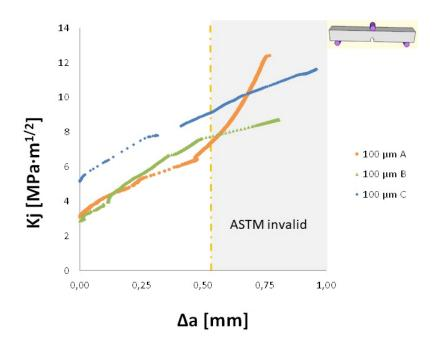
Figure 5.52: R-curves of the material with  $100\mu$ m foil
