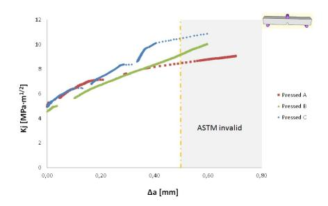
Figure 3.10: R-curves of the material processed by uniaxial pressing. ASTM invalid area concerns crack extension surpassing 0.25 of ligament length.
