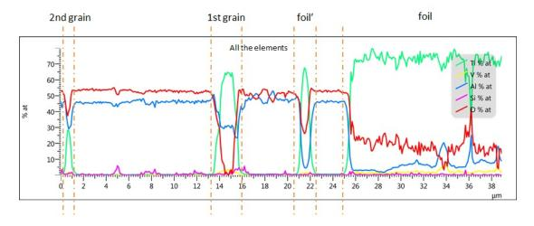
Figure 5.26: Linear analysis of all elements present in the composite starting from alumina to titanium layer, through the diffusion zone
