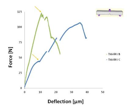
Figure 5.57: Force-Deflection curves of the material with Ti6Al4V foil (around 500 $\mu$ m thick)
