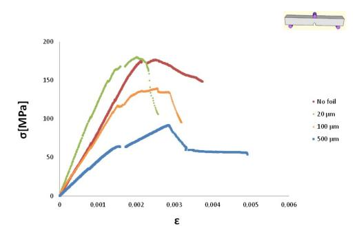
Figure 5.68: Comparison of Stress-Strain curves of materials with different foil thickness with reference material
