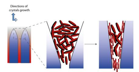
Figure 1.14: Scheme of mechanism of platelets alignment by advancing ice crystals [11]
