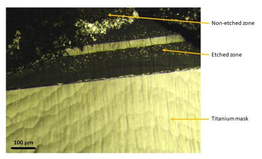
Figure 2.7: Titanium/alumina sample polished by Ilion II+. Inside the etched zone we can see titanium foil and diffusion zone (light colour) and alumina matrix (dark colour).
