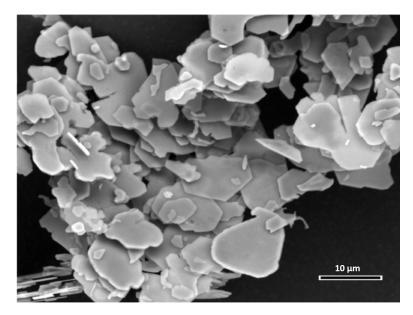
Figure 2.1: Alumina platelets used in this study [11]
