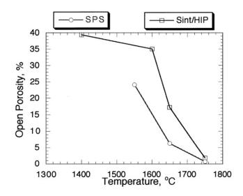
Figure 1.16: Comparison of percentage of open porosity in ceramics sintered by FAST and sintered naturally with HIP step at different temperatures [13]
