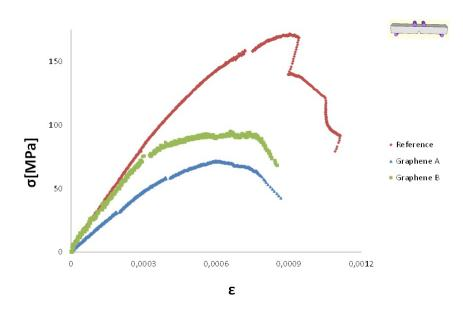
Figure 4.23: A comparison of stress-strain curves of the material with graphene in the interphase with standard nacre-like alumina
