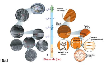
Figure 1.4: The structure of nacre: aligned aragonite tablets (diameter approximately 8  $\mu$ m and thickness 0.4  $\mu$ m) and thin organic interphase [4]
