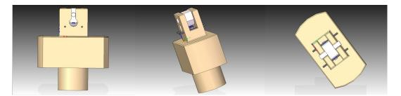
Figure 2.12: Four-point bending montage assembled
