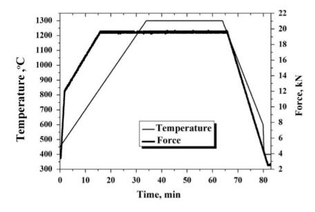
Figure 1.24: Sintering cycle for alumina/titanium composite processing [17]
