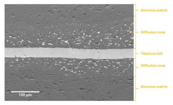
Figure 5.1: SEM image of alumina/titanium composite (sintered at 1500°C) showing three regions (initial titanium foil thickness of  $50\nu$ m, final  $30-40\mu$ m). Some platelets pull out has occurred during polishing in the alumina matrix.
