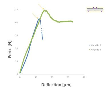
Figure 4.11: Force-Deflection curve of the material with platelets processed by alkoxide reaction
