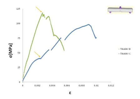
Figure 5.58: Stress-Strain curves of the material with Ti6Al4V foil (around 500 $\mu$ m thick)
