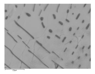
Figure 5.18: Intermetallic structures inside Ti6Al4V foil. Bright grey: metal,dark grey: inclusions.
