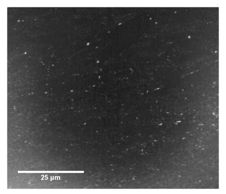
Figure 5.14: One picture from volume reconstruction of the sample 30 min at 1200°C. It shows residual porosity (light) in ceramic matrix (darker). It is the zone close to the titanium film (scan perpendicular to the metal layer) but no visible diffusion was noticed.
