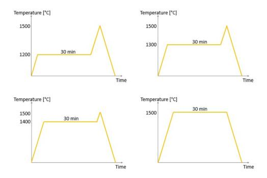
Figure 5.9: Temperature profiles of applied sintering cycles. Holding time of 30 minutes at 1200, 1300, 1400 and 1500°C respectively, max. temp. 1500°C for all treatements.
