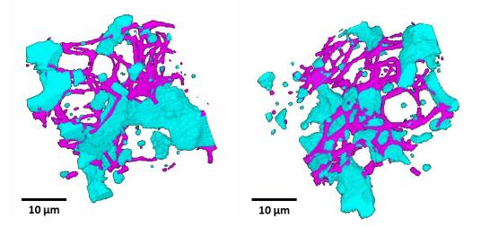
Figure 5.16: Close-up look on grain interconnections and residual porosity which was not infiltrated by metal. Sample sintered during 30 min at 1500°C. Ceramic phase was removed from the reconstruction to show titanium and porosity. Titanium phase is in cyan and porosity in magenta.
