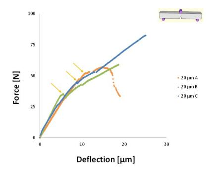
Figure 5.47: Force-Deflection curves of the material with  $20\mu$ m foil. Sintered at 1500°C, heating rate: 100°/min, cooling rate: 10°/min.
