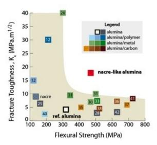
Figure 1.10: Improved mechanical properties of biomimetic nacre-like alumina in comparison to conventional composites of alumina [9]
