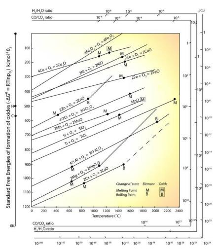
Figure 5.64: Ellingham-Richardson diagram of common oxides (free energy in function of temperature). It shows that thermodynamically alumina is more stable than titanium oxide  $(TiO_2)$  in our temperature range.
