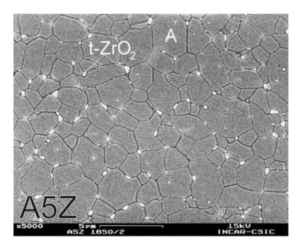
Figure 4.9: SEM image of alumina/zirconia composite fabricated thanks to alkoxide processing [20]
