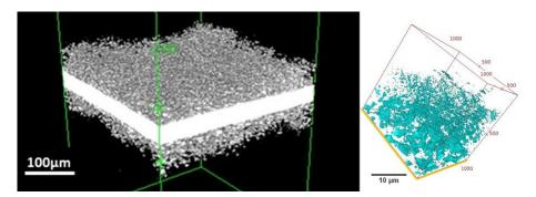
Figure 2.9: Comparison of 3D reconstructions of scans performed in EasyTomo Nano tomograph in MATEIS laboratory (on the left) and in ESRF synchrotron facility (on the right). Samples were composed of layers of alumina and titanium with significant diffusion of metal into ceramic matrix. Resolution on the left: 700 nm, on the right: 50 nm. In the right picture titanium foil is not visible because of the noise in the scan, yellow lines indicate where titanium was placed.
