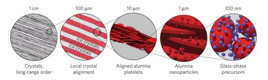
Figure 1.11: Microstructural composition of nacre-like alumina [9]
