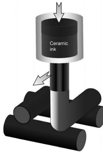
Figure III-10 : Schematic of robocasting technique (Saiz et al. [162])
