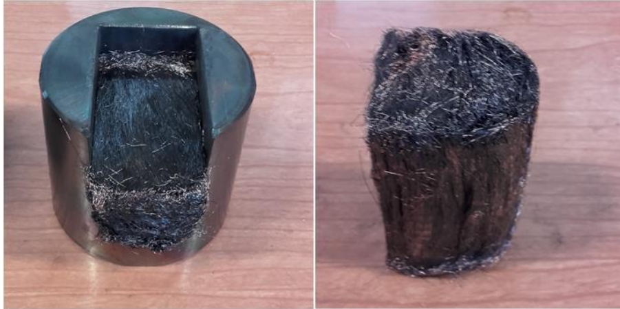
Figure III-12: Pictures of the porous structure after PECS
